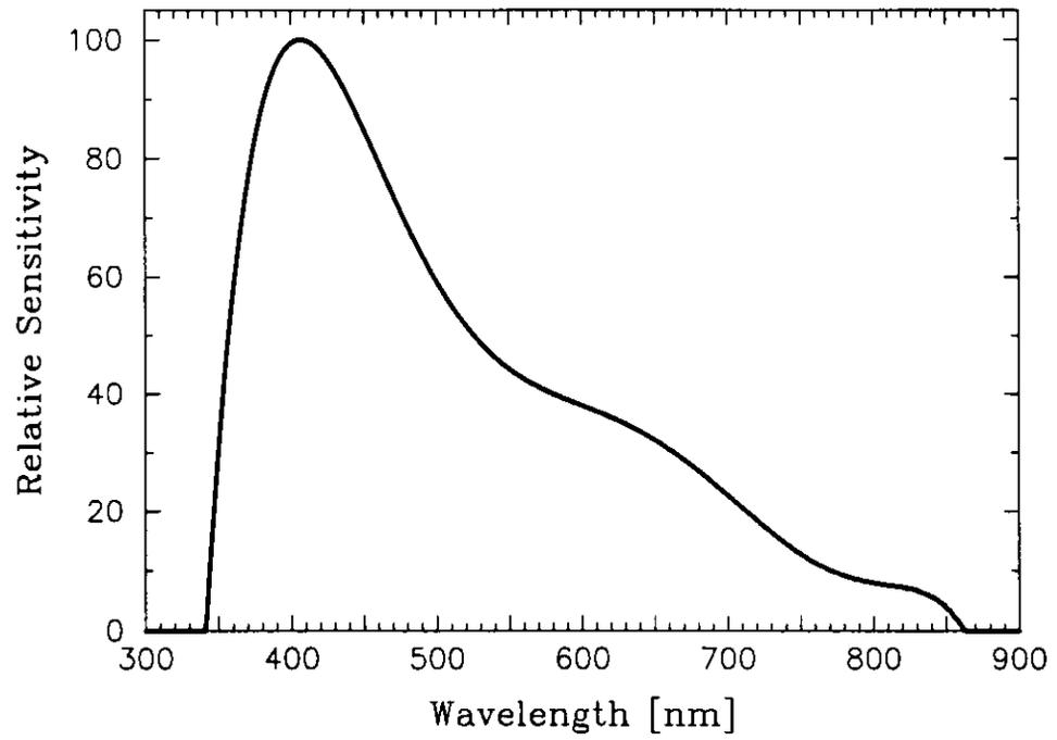
FIGURE 2.5. Spectral sensitivity curve of the intensified HDTV camera operated on FISTA. This system is sensitive in 360 - 850 nm range, with the maximum sensitivity at 405 nm.
