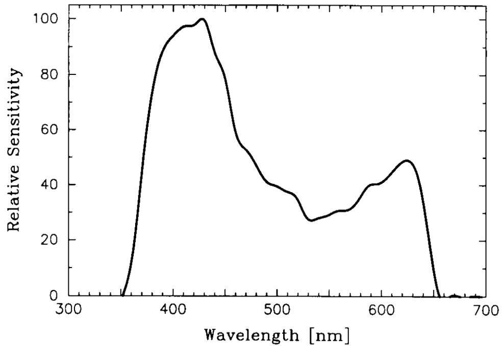
FIGURE 8.1. Relative spectral sensitivity of the observational system. The system is sensitive in the 370 - 640 nm range. The sensitivity curve is normalized to 100.0 at the peak wavelength,  $\sim 428$  nm.
