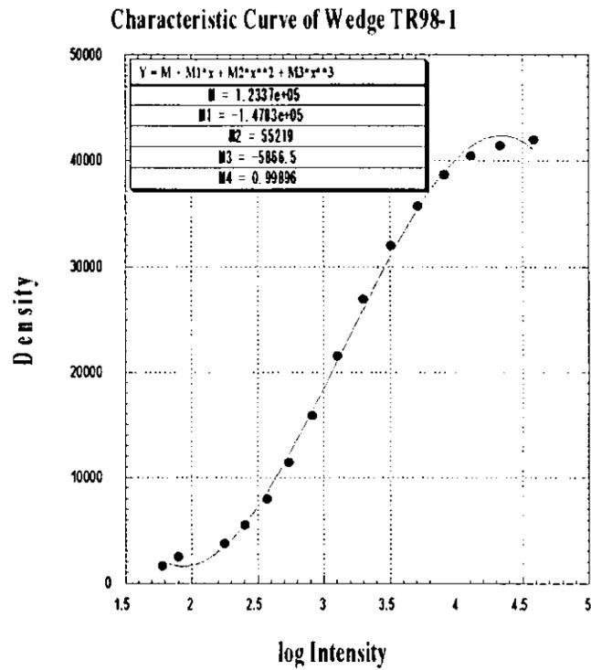
FIGURE 8.2. Characteristic curve of photographic plate obtained by photographic wedge. This curve used for reducing the reading of film density to the linear scale in magnitude for the persistent train spectrum No.1. - No.4.
