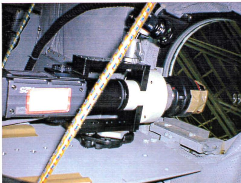
FIGURE 2.3. Intensified High-Definition TV Camera installed on FISTA.
