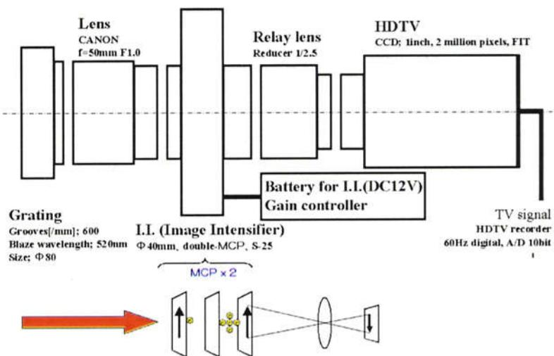
FIGURE 2.4. Schematic of Intensified High-Definition TV Camera.
