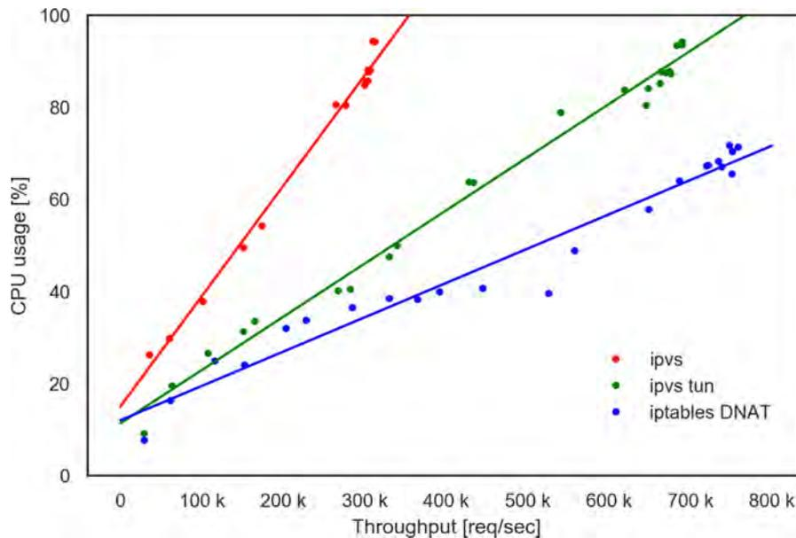
Figure 5.3: CPU usage of load balancers in containers. The iptables DNAT rules exist in the node net namespace. The IPVS and IPVS-TUN are in containers. The iptables DNAT consumes the smallest amount of the CPU resource.
