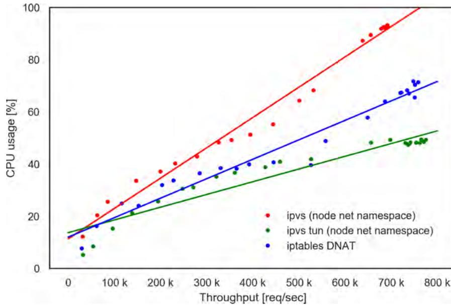
Figure 5.5: CPU usage of load balancers on nodes. CPU usages of IPVS and IPVS-TUN greatly improved from those in Figure 5.3 by placing them in node net namespace. While the IPVS-TUN consumes the smallest amount of the CPU resource, the CPU usage of IPVS is still larger than that of iptables DNAT.
