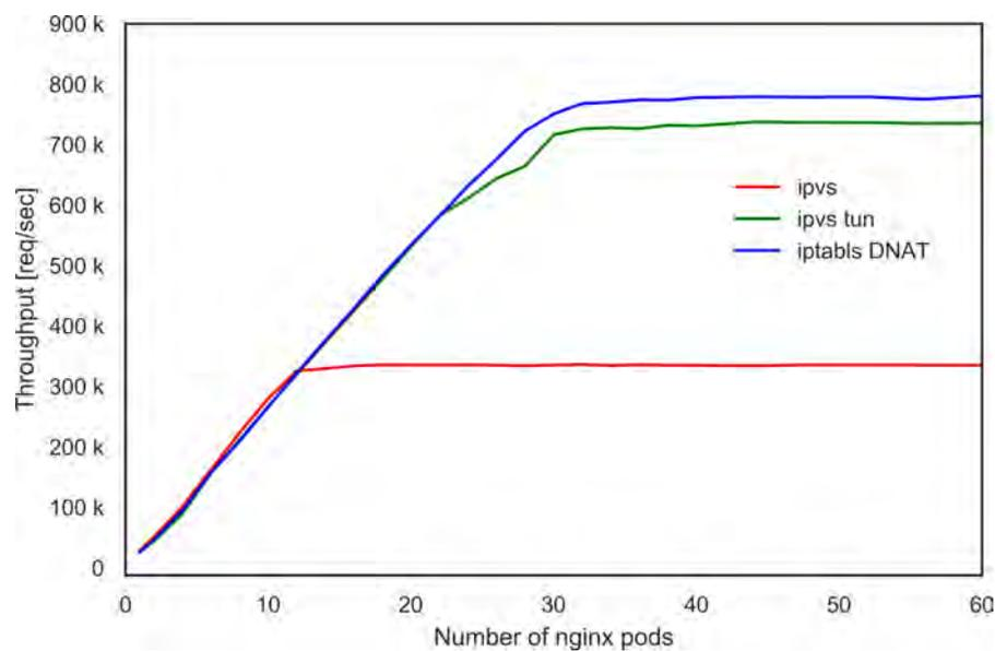
Figure 5.2: Throughput of load balancers in 10 Gbps. The iptables DNAT rules exist in the node net namespace. The IPVS and IPVS-TUN are in containers. The throughput of the iptables DNAT is the highest.
