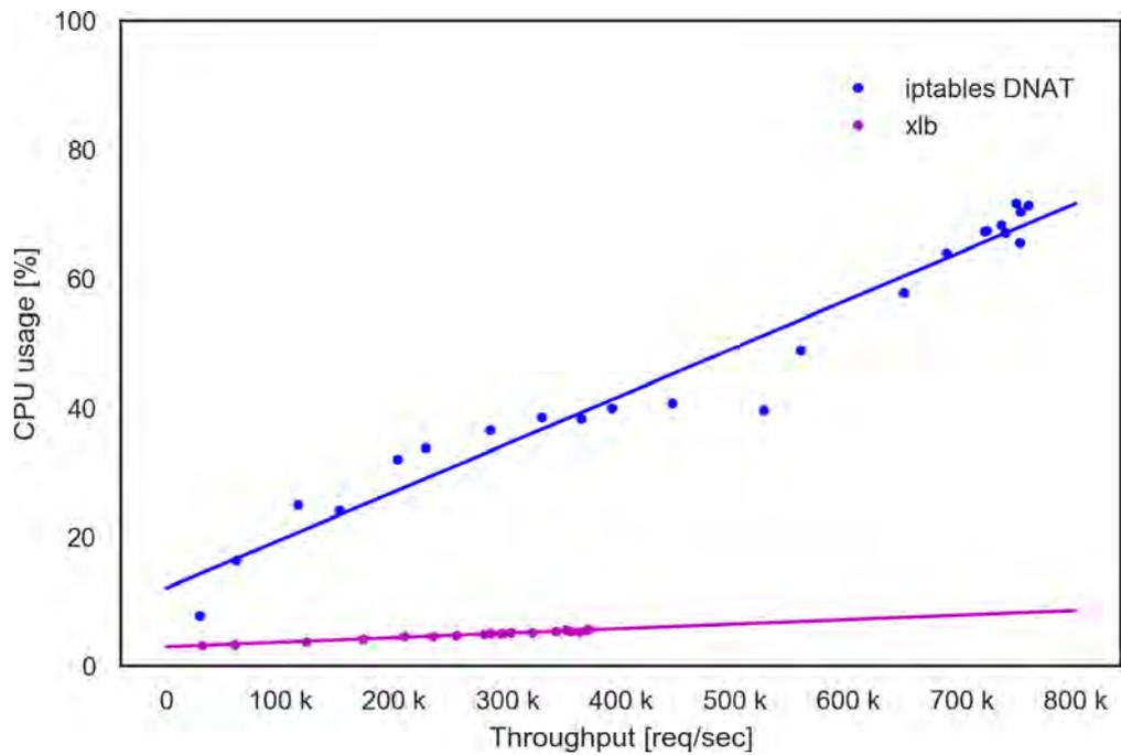
Figure 5.8: CPU usage of xlb load balancer. The xlb uses much less CPU resource than iptables DNAT.
