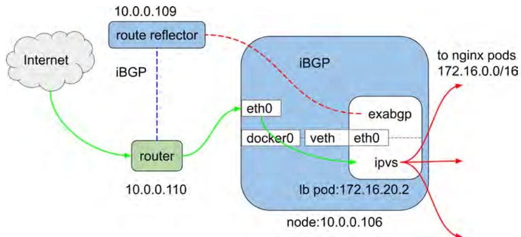
Figure 3.8: Network path by the exabgp container. The packets from Internet to service IPs, 10.1.1.0/24 are routed to the load balancer pod (green arrows) by the set of routing rules shown in Table 3.2. And then the IPVS container forwards them to nginx pods (red arrows). The IP address of any pod is dynamically assigned from 172.16.0.0/16 when the pod is started.
