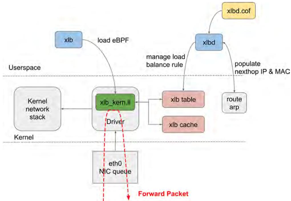
Figure 5.6: Xlb architecture. The author implemented an XDP load balancer named xlb.
