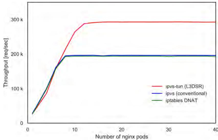
Figure 4.9: Throughput of L3DSR using IPVS-TUN. The throughput of IPVS-TUN is 1.5 times higher than those of conventional IPVS and iptables DNAT.
