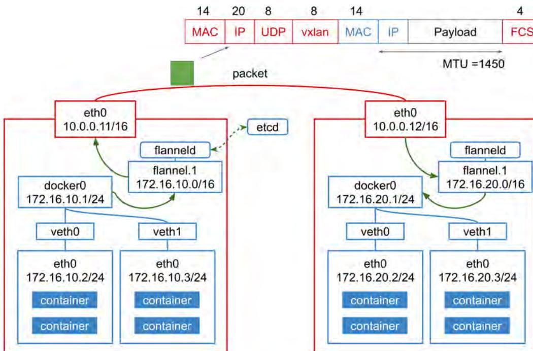
Figure 2.3: Flannel setup with vxlan. The flanneld on the nodes updates routing entries for containers. In addition to that, the flanneld also create Linux kernel's vxlan device, flannel.1 on every node. When packets are sent out through flannel.1 devices, the flannel.1 encapsulate the original packets with vxlan headers.
