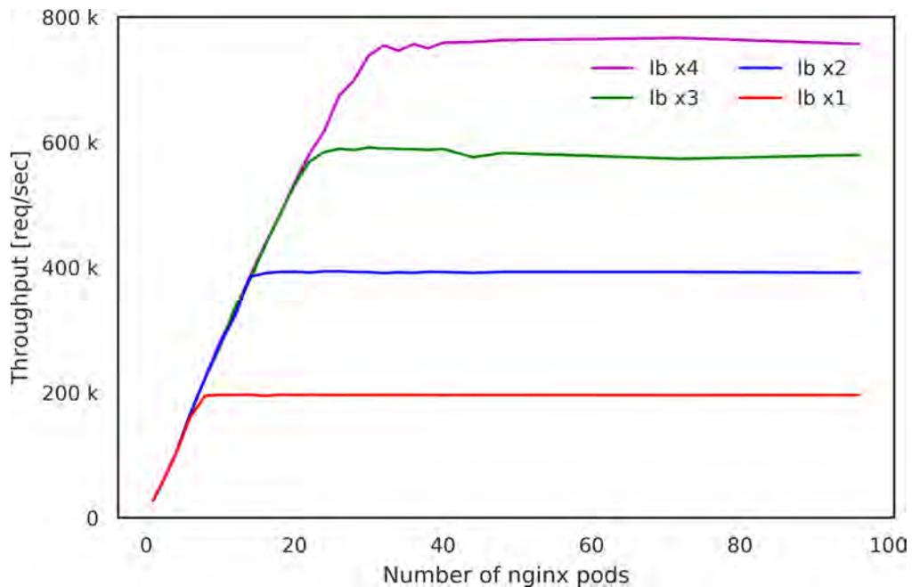
Figure 4.13: Throughput of ECMP redundant load balancer. The throughputs are measured for a single load balancer (lb x1), two (lb x2), three (lb x3) and four (lb x4) load balancers.
