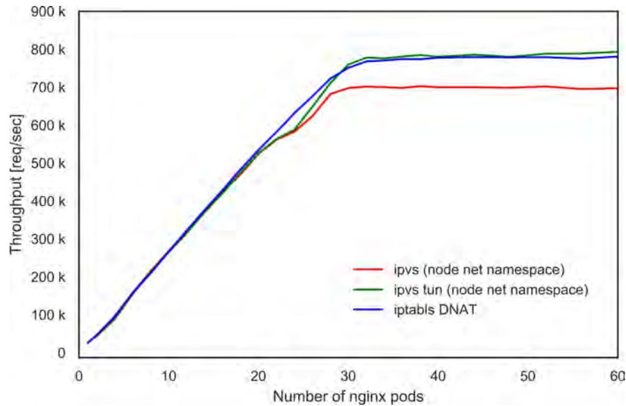
Figure 5.4: Throughput of load balancers in node namespace. The performance levels of the IPVS and IPVS-TUN are greatly improved from those in Figure 5.2 by placing them in node net namespace.
