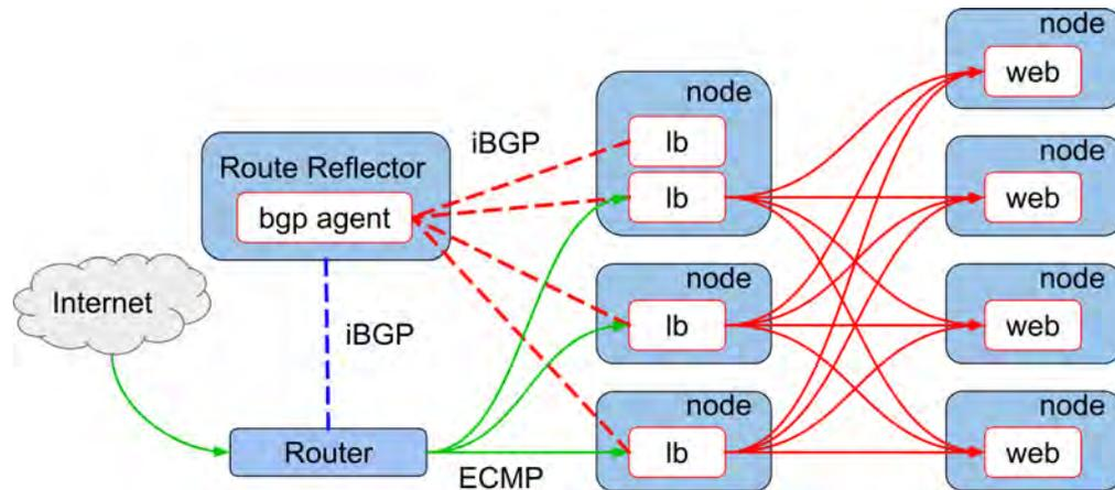
Figure 3.3: The proposed architecture of load balancer redundancy with ECMP. The traffic from the internet is distributed by the upstream router to multiple of load balancer (lb) pods using hash-based ECMP (the solid green line), after which distributed by the lb pods to web pods using Linux kernel's IPVS (the solid red line). The route toward a service IP is advertised to the route reflector (the dotted red line), after which advertised to the upstream router (the blue dotted line) using iBGP.
