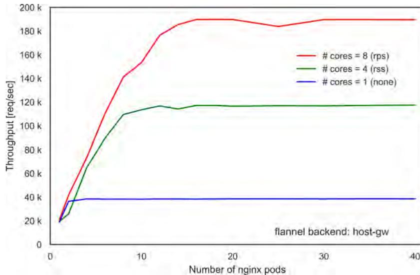
Figure 4.2: Effect of multicore packet processing on IPVS throughput. Throughput linearly increases as the number of nginx *pods* increases and then it eventually saturates. The throughput is highest for the setting with eight cores (rps = on), followed by four cores (rss = on), then single core (none).
