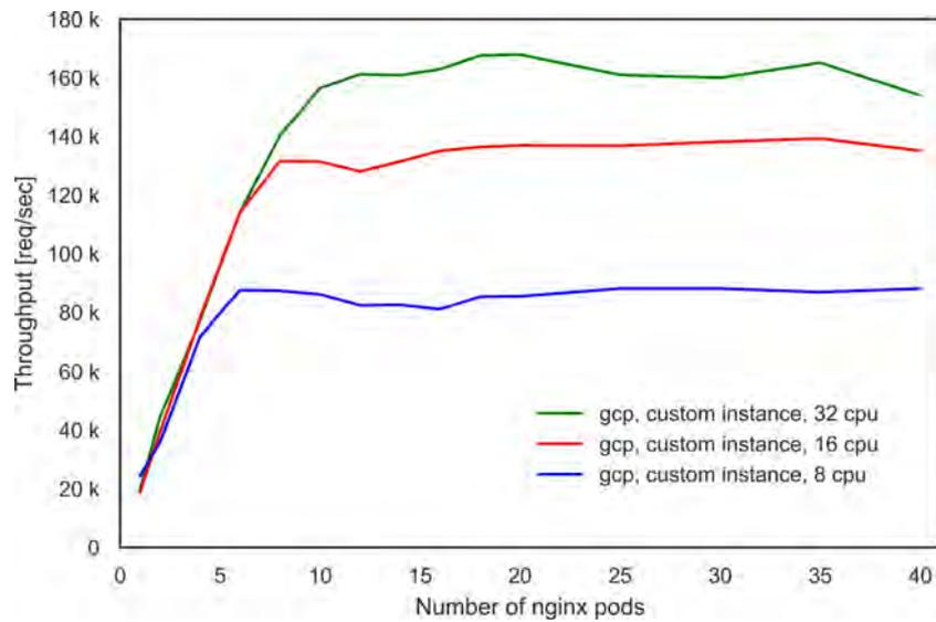
Figure 4.10: Throughput measurement results in GCP. The throughput increases linearly as the number of nginx *Pods* increases until it reaches the saturation level. The maximum throughput is higher for instances with more virtual CPUs.
