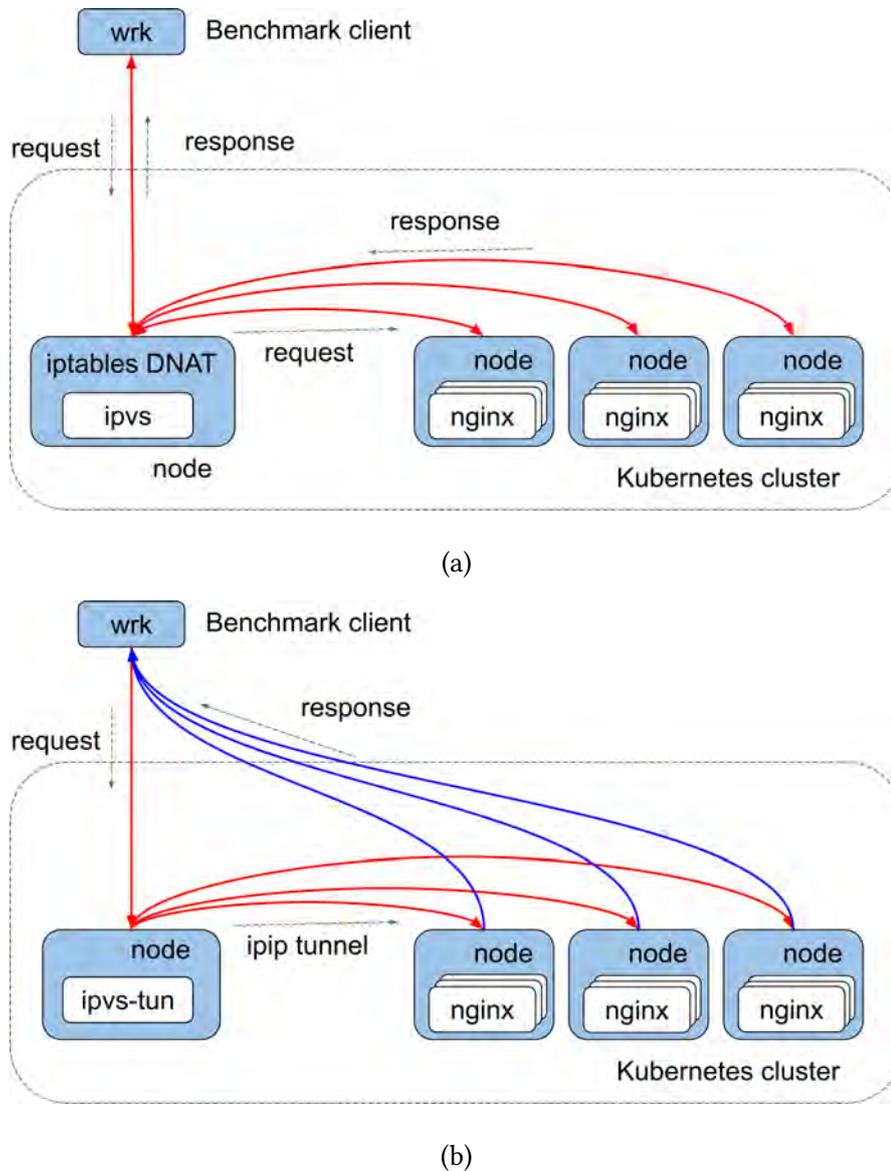
Figure 5.1: Benchmark setups in 10 Gbps experiment. (a) The setup used in throughput measurements of IPVS and iptables DNAT. The request and response packets both go through the load balancer node. (b) The setup used in throughput measurements of IPVS-TUN. The response packets for IPVS-TUN, return directly to the benchmark client.
