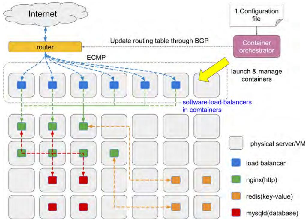
Figure 1.7: Load balancer for container clusters. In order to distribute the traffic, the container orchestrator launches a cluster of software load balancer containers. The container orchestrator also communicates with the upstream router through BGP protocol, and the router sets up an ECMP routing rule in the routing table.
