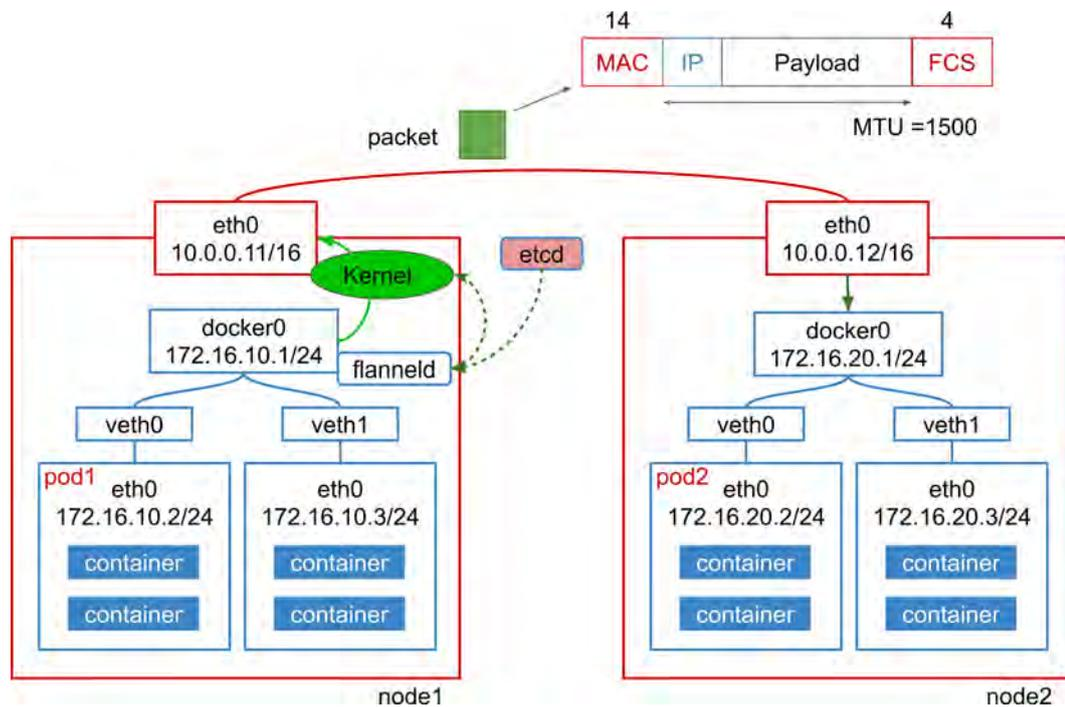
Figure 2.2: Flannel setup with host-gw mode. The *pod1* on the node1 sends out an IP packet to *pod2* on the node2. After receiving packets from the *pod1*, the node1 learns that *pod2* is on the node2, and forward the packets to the node2 without any encapsulation. The flanneld continuously updates routing entries for containers in the routing table on each node.
