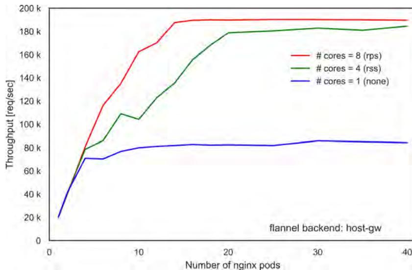
Figure 4.3: Effect of multicore packet processing iptables DNAT throughput. Throughput linearly increases as the number of nginx *pods* increases and then it eventually saturates. The throughput is highest for the setting with eight cores (rps is on), followed by four cores (rss is on), then single core (none).
