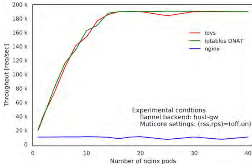
Figure 4.6: Throughput of IPVS, iptables DNAT and nginx. The performance levels of IPVS and iptables DNAT are almost the same. The nginx as a load balancer does not perform well in the experiment.
