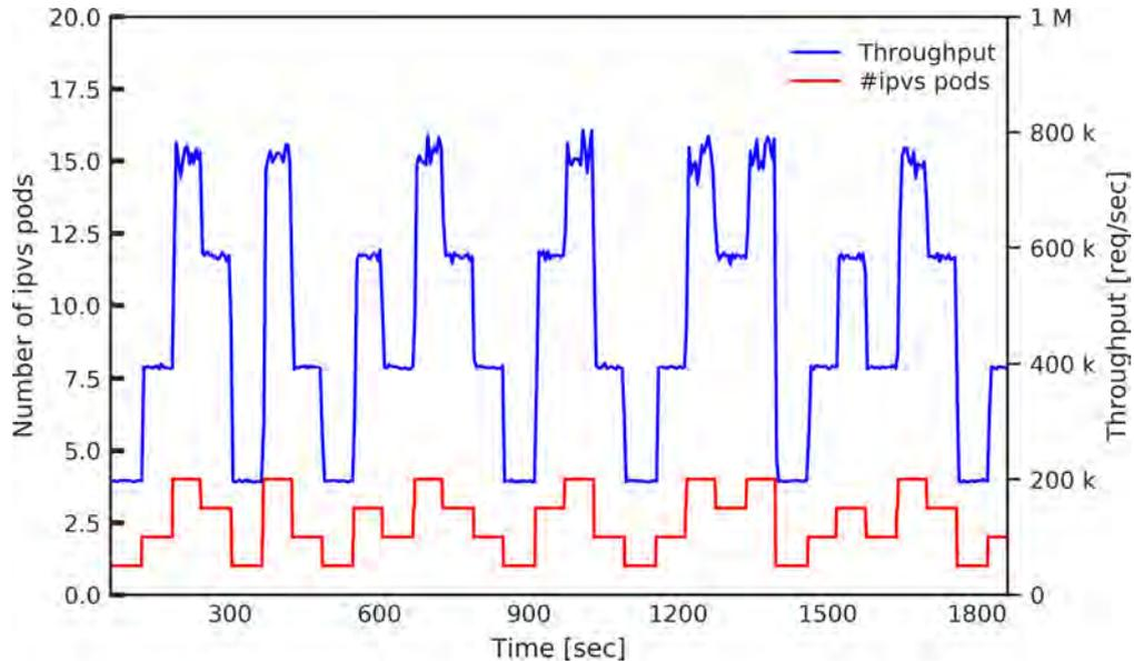
Figure 4.14: Throughput responsiveness. Throughput responsiveness when the number of load balancers is changed randomly in every 60 seconds is shown.
