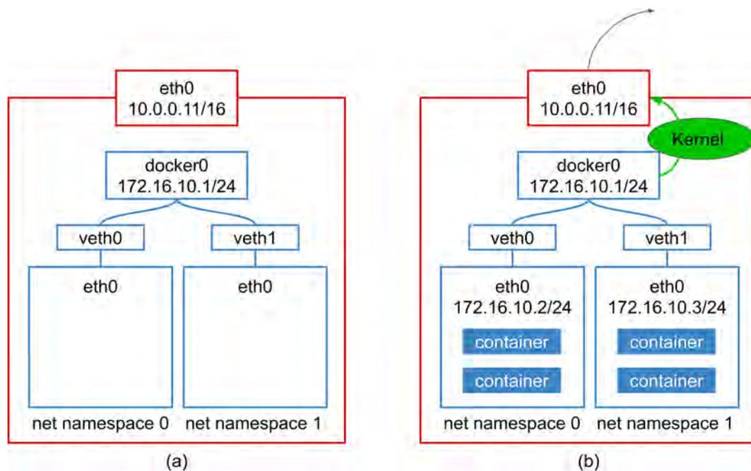
Figure 2.1: Docker networks setup. (a) Two pairs of network interfaces (`veth0,eth0`) and (`veth1,eth0`) are created. Each of the pairs acts like a pipe. The `veth0` and `veth1` are placed in the host (node) network namespace, and connected to the `docker0` bridge. The `eth0`s are placed in respective container namespaces. (b) Communication between network namespace 0 and 1 is through the `docker0`. Communication with the outside of the node follows the routing table inside the kernel.
