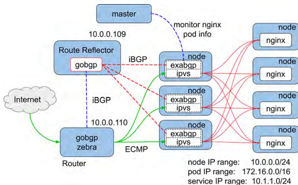
Figure 3.4: An experimental container cluster with proposed redundant software balancers. The master and nodes are configured as Kubernetes's master and nodes on top of conventional Linux systems, respectively. The route reflector and the upstream router are also conventional Linux systems. For the green lines, a service IP address is used. The red lines use the IP addresses of the overlay network. The blue line uses the IP addresses of the node network.
