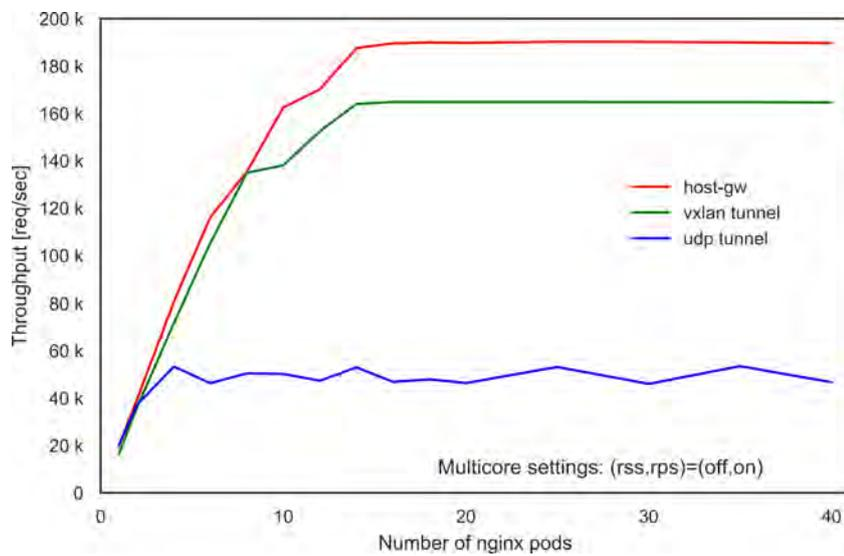
Figure 4.5: Effect of flannel backend modes on iptables DNAT throughput. the host-gw mode shows the highest performance level, followed by the vxlan mode. The udp mode shows significantly lower performances levels.
