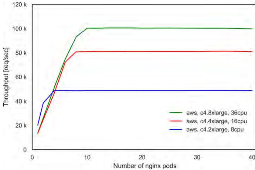
Figure 4.11: Throughput measurement results in AWS. The throughput increases linearly as the number of nginx *Pods* increases until it reaches the saturation level. The maximum throughput is higher for instances with more virtual CPUs.
