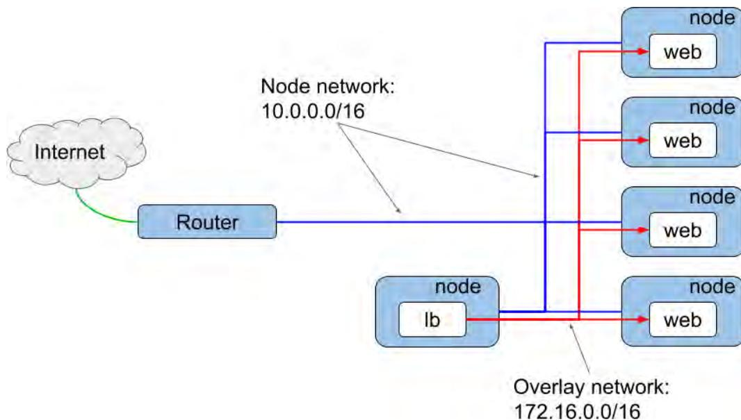
Figure 2.5: A network architecture of container cluster system. A load balancer (lb) pod (the white box with "lb") and web pods are running on nodes (the blue boxes). The traffic from the internet are forwarded to the lb pod by the upstream router using the node network, and the distributed to web pods using the overlay network.
