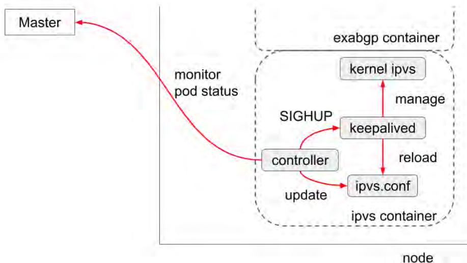
Figure 3.5: Implementation of IPVS container. The controller checks the pod status every second, by consulting the master node. Upon a change of the status, the controller updates the *ipvs.conf* and sends *SIGHUP* to *keepalived*. The *keepalived* reload the *ipvs.conf* and updates the load balancing rules in the kernel correctly.
