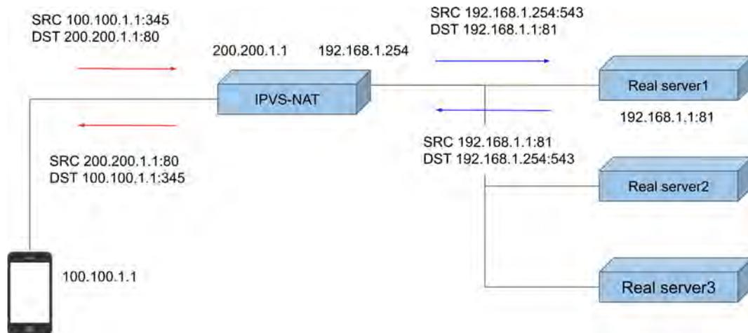
Figure 2.10: Schematic diagram of IPVS NAT mode. The IP packets arriving at the IPVS NAT enabled host are forwarded to real servers. The IP headers are translated by IPVS NAT function in the Linux kernel.
