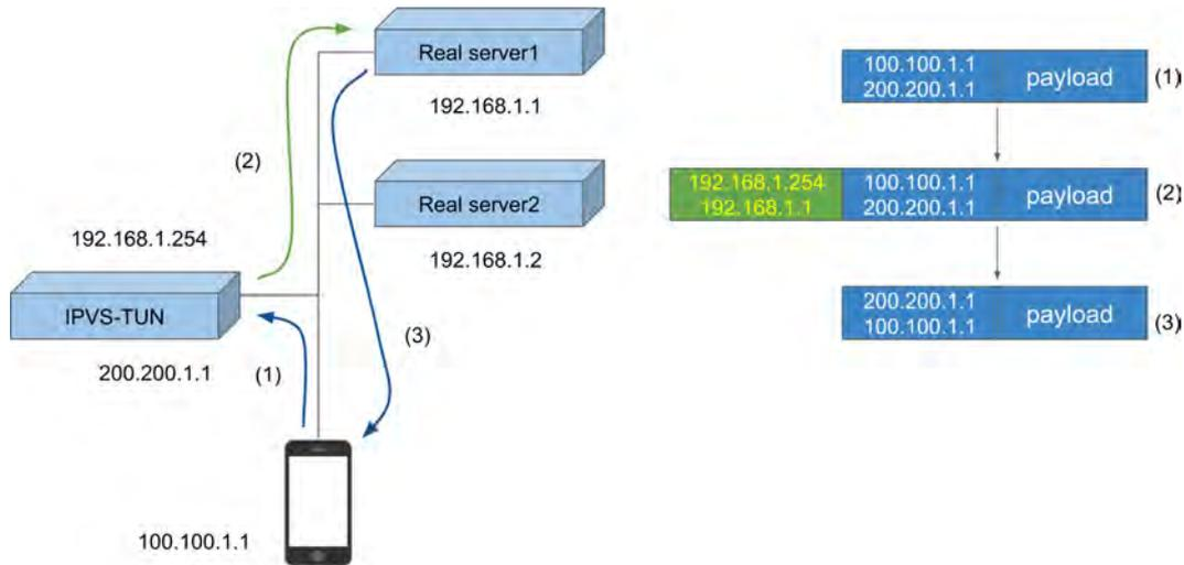
Figure 2.11: Schematic diagram of IPVS tunneling mode. (1) The packet arriving IPVS-TUN enabled host is encapsulated and (2) sent out to one of the real servers. (3) The real server returns the response packets to the client directly.
