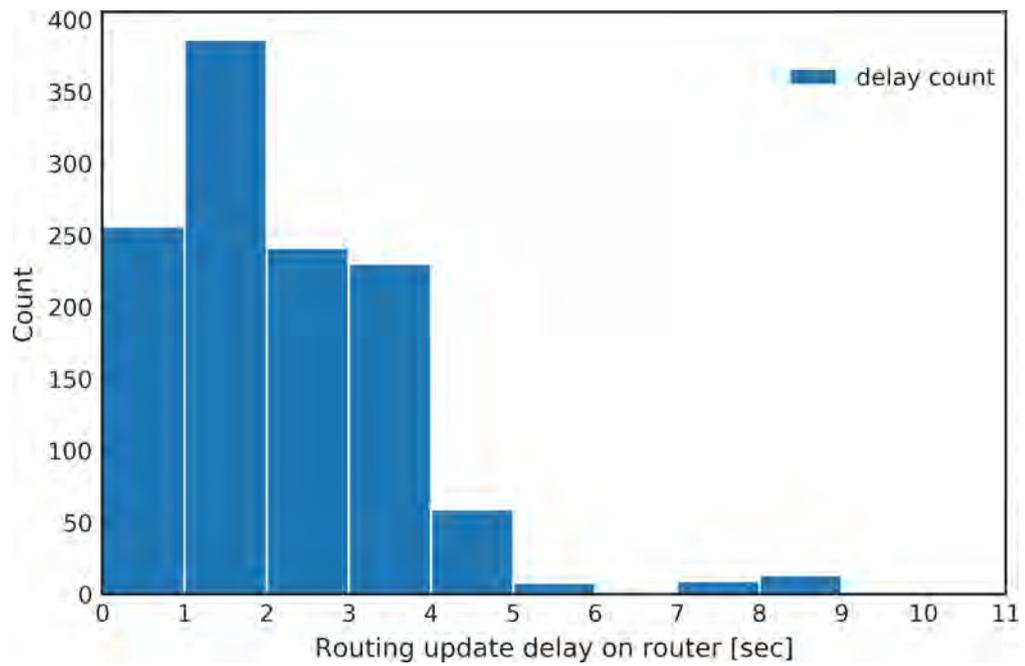
Figure 4.15: ECMP update delay histogram. This shows the delays until the number of running IPVS pods is reflected in the routing table on the benchmark client, when the number of the IPVS pods is changed randomly every 60 seconds for 20 hours.
