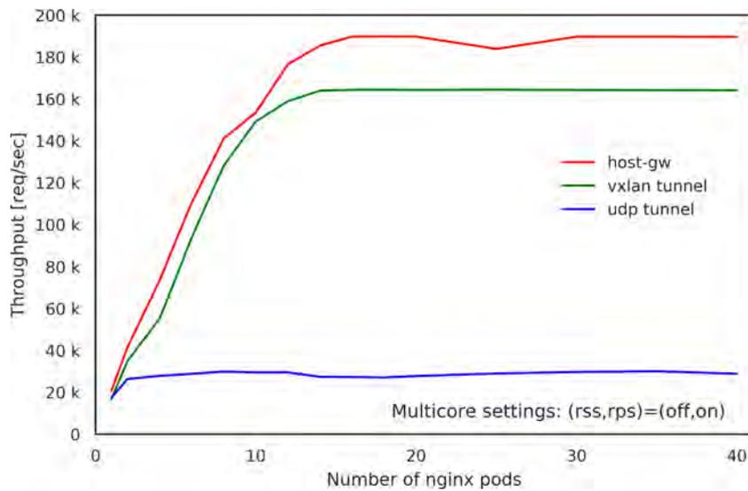
Figure 4.4: Effect of flannel backend modes on IPVS throughput. The host-gw mode shows the highest performance level, followed by the vxlan mode. The udp mode shows significantly lower performances levels.
