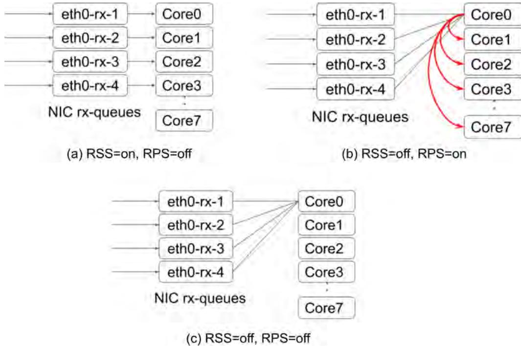
Figure 2.9: RSS/RPS settings used in this study. (a) In the case of “RSS=on,RPS=off”, only four cores are used for packet processing. (b) In the case of “RSS=off,RPS=on”, eight cores are used for packet processing. (c) In the case of “RSS=off,RPS=off”, only one core is used for packet processing.
