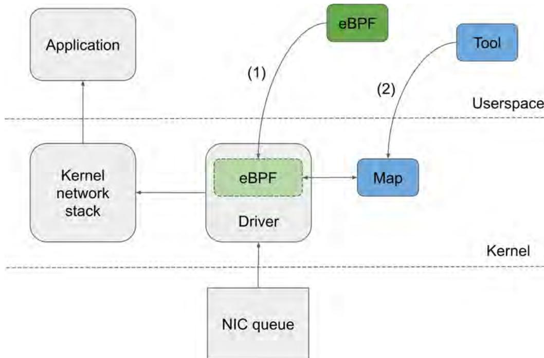
Figure 2.12: XDP architecture. In XDP, user can inject self-made byte-compiled eBPF code in the NIC driver and let it process the incoming packets much earlier than the kernel's network stack. The eBPF programs can make a map inside the kernel, and read/store temporal data from that map. The map is mount at `"/sys/fs/bpf/"`. User can manipulate the behaviour of the eBPF through this map.
