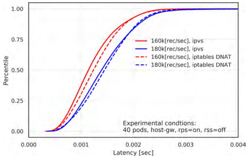
Figure 4.7: Latency for IPVS and iptables DNAT. Cumulative Distribution Function (CDF) of the latency for IPVS and iptables DNAT are compared, at the two constant loads, 160K[req/sec] and 180K[req/sec]. Smaller latencies are observed for IPVS.
