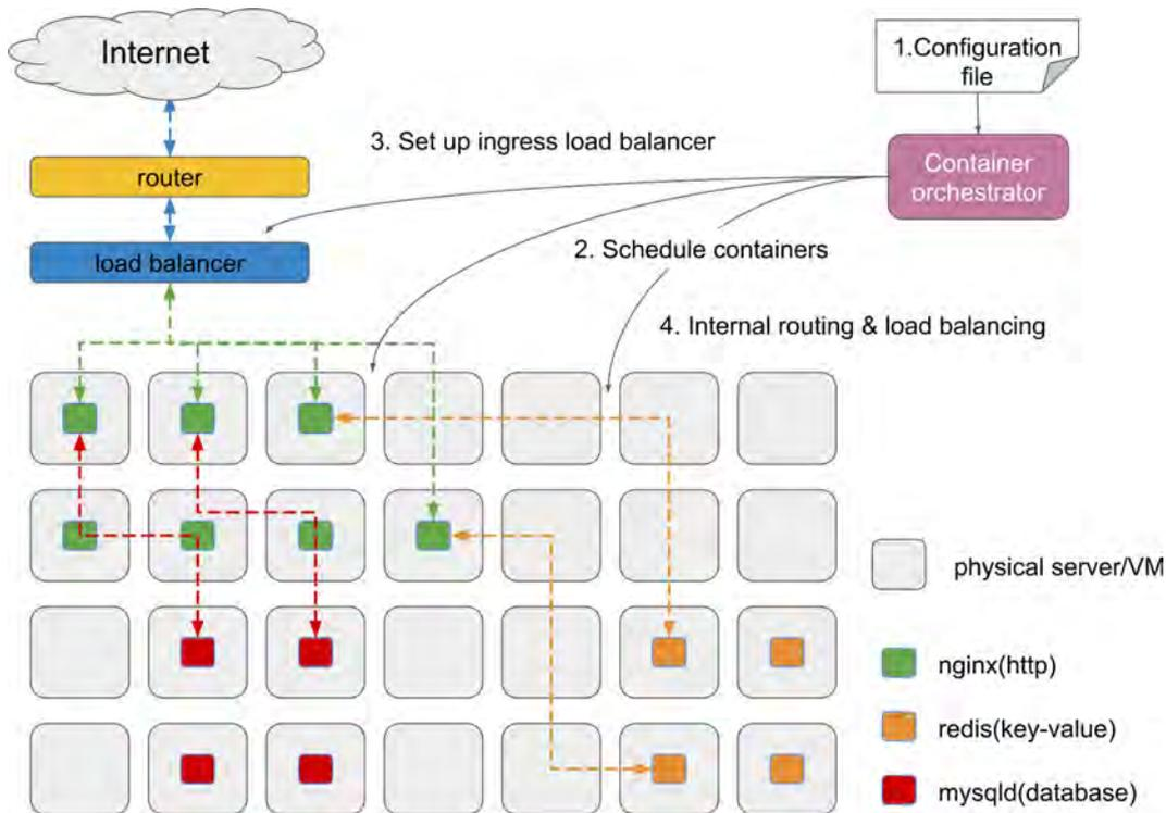
Figure 1.5: A web application cluster and container orchestrator. A web application cluster consists of nginx (http), redis (key-value store) and mysql (database) is depicted in this figure. Each of the component consists of a container cluster. Container orchestrator receive configuration file(1), schedule containers(2), set up ingress routing using load balancer(3) and set up internal routing(4).
