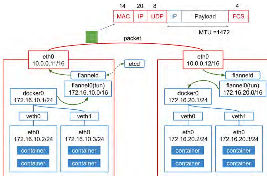
Figure 2.4: Flannel setup with udp. The flanneld creates the tun device, flannel0, and updates routing entries for containers. The flannel0 device is connected to the flanneld daemon itself. When packets are sent out through flannel0 devices, the flanneld daemon encapsulates the original packets with udp headers.
