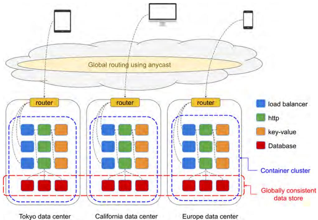
Figure 1.3: An ideal global container infrastructure. Multiple web application clusters, each of which consisting of a cluster of containers, are deployed in three different data centers as an example. In each of the data center, container orchestrator manages the container cluster. Important data are stored in a globally consistent data store. Access from the client is routed to the closest data center using anycast.
