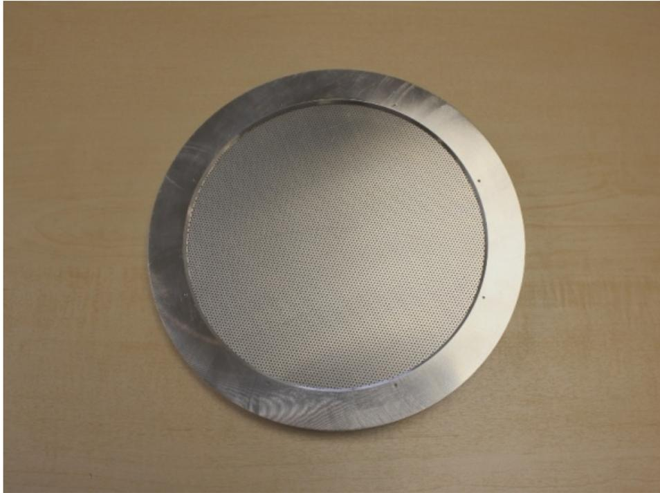
Figure 78 The neutralization grid for the beam area of  $300 \text{ cm}^2$
