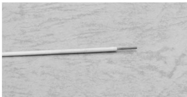
Figure 42 The picture of Langmuir probe
