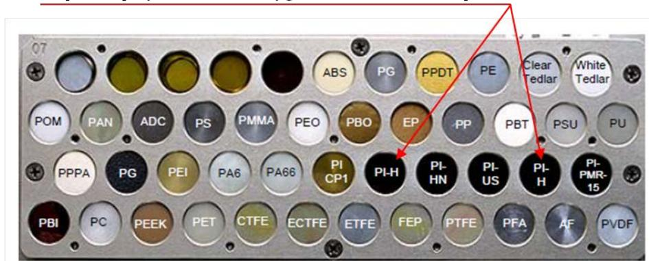
**Figure 46** Photograph of the MISSE2 PEACE Polymers experiment including two Kapton-H polyimide atomic oxygen fluence witness samples.
