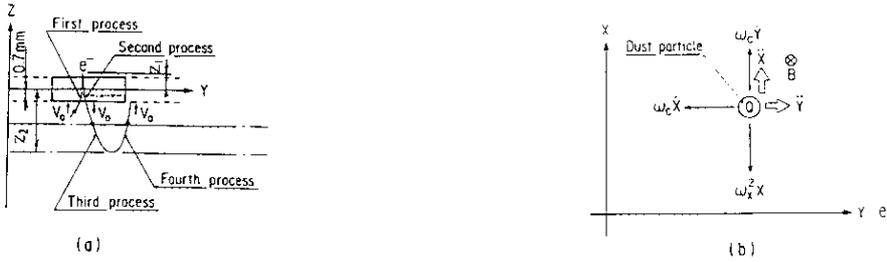
For example, setting  $QE_z/m$  to be  $1.85 \times 10^5$  Newton/kg,  $t_1 = 6.67 \times 10^{-11}$  s,  $t_2 = 1.26 \times 10^{-6}$  s,  $X_x = 0.045$  m and  $X = 0.037$  m as shown in Sec. II C 2, the calculated vertical velocity at  $r_b = 0.7$  mm is 0.244 m/s, and the distances  $Z_1$  and  $Z_2$  are calculated to be about 1.2 and 8.1 mm, respectively. The calculated period of the vertical oscillation is 1 s.
