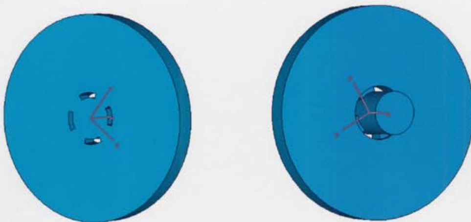
Figure 2-23: Model for phase sensor simulation.
