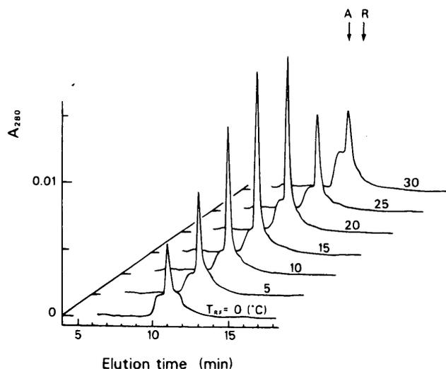
FIGURE 2: Elution profiles of the refolded Δ1 on RPHPLC. Each profile is labeled with the temperature,  $T_{RF}$ , at which the refolding reaction was carried out. 8.2  $\mu$ g of reduced Δ1 was refolded, filtered through a 0.2- $\mu$ m filter, and subjected to RPHPLC as described in Materials and Methods. Arrows A and R indicate the elution positions for authentic and reduced lysozymes, respectively.
