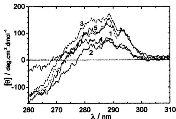
**Figure 2.** Near-UV CD spectra of 3SS-lysozymes. Spectra were measured in 50 mM sodium acetate buffer (pH 4.0) and 4.0°C. 1, (···) C6S/C127A; 2, (-·-) C30A/C115A; 3, (---) C64A/C80A; 4, (—) C76A/C94A; 5, (—) metLYZ.
