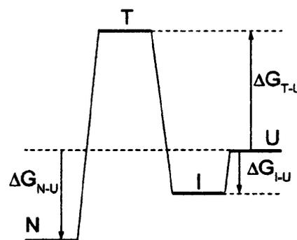
**Figure 9.** Free energy diagram of 3SS-lysozyme folding. T-state denotes the transition state, I-state the compact disordered state, N-state the native state and U-state the unfolded state.  $\Delta G$  represents the difference in Gibbs free energy between two states.
