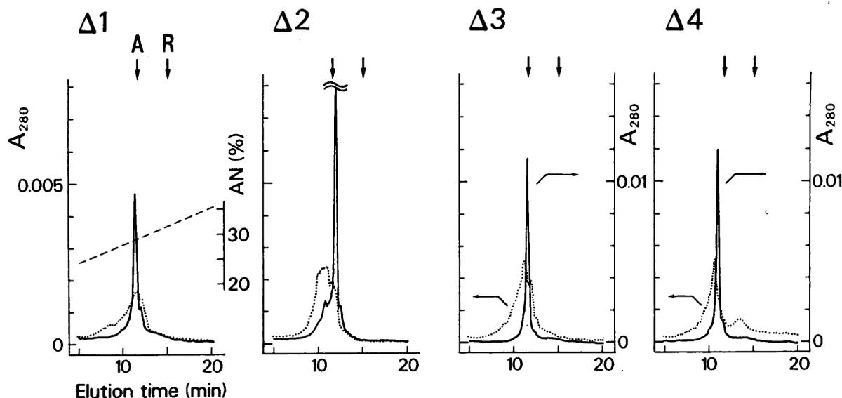
Fig. 2. Elution profiles of the 3SS-derivatives reoxidized at 37°C without glycerol (dotted lines) and those at 15°C with 20% glycerol (full lines). The gradients in acetonitrile are in broken lines. The amount of protein reoxidized was about 4  $\mu$ g, the filtrate of which was subjected to RPHPLC. A and R indicate the elution positions of authentic and reduced lysozymes, respectively.
