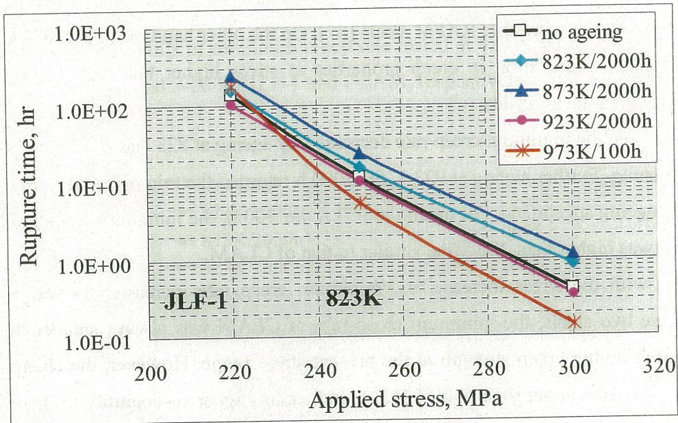
Fig. 3-27 Ageing effect on rupture time for JLF-1 (tested at **823 K**).
