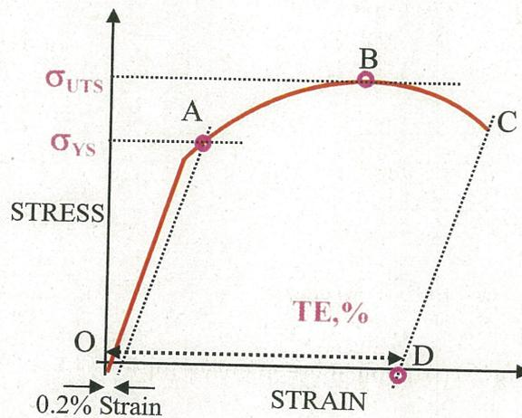
Fig. 2-8 Schematic illustration of the typical tensile curve for RAFM steels
