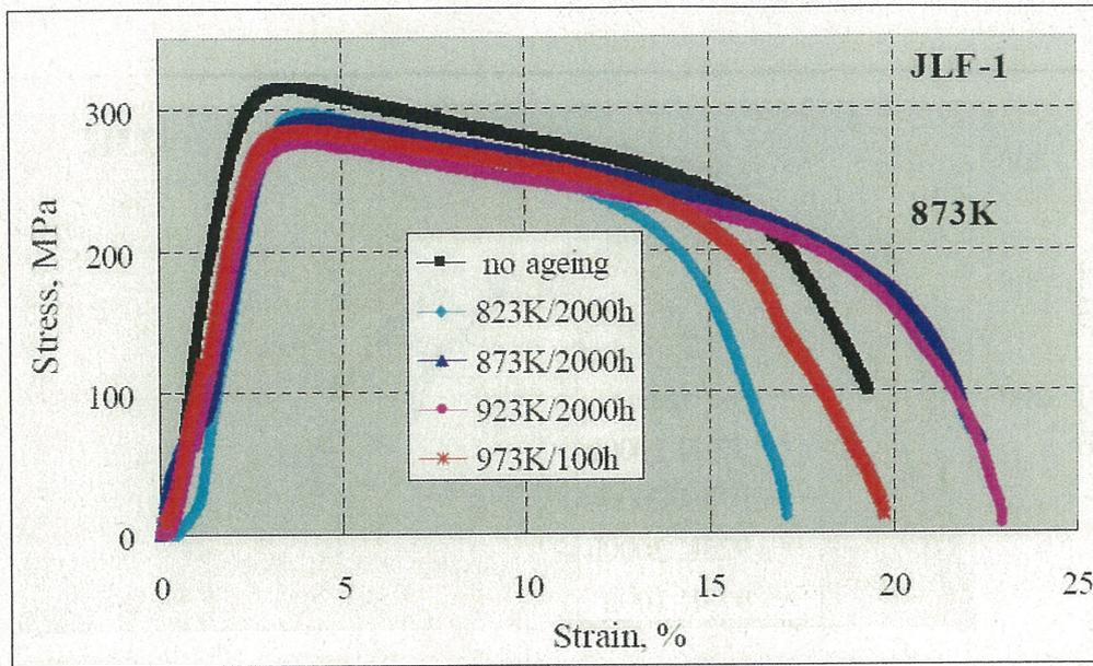
Fig. 3-11 Tensile curves for JLF-1 steel before and after different thermal ageing (tested at 873 K)
