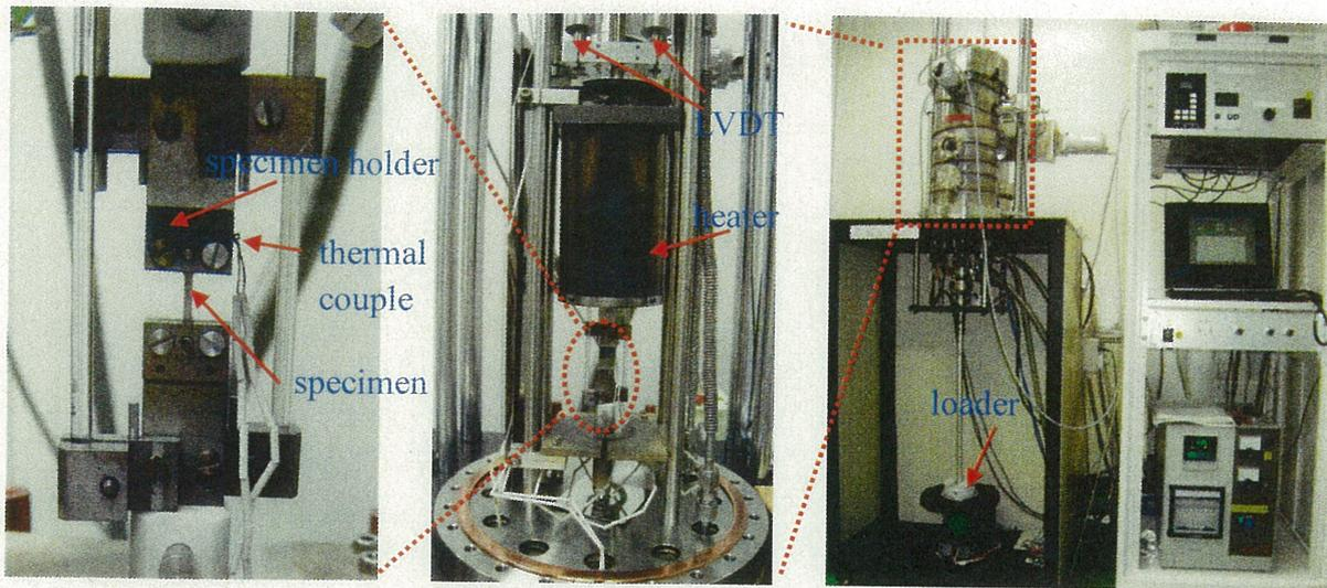
Fig. 2-11 View of the creep property test machine
