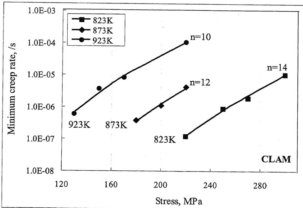
Fig. 3-31 Minimum creep rate vs. the applied stress for CLAM steel before ageing (from the lines slope the stress exponent  $n$  can be determined at each test temperature from 823 to 923 K).
