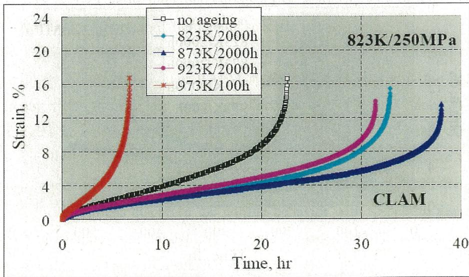
Fig. 3-22 Ageing effects on creep curves of CLAM steel (tested at **823K/250MPa**)
