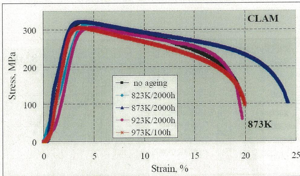
Fig. 3-12 Tensile curves for CLAM steel before and after different thermal ageing (tested at 873 K)
