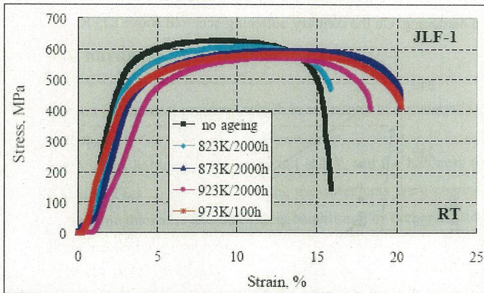
Fig. 3-3 Tensile curves for JLF-1 steel before and after different thermal ageing (tested at RT)
