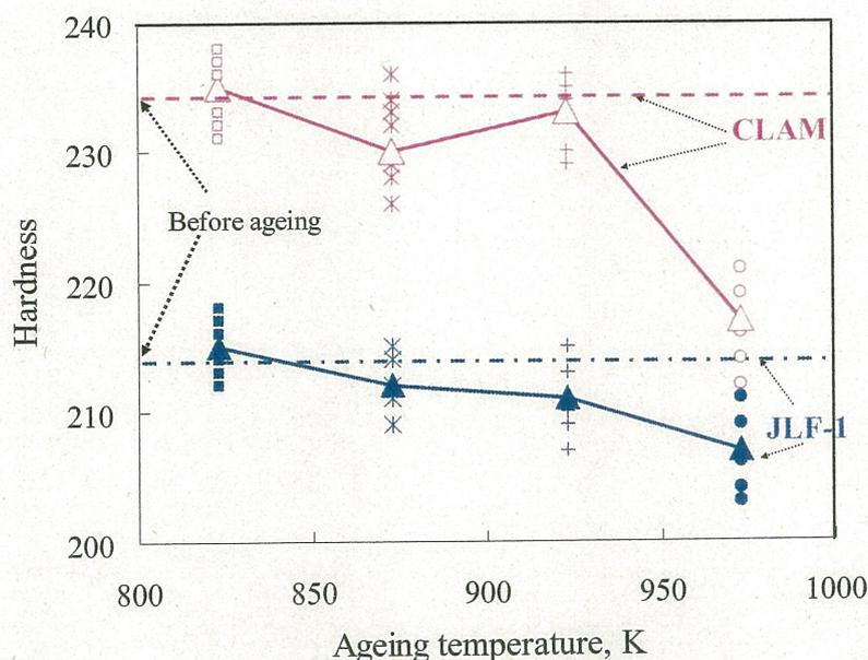
*Fig. 3-1* Hardness change of JLF-1 and CLAM steels after ageing for 100 h.
