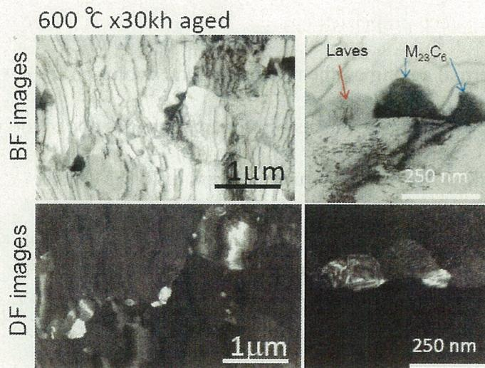
Fig.1-19 Large Laves phase is formed adjacent to  $M_{23}C_6$  for F82H steel after ageing at 600°C for 30 000 h [88].
