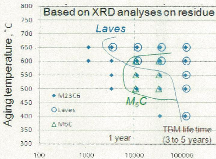
Fig.1-20 The Temperature - Time - Precipitates curves for F82H steel [88].
