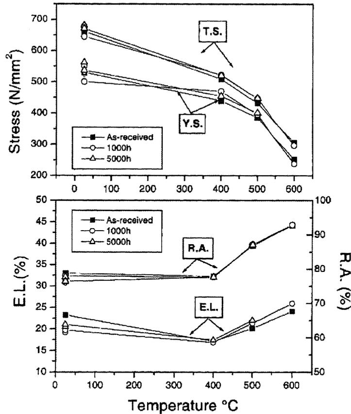
Fig. 1-14 Tensile properties of the EUROFER 97 steel in the as-received condition and after ageing at 400 and 500°C [84].
