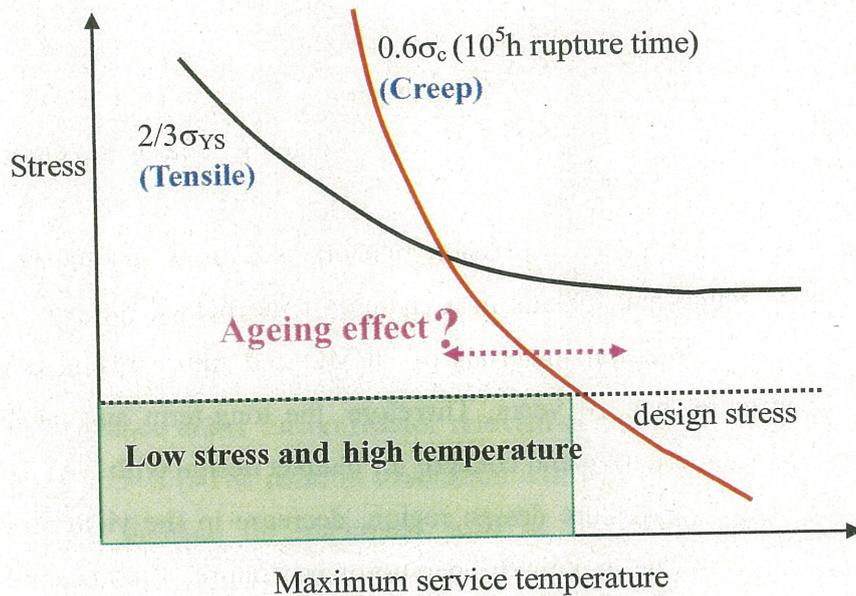
Fig. 1-11 Possible effect of thermal ageing on creep property for RAFM steels
