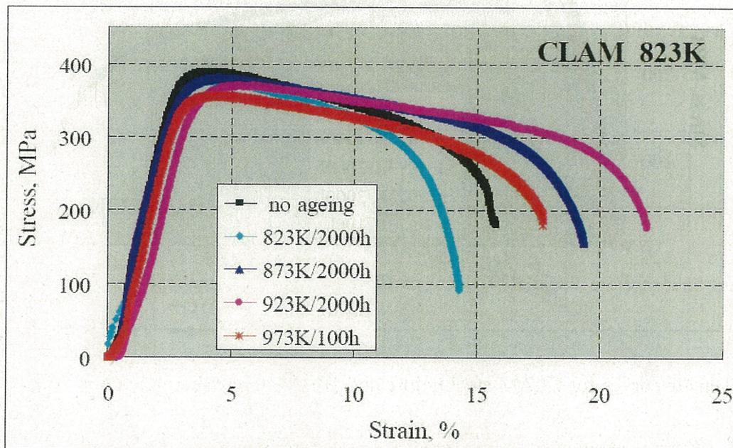
Fig. 3-10 Tensile curves for CLAM steel before and after different thermal ageing (tested at 823 K)
