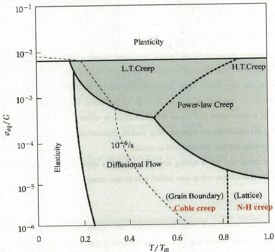
Fig. 3-29 Schematic deformation-mechanism map by Ashby ( $T_m$ : the melting temperature,  $G$ : shear modulus, L.T.Creep: low temperature creep, and H.T. Creep: high temperature creep) [91]
