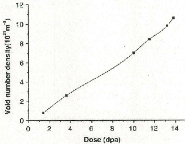
Fig.1-8 Dose dependence of void number density up to 13.8 dpa for irradiation at 723 K for CLAM steel [74].
