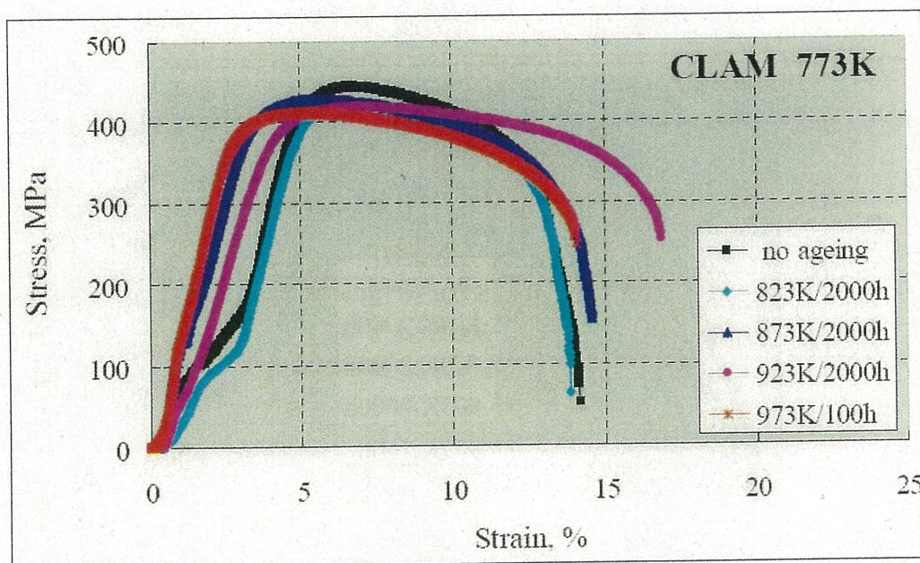
Fig. 3-8 Tensile curves for CLAM steel before and after different thermal ageing (tested at 773 K)
