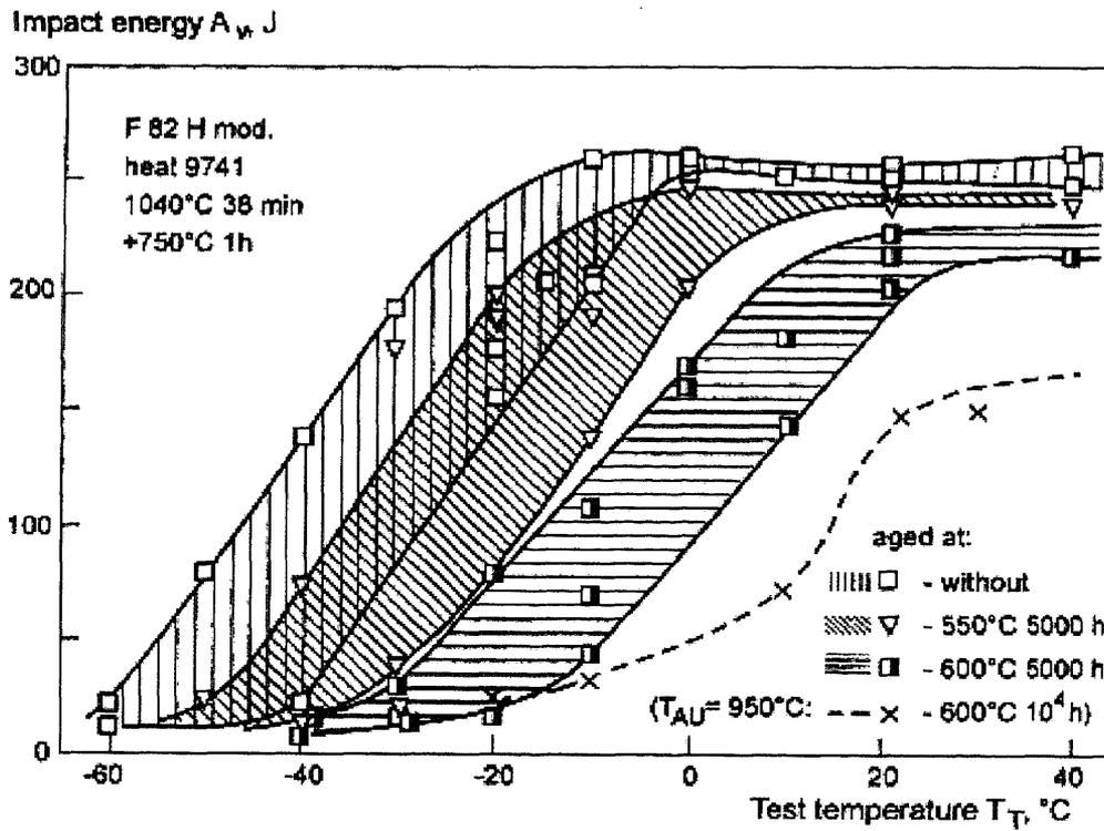
Fig. 1-15 Impact energy of the F82H-mod steel as a function of the test temperature showing an increase in DBTT (up to +68 K) after ageing [83].
