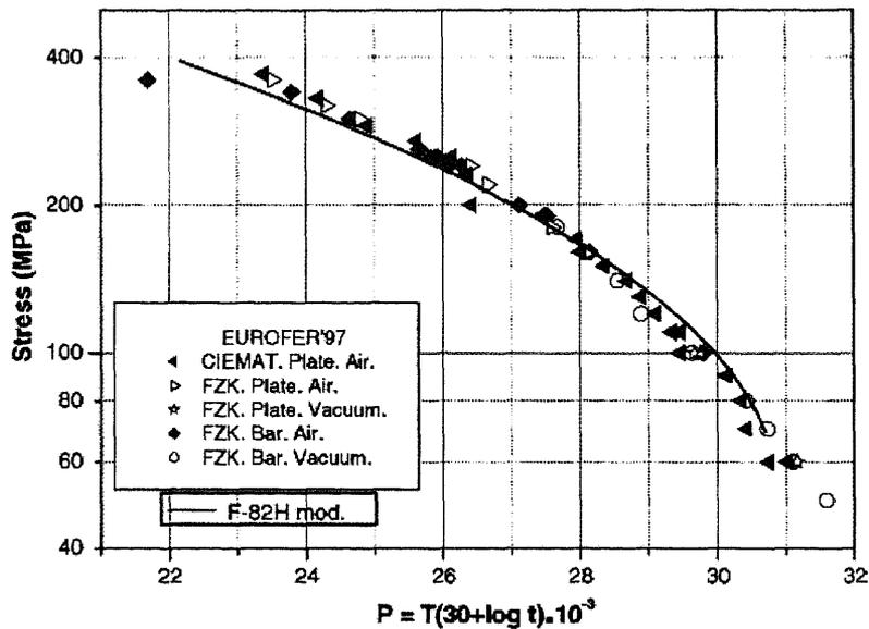
Fig.1-7 Larson-Miller parameter of the EUROFER 97 steel and the F82H-mod steel in the as-received condition [69].
