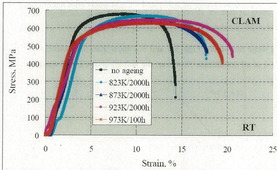
Fig. 3-4 Tensile curves for CLAM steel before and after different thermal ageing (tested at RT)
