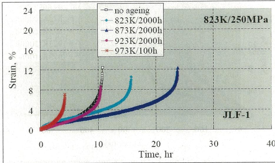
Fig. 3-21 Ageing effects on creep curves of JLF-1 steel (tested at **823K/250MPa**)
