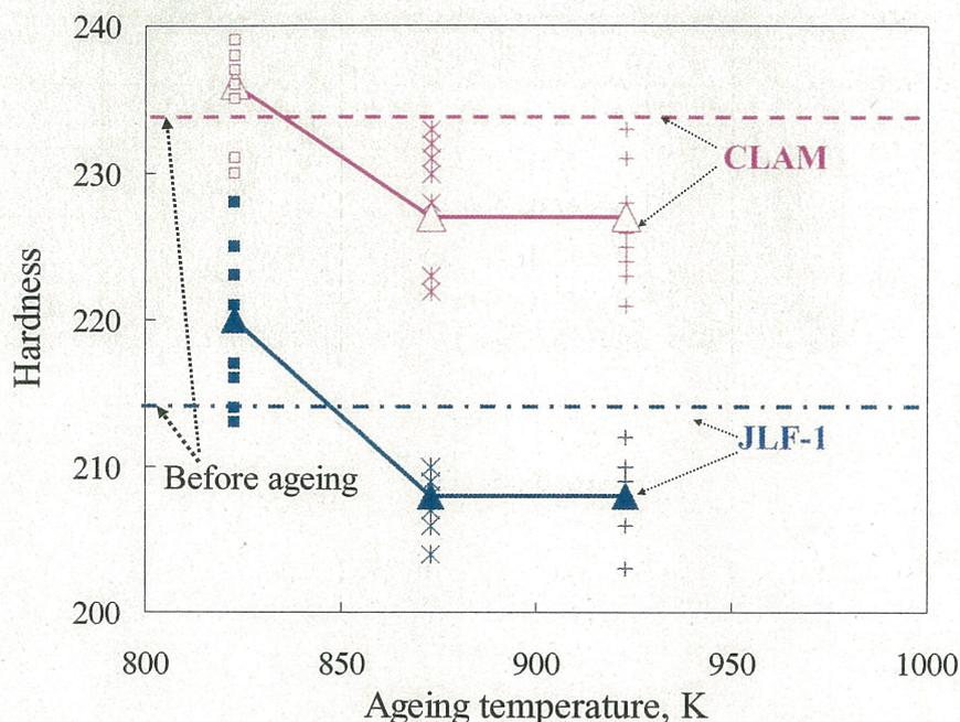
Fig. 3-2 Hardness change of JLF-1 and CLAM steels after ageing for 2000 h.
