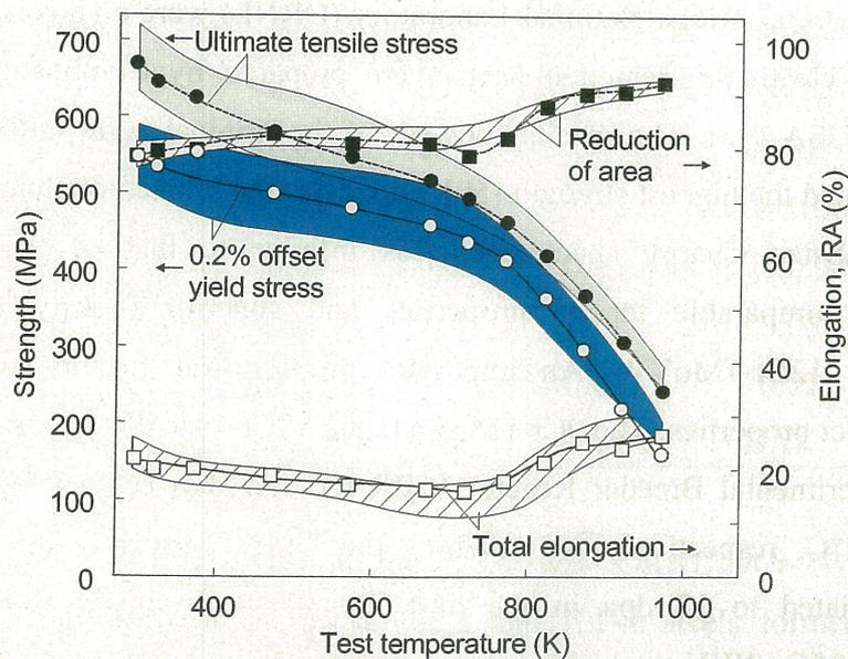
Fig. 1-4 Tensile properties of F82H IEA heat [64]
