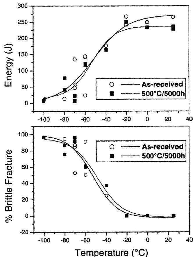
Fig. 1-17 Impact curves for the EUROFER 97 steel in the as-received condition and after ageing at 500°C for 5000 h [84].
