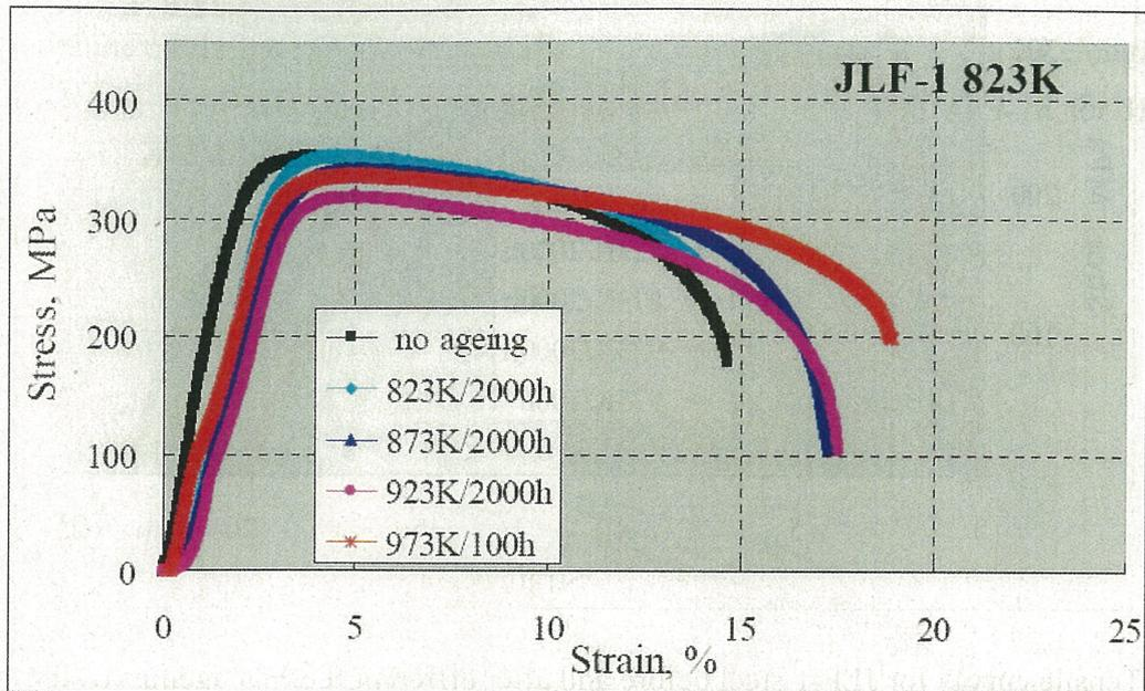
Fig. 3-9 Tensile curves for JLF-1 steel before and after different thermal ageing (tested at 823 K)
