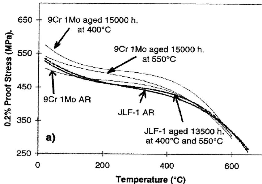
Fig.1-13 Evolution of the 0.2% proof stress (yield stress) with ageing of JLF-1 at normalization and tempering (N&T) initial conditions compared with other steels [79].
