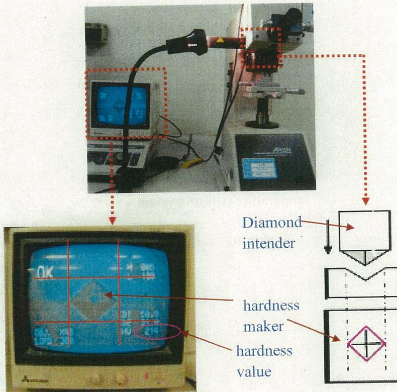
Fig. 2-7 Vickers hardness test machine
