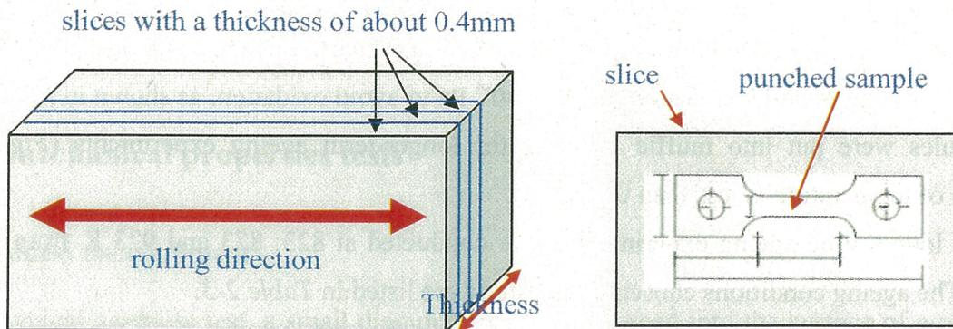
Fig.2-3 Preparation process for samples: sliced and punched
