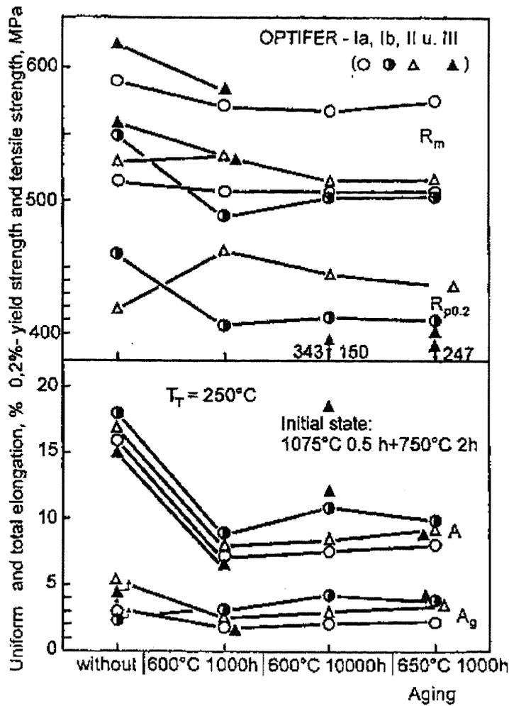
Fig. 1-12 Tensile properties at 250°C of the steels OPTIFER-Ia, Ib, II and III after ageing [83]. The OPTIFER steels have a basic compositions of 9Cr-0.1C-0.25V-0.5Mn with different contents of W and Ta (Ia: 1%W + 0.066%Ta, Ib:1%W+0.163%Ta, II:0.018%Ta, and III:1.6%Ta).  $R_m$ : ultimate tensile strength,  $R_{p0.2}$ : yield strength, A: total elongation and  $A_g$ : uniform elongation).
