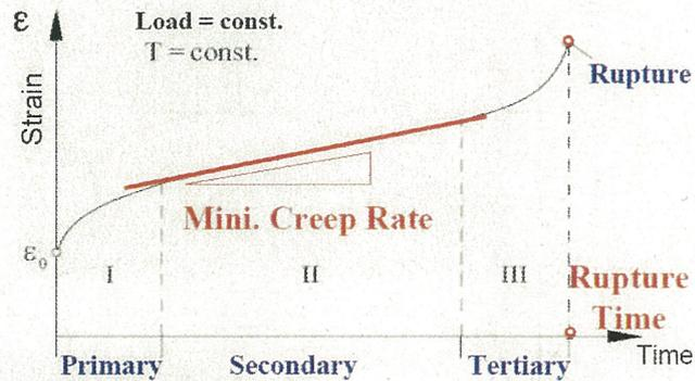
Fig. 2-10 Typical creep curve for RAFM steels
