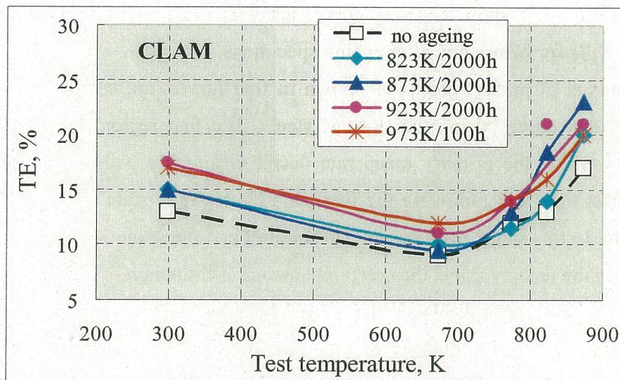
Fig. 3-18 Effect of thermal ageing on total elongation (TE) for CLAM
