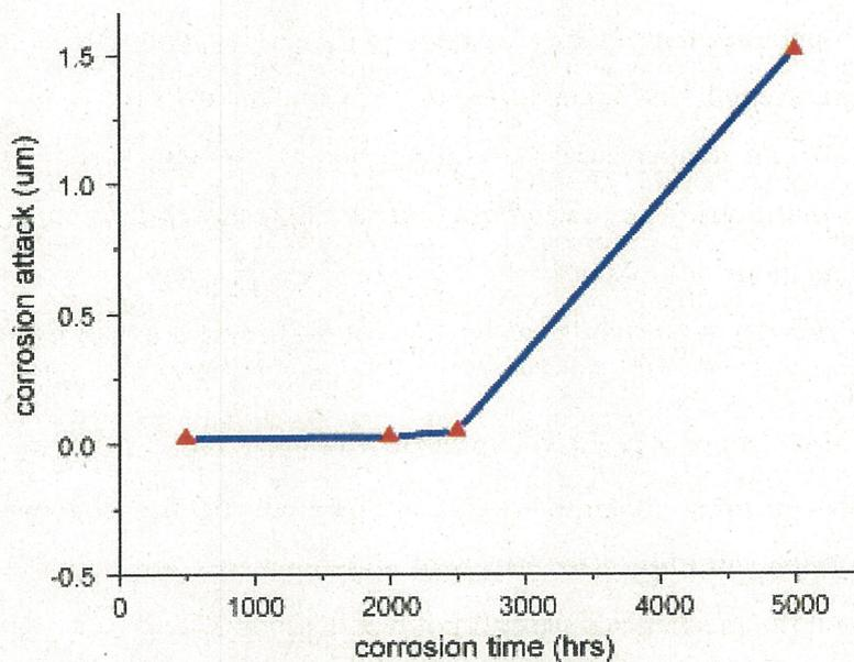
Fig.1-9 Metal weight loss vs. exposure time for CLAM in flowing LiPb loop [72].
