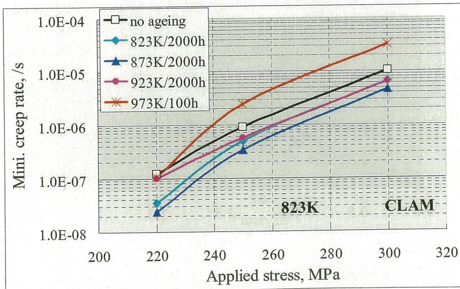
Fig. 3-26 Ageing effects on minimum creep rate for CLAM steel (tested at 823K)
