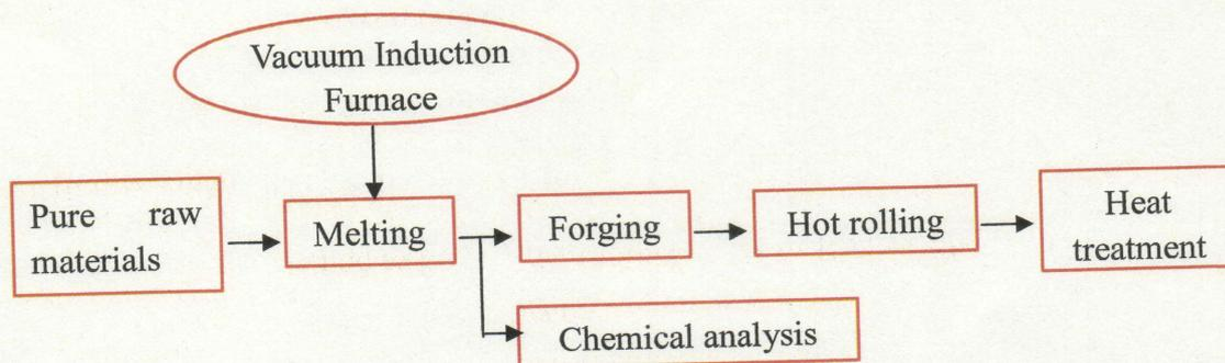
Fig. 2-1 Flow chart for the preparation of CLAM steel
