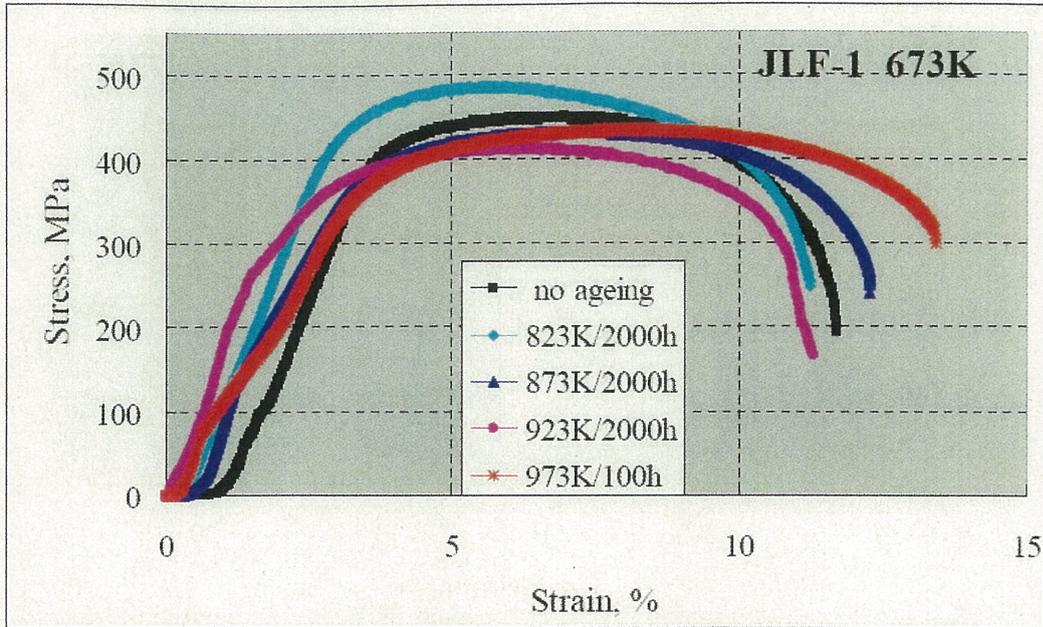
Fig. 3-5 Tensile curves for JLF-1 steel before and after different thermal ageing (tested at 673 K)
