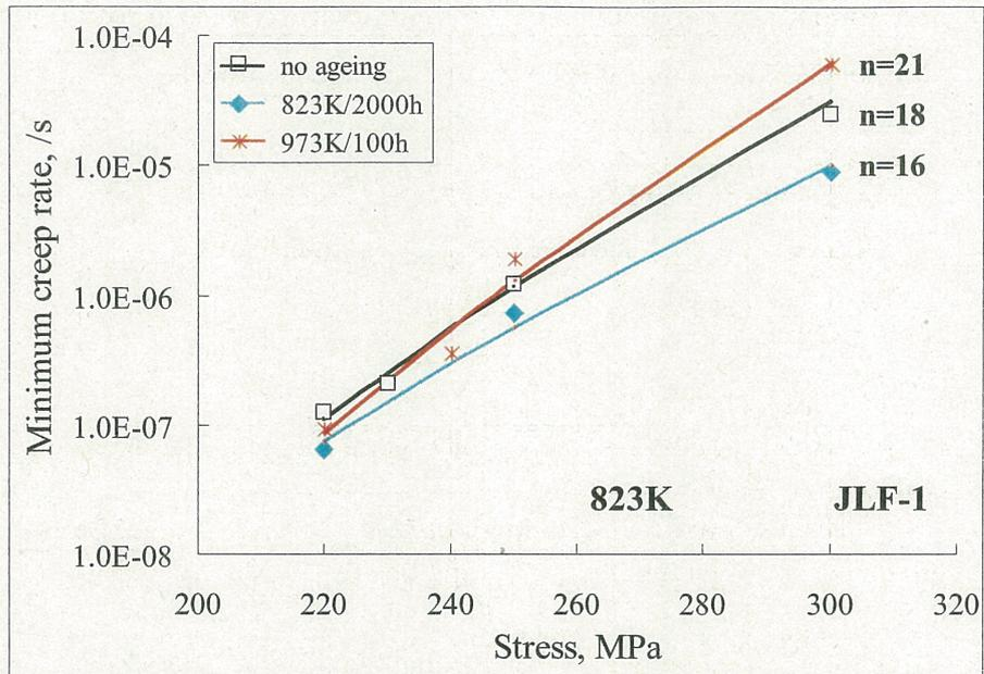
Fig. 3-32 Minimum creep rate vs. applied stress for JLF-1 steel after ageing, compared with that no ageing (from the slope the stress exponent  $n$  can be determined at test temperature of 823 K)
