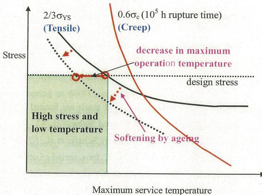
Fig. 1-10 Possible softening of tensile stress by thermal ageing
