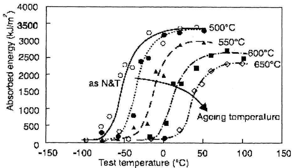
Fig. 1-16 Absorbed impact energy of F82H after ageing for 10000 h at indicated temperatures [82]
