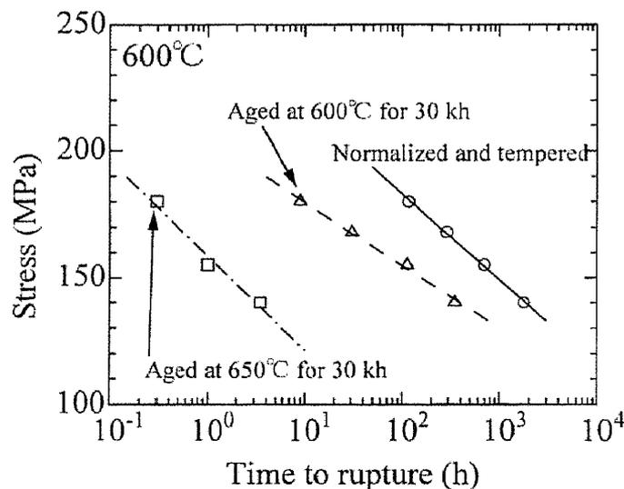
Fig. 1-18 Stress vs. time to rupture diagram for pre-F82H IEA steel
