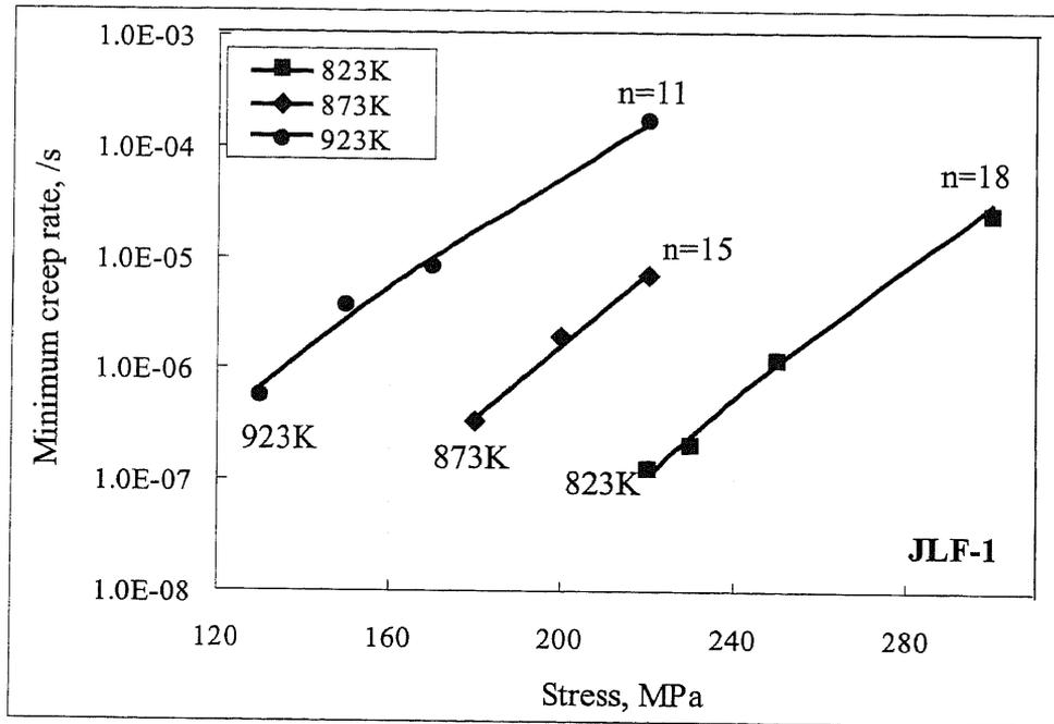
Fig. 3-30 Minimum creep rate vs. the applied stress for JLF-1 steel before ageing (from the lines slope the stress exponent  $n$  can be determined at each test temperature from 823 to 923 K).
