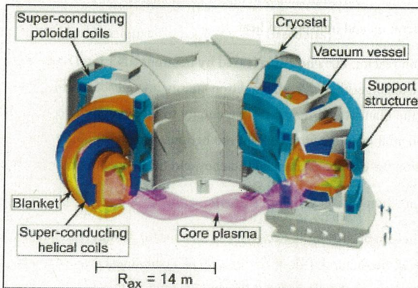
Fig. 1-3 The 3-D illustration of the FFHR2m1, the Helical-type DEMO reactor [16]
