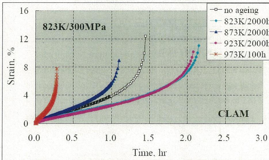
Fig. 3-24 Ageing effects on creep curves of CLAM steel (tested at **823K/300MPa**)
