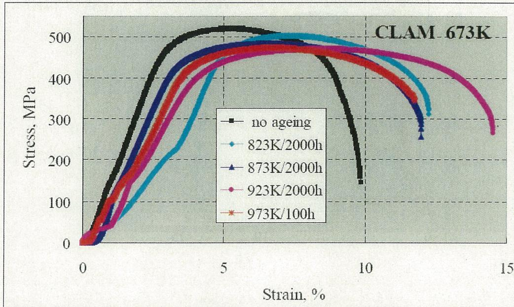
Fig. 3-6 Tensile curves for CLAM steel before and after different thermal ageing (tested at 673 K)
