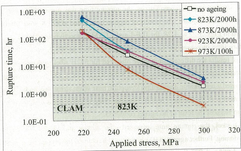
Fig. 3-28 Ageing effect on rupture time for CLAM (tested at **823 K**).
