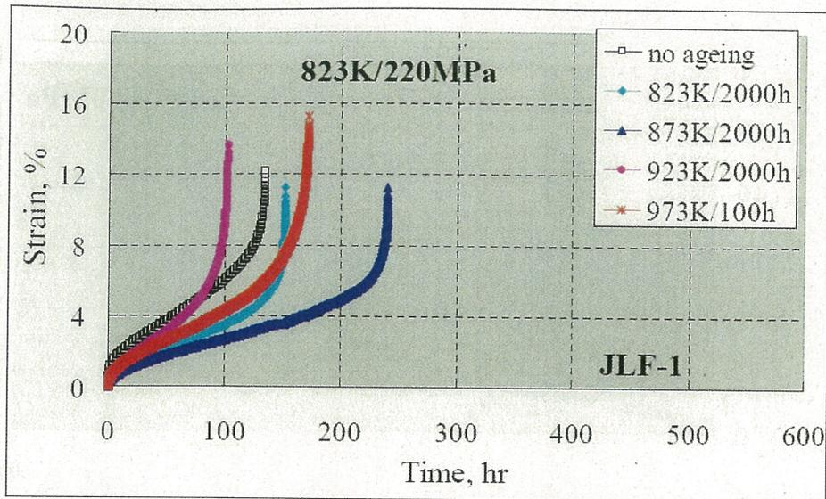
Fig. 3-19 Ageing effects on creep curves of JLF-1 steel (tested at **823K/220MPa**)
