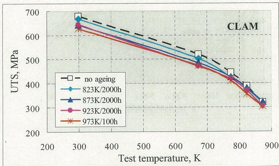
Fig. 3-14 Effect of thermal ageing on ultimate tensile strength (UTS) for CLAM
