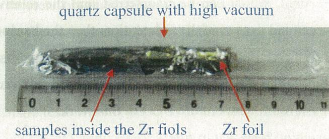
Fig. 2-5 Samples were sealed in quartz capsule under high vacuum
