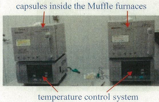
Fig. 2-6 Capsules were inside in Muffle furnaces for long time ageing experiments
