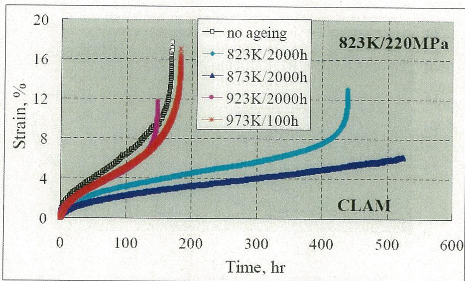
Fig. 3-20 Ageing effects on creep curves of CLAM steel (The sample aged at 873k/2000h did not run to rupture) (tested at **823K/220MPa**)
