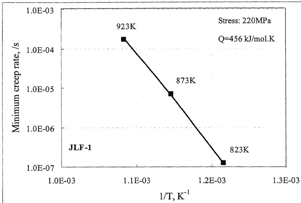
Fig. 3-34 The dependence of minimum creep rate on 1/T for JLF-1 before ageing, from which the activation energy Q of 456 kJ/mol-K was obtained.
