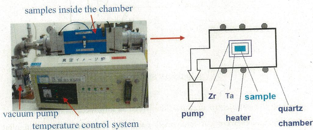
Fig. 2-4 Infrared image furnace for short time ageing experiments
