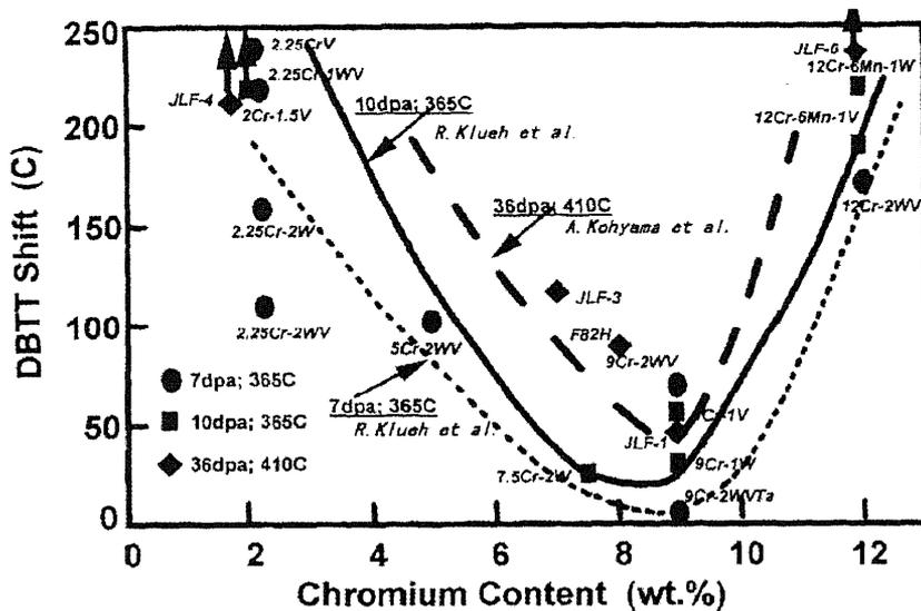
Fig.1-6 Effects of Cr content on DBTT shift for low activation ferritic steels by neutron irradiation in FFTF [66].
