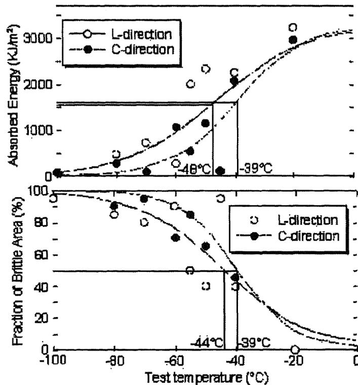
Fig. 1-5 Charpy impact test results of F82H IEA heat [64].
