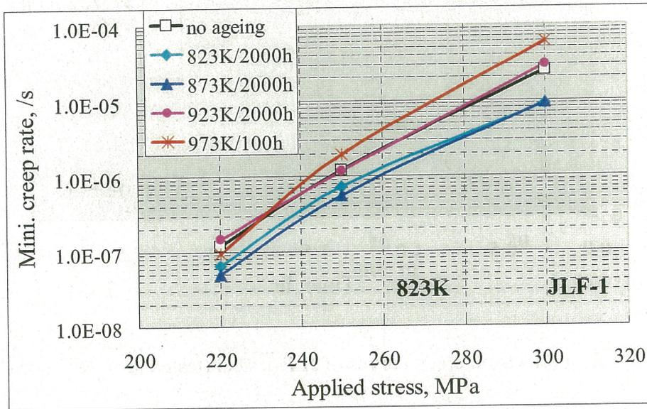
Fig. 3-25 Ageing effects on minimum creep rate for JLF-1 steel (tested at 823K)
