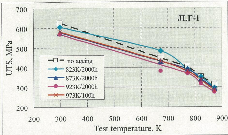
Fig. 3-13 Effect of thermal ageing on ultimate tensile strength (UTS) for JLF-1
