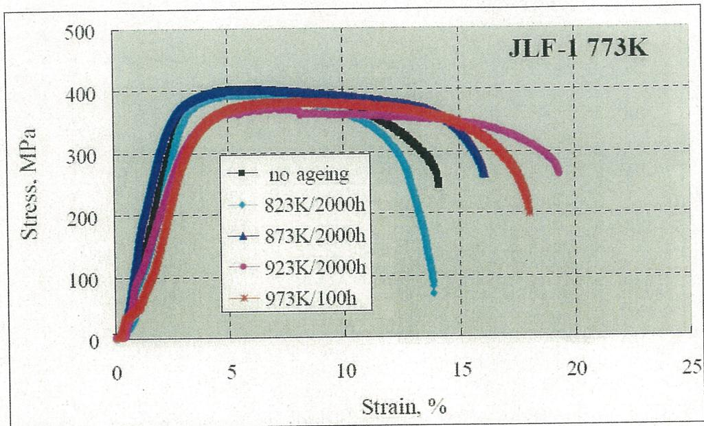
Fig. 3-7 Tensile curves for JLF-1 steel before and after different thermal ageing (tested at 773 K)
