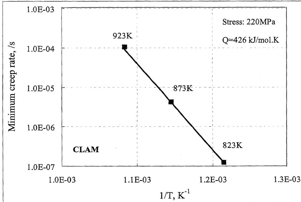
Fig. 3-35 The dependence of minimum creep rate on 1/T for CLAM before ageing, from which the activation energy Q of 426 kJ/mol-K was obtained.
