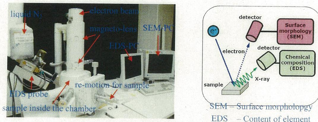
Fig. 2-13 SEM for the microstructure observation
