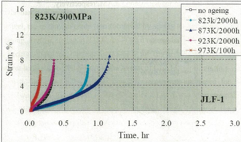
Fig. 3-23 Ageing effects on creep curves of JLF-1 steel (tested at **823K/300MPa**)
