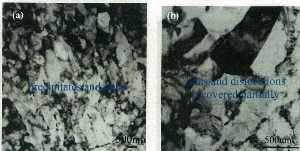
Fig. 4-17 TEM micrographs for CLAM after ageing at 923 K for 2000 h :
