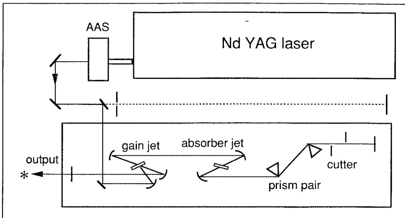
Figure II-1. Homemade passive mode-locked dye laser synchronously pumped by Nd YAG laser. AAS stands for active amplitude stabilizer.
