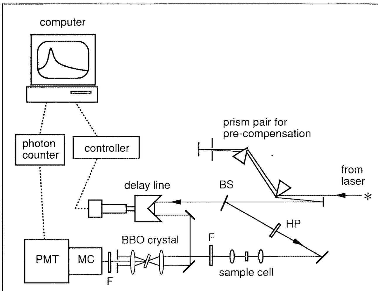
Figure II-2. Fluorescence up-conversion system for the dye laser. BS: beam splitter, HP: half-wave plate, F: filter, MC: monochromator, and PMT: photo multiplier tube.
