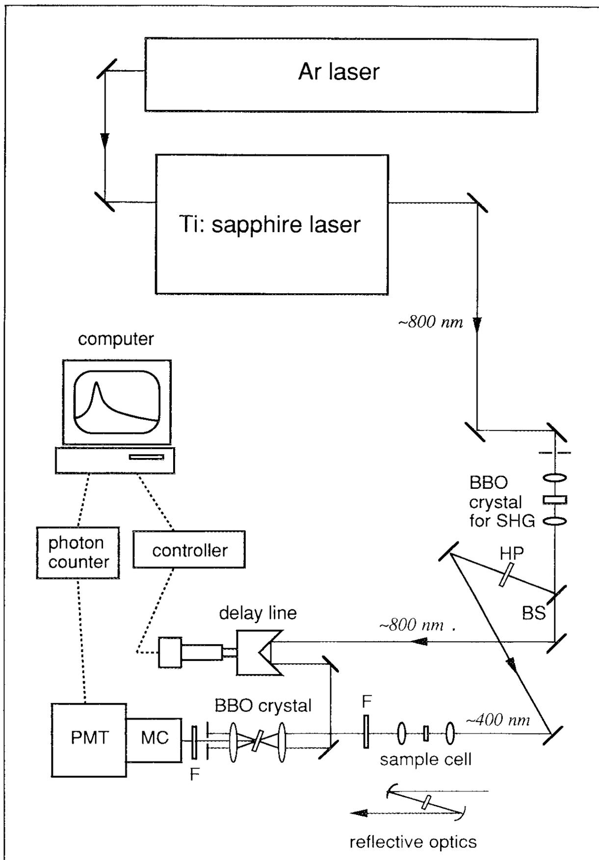
Figure II-3. Fluorescence up-conversion system for the Ti: sapphire laser. SHG: second harmonic generation, BS: beam splitter, HP: half-wave plate, F: filter, MC: monochromator, and PMT: photo multiplier tube.
