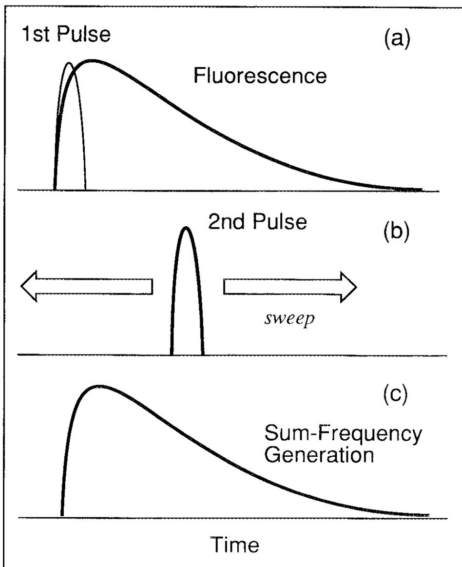
Figure II-5. Principle of fluorescence up-conversion method. (a) Fluorescence is generated by the first pulse. (b) The delay between the first and second pulse is varied. (c) Sum-frequency is generated between the fluorescence and the second pulse. If the intensities of the pulses do not change, the intensity of the sum-frequency will be proportional to the intensity of the fluorescence.
