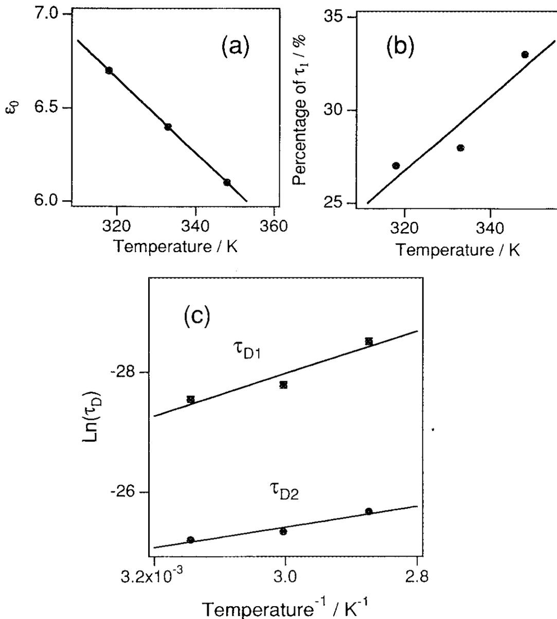
Figure III-6. Temperature dependence of (a)  $\epsilon_0$ , (b) percentage of the first Debye relaxation time  $\tau_1$  (%), and (c) Debye relaxation times  $\tau_1$  and  $\tau_2$  of AN, plotted from the experimental results of Bhattacharyya *et al.* (*J. Phys. Soc. Jap.*, **28**, 204, (1970)).
