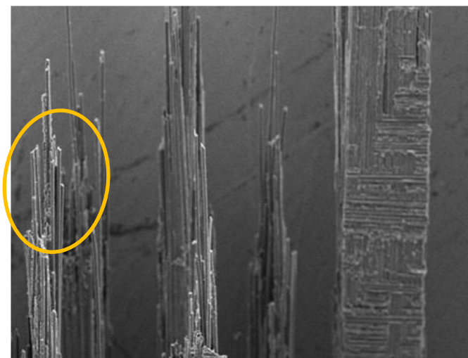
Fig. 6.8: (HTT): 3173K, t_i : 13MPa. Fracture occurs in small fibre bundles (FB)
