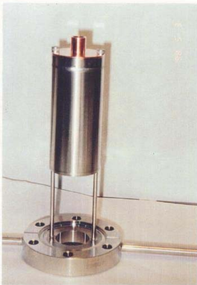
Photo 3.3. Picture of the evaporator with water-jacket and collimator. This part along with the electrical feedthroughs is inserted into the preparation chamber.
