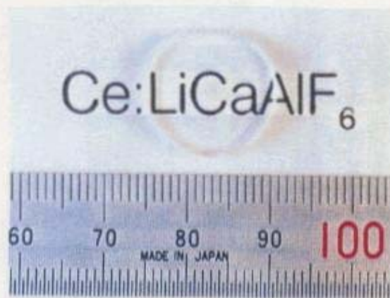
Fig. 5.1 Photograph of the large Czochralski-grown Ce:LiCAF crystal with 15-mm diameter.
