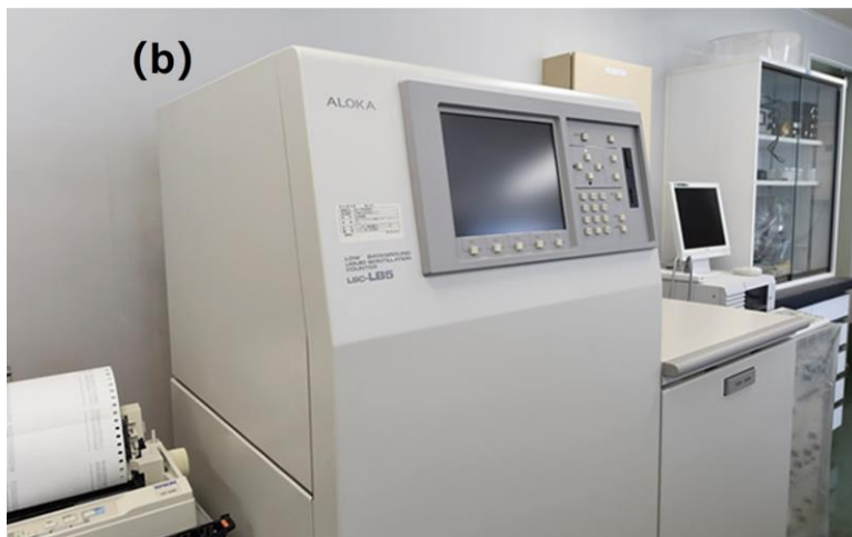
Fig. 1-4. Typical devices for measuring hydrogen isotope. (a) Isotope-ratio mass spectrometry [1-7]. (b) Liquid scintillation counter [1-8].
