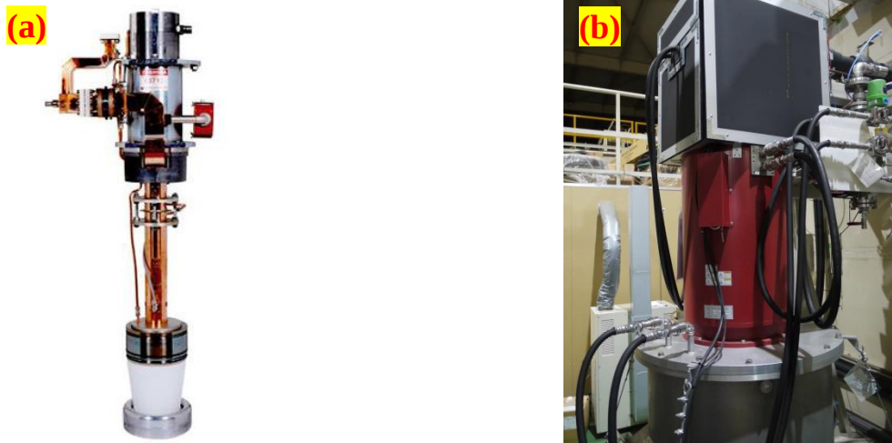
Figure 14: Toshiba 3712 klystron: (a) is the klystron without cover, (b) is the klystron with cover
