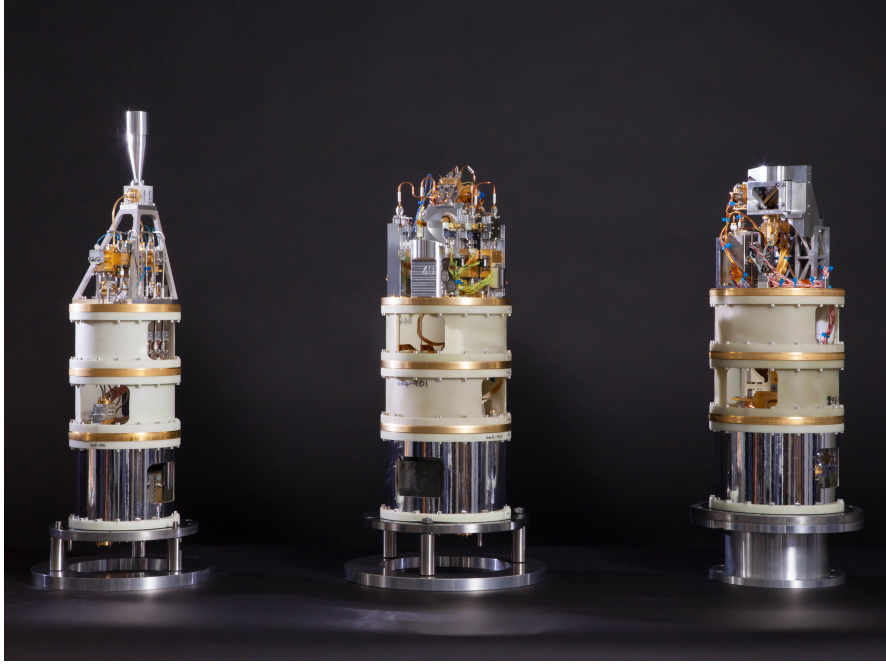
Fig. 1.1 ALMA receiver cartridges. Left: Band 4 (125-163GHz), Center: Band 8 (385-500GHz), Right: Band 10 (787-950GHz). Photo credit: ALMA(ESO/NAOJ/NRAO). https://www.nao.ac.jp/en/gallery/weekly/2014/20140701-alma-receivers.html
