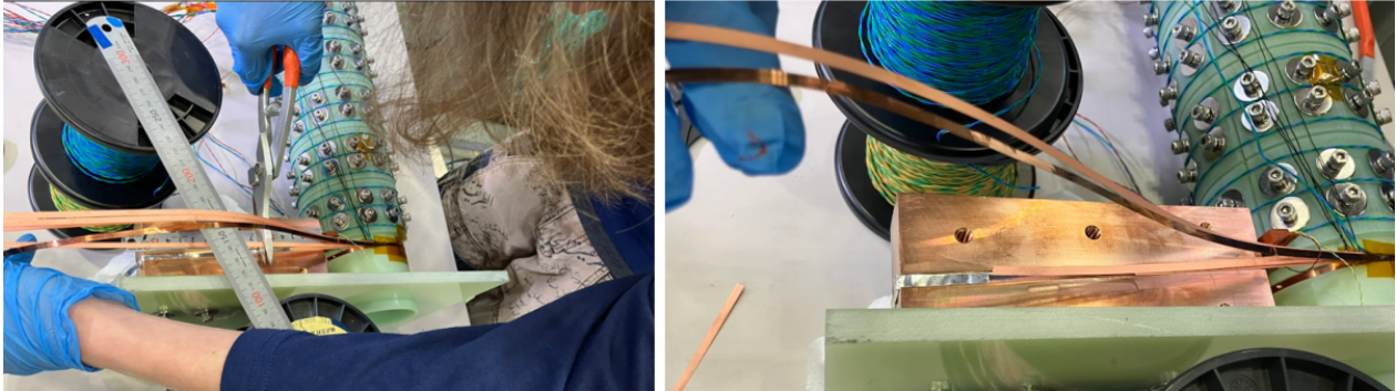
Figure 64: L-RAISER Case 2. The configuration was changed from NUCD to uniform current distribution. The REBCO tapes were cut in a staircase shape, and the step gaps filled with indium foil. The lower resistance via the indium foil facilitates a more uniform current distribution, by eliminating intermediate REBCO tapes that have the more-resistive hastelloy substrate embedded.
