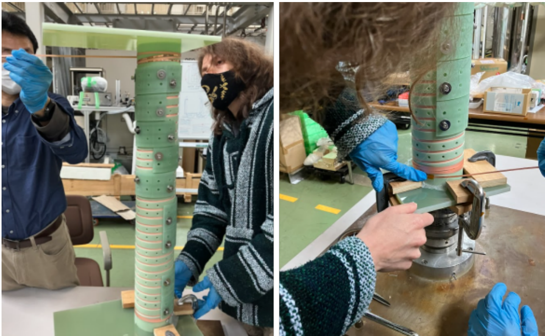
Figure 51: L-RAISER Assembly 3. Left: Starting the winding of one HTS tape, wound from top to bottom. Right: After finishing the winding of each HTS tape, they are temporarily secured with Kapton tape, before attaching them to the current leads.
