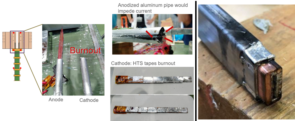
Figure 33: Quench experienced in simple-stacking HTS conductors. Left: A NUCD may have enhanced localized heating in the current lead, rising the temperature that led to a quench [118]. Right: For STARS conductor, a mistake in the quench detection led to a late response when a quench was starting, that led to damage and burning of the sample.
