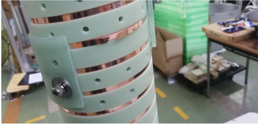
Figure 52: L-RAISER Assembly 4. Outer copper cushion tape wound after the 5 HTS tapes, for mechanical damage protection from pressure plates to HTS tapes. As the copper tapes were 5 m long, unlike the 10+ m from the HTS tapes, two copper tapes per layer were used.
