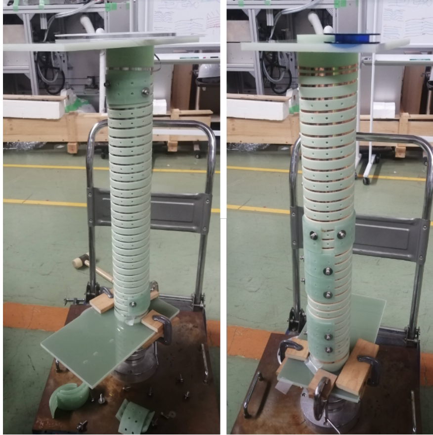
Figure 49: L-RAISER Assembly 1. Left: Dummy steel tape used for preliminary winding practice. Right: Copper tape, first tape in the stack, used as cushion and stabilizer to protect the HTS tapes from mechanical damage by the pressure plates.
