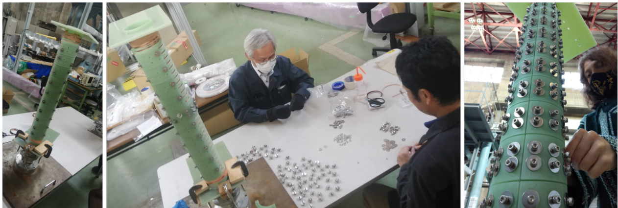
Figure 53: L-RAISER Assembly 5. Left: 5 HTS tapes plus 2 copper tapes wound and secured by pressure plates. Center: Preparation of bolts to collocate all the pressure plates in the bobbin. Right: Finalizing process for all bolts to secure and press the HTS tapes, to reduce contact resistance and have good current transfer among them.
