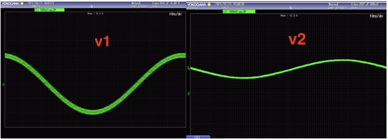
Figure 4.11: Kaladin output noise reduction from version 1 (left) to 2 (right).
