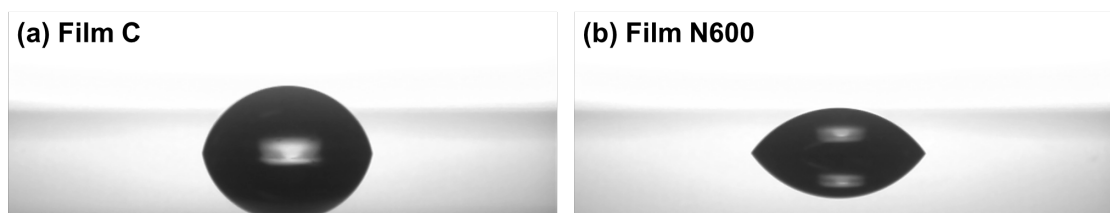
Figure 5.3 Static water contact angle measurements for carbon thin films: (a) Film C and (b) Film N600.
