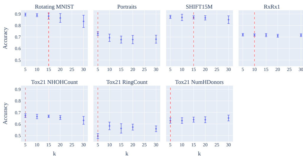
Figure 4.7: Experimental result of the training of our flow-based model with various hyperparameter k values. The appropriate k can be determined roughly by the fitting of the k NN classifier on the source dataset.
