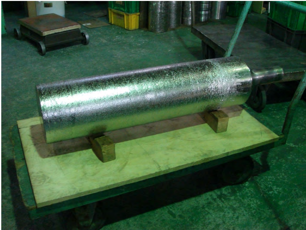
Fig. 2.4: Nb ingot with a base plate in the right side. The base plate is cut off by a saw and reused in the next melting process.
