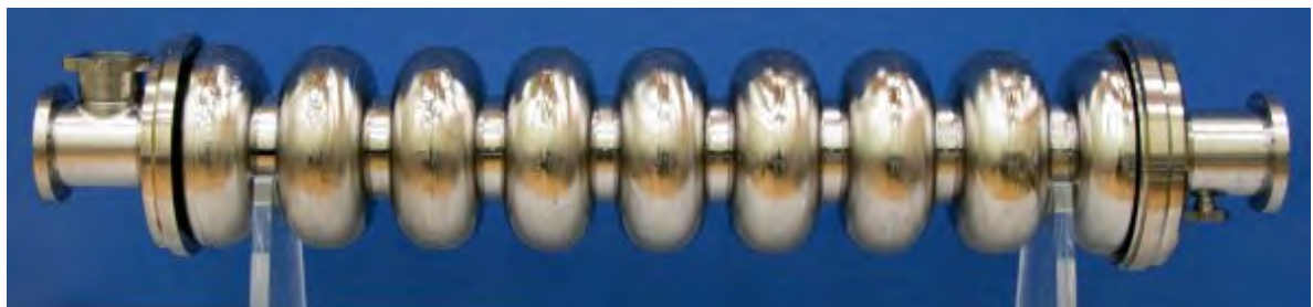
Fig. 4.1: 1.3 GHz SRF cavity made by LG niobium (KEK-2) [1].
