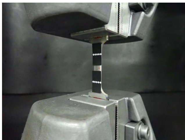
Fig. 3.6: Tensile testing specimen with gauge markers for video extensometer. Marker displacement is tracked to obtain continuous strain data until fracture.
