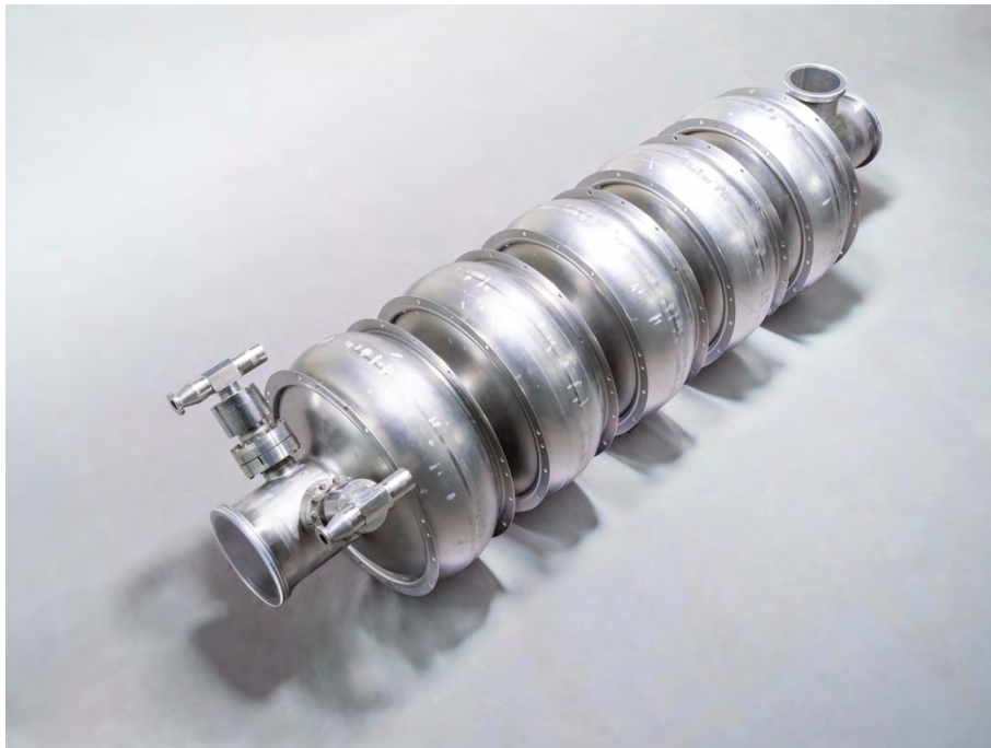
Fig. 1.1: TRISTAN MR superconducting cavity. TRISTAN was the first large-scale, practical application of SRF cavities made from high-purity niobium. This milestone accelerated the worldwide adoption of the SRF technology.
