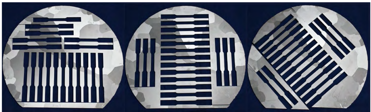
Fig. 4.3: Layout of tensile testing specimens cut from LG niobium disks (LG2) with random crystal orientations. Outer diameter: 240 mm, thickness: 2.8 mm.
