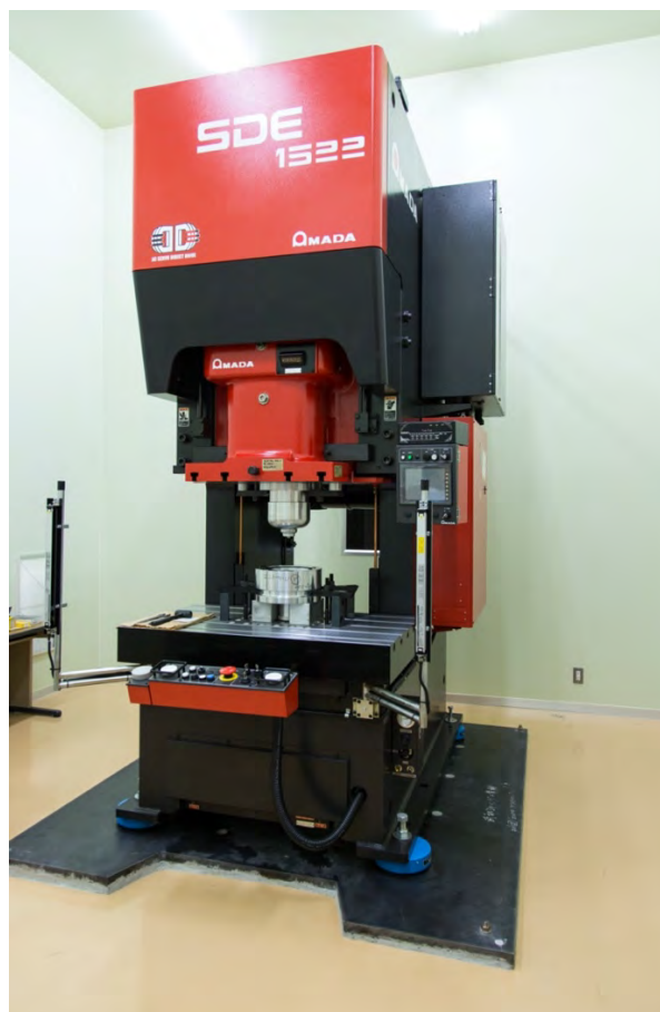
Fig. 3.15: Press-forming machine used for half-cell forming.
