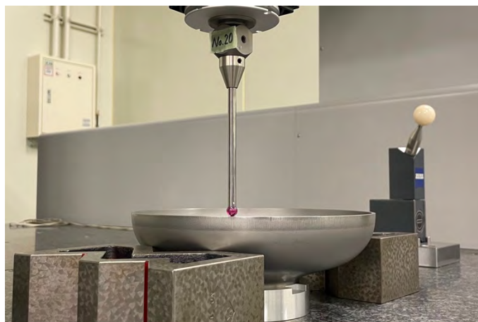
Fig. 3.19: Measurement of half-cell shape using a coordinate measuring machine. The equator region is scanned by probe.
