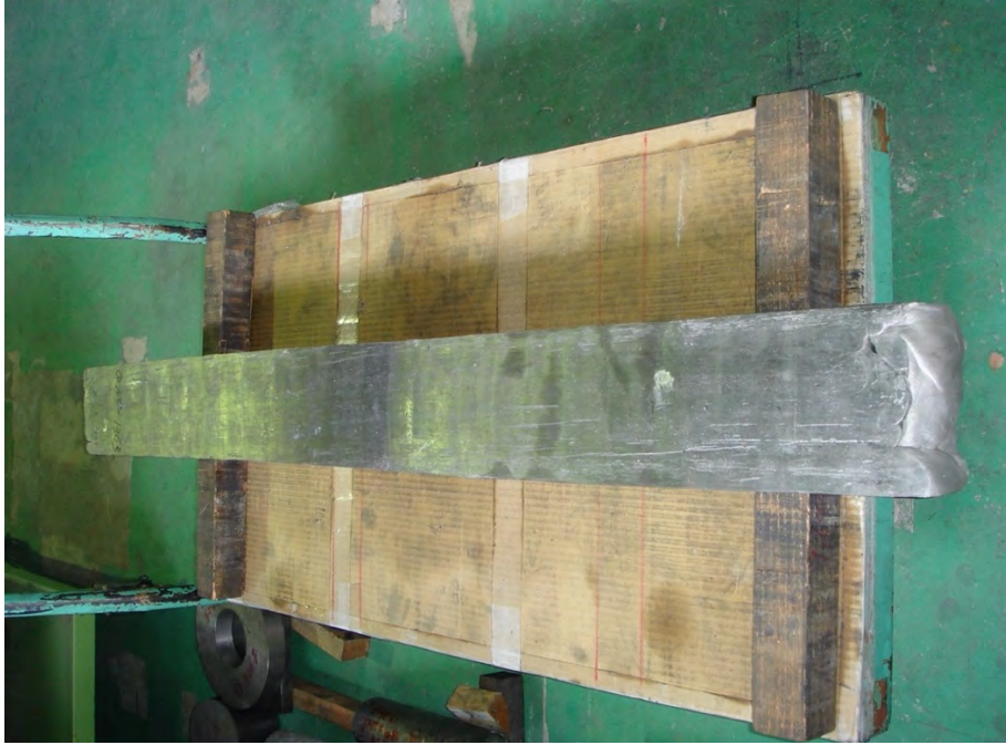
Fig. 2.5: Forged Nb. The cylindrical ingot is forged into a rectangular prism.
