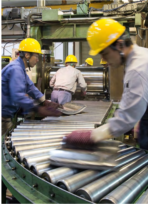
Fig. 2.7: Rolling process. Pass the material between the upper and lower rollers, repeating this process to achieve the desired thickness.
