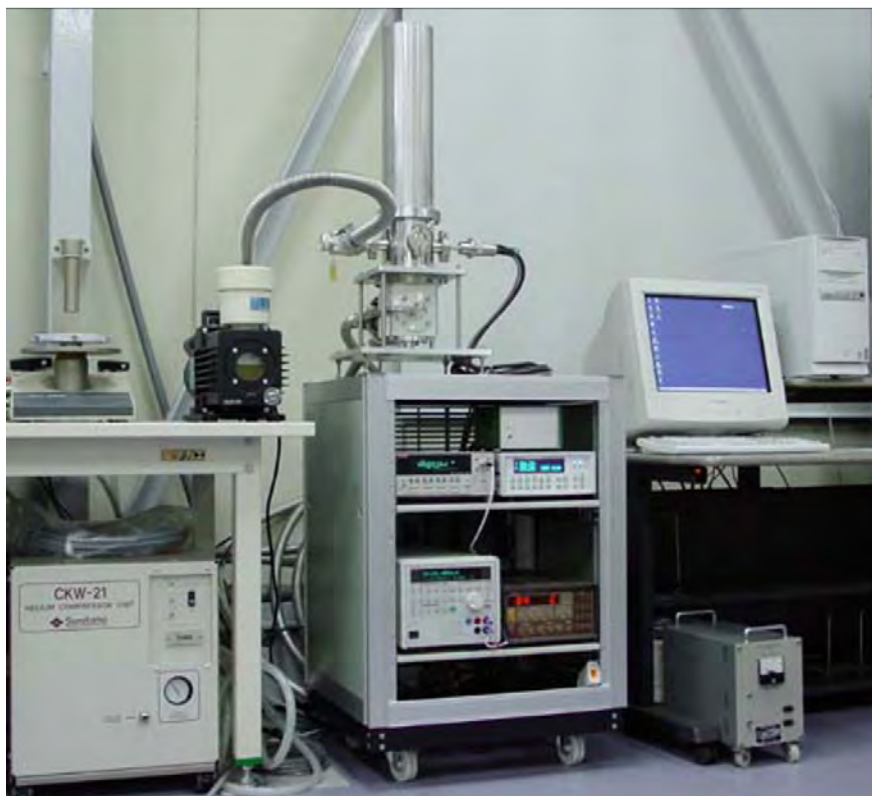
Fig. A.28: RRR measurement system cooled by refrigerator.
