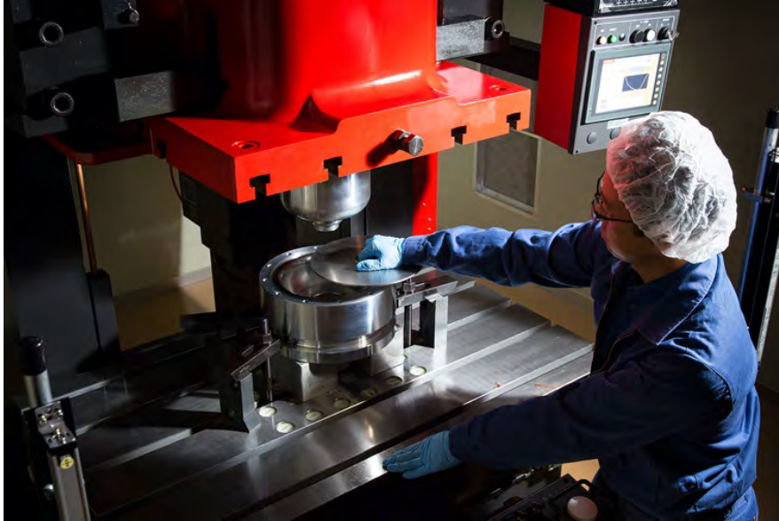
Fig. 3.16: Press forming process for half-cells.
