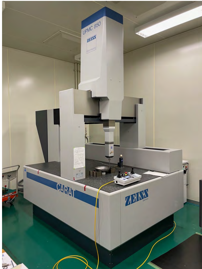
Fig. 3.18: Coordinate measuring machine used for roundness measurement for the equator region.
