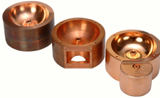
Fig. A2.2: Linac cavity at various stage of fabrication
