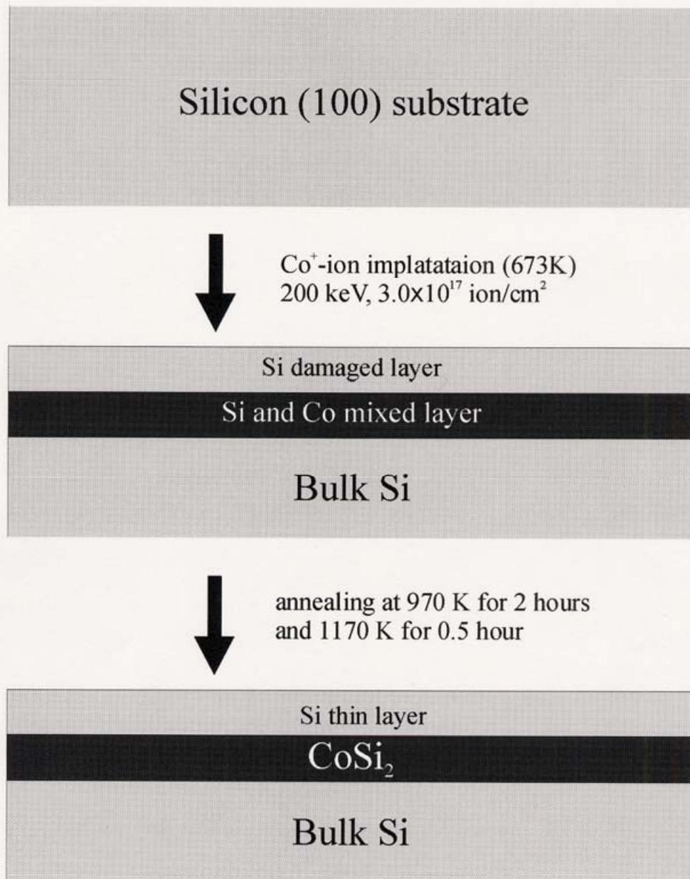
Figure 2.6: BML substrates fabrication procedure using ion implantation method.
