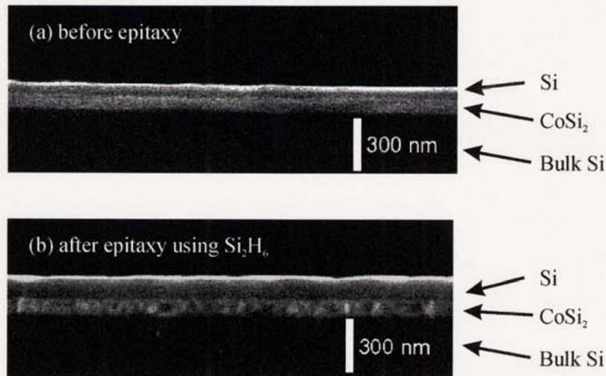
Figure 2.8: Cross-sectional structure observed by SEM of BML sample (a) before epitaxy and (b) after epitaxy using  $\text{Si}_2\text{H}_6$
