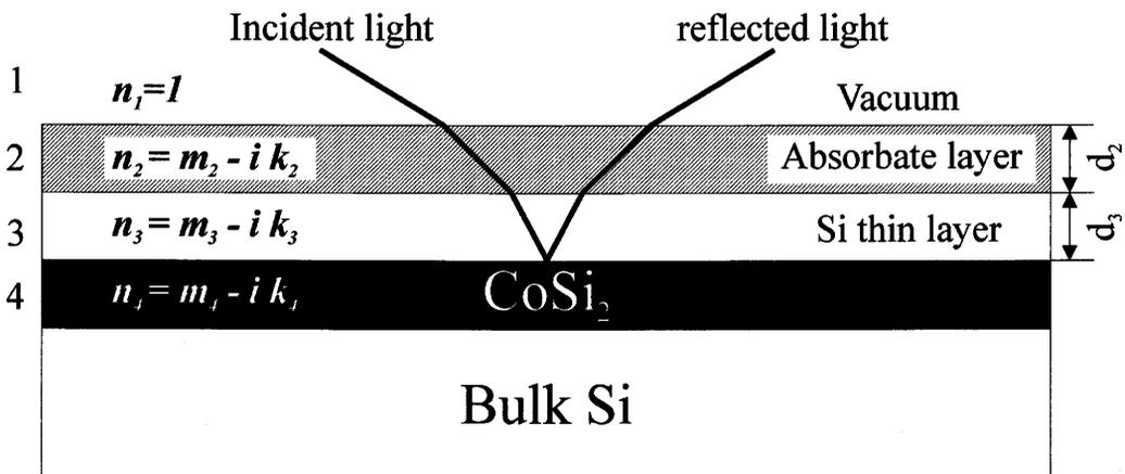
Figure 2.3: The principle of the BML-IRRAS. 1, 2, 3 and 4 represent the vacuum region 1, the layer 2, the layer 3 and the layer 4, respectively.
