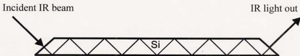
Figure 2.2: Arrangements of ATR or MIR method.
