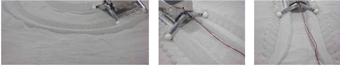
Figure 4.18 : Various rut formations by the prototyped rover on sand.
