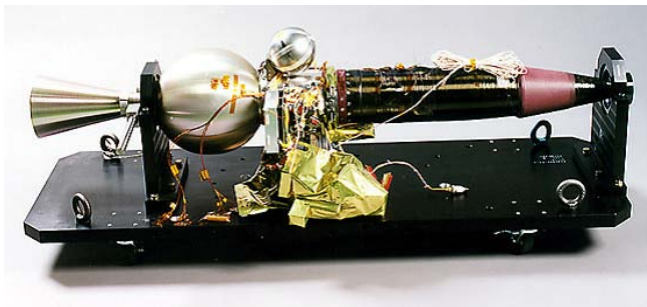
(a) Schematic of the LUNAR-A penetrator.
