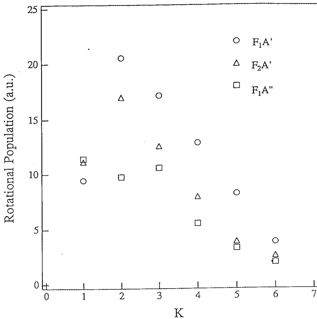
Fig.26. Nascent rotational state distribution of OH ( $v''=0$ ) for the reaction  $O(^3P)+H_2S$  under the bulk condition.
