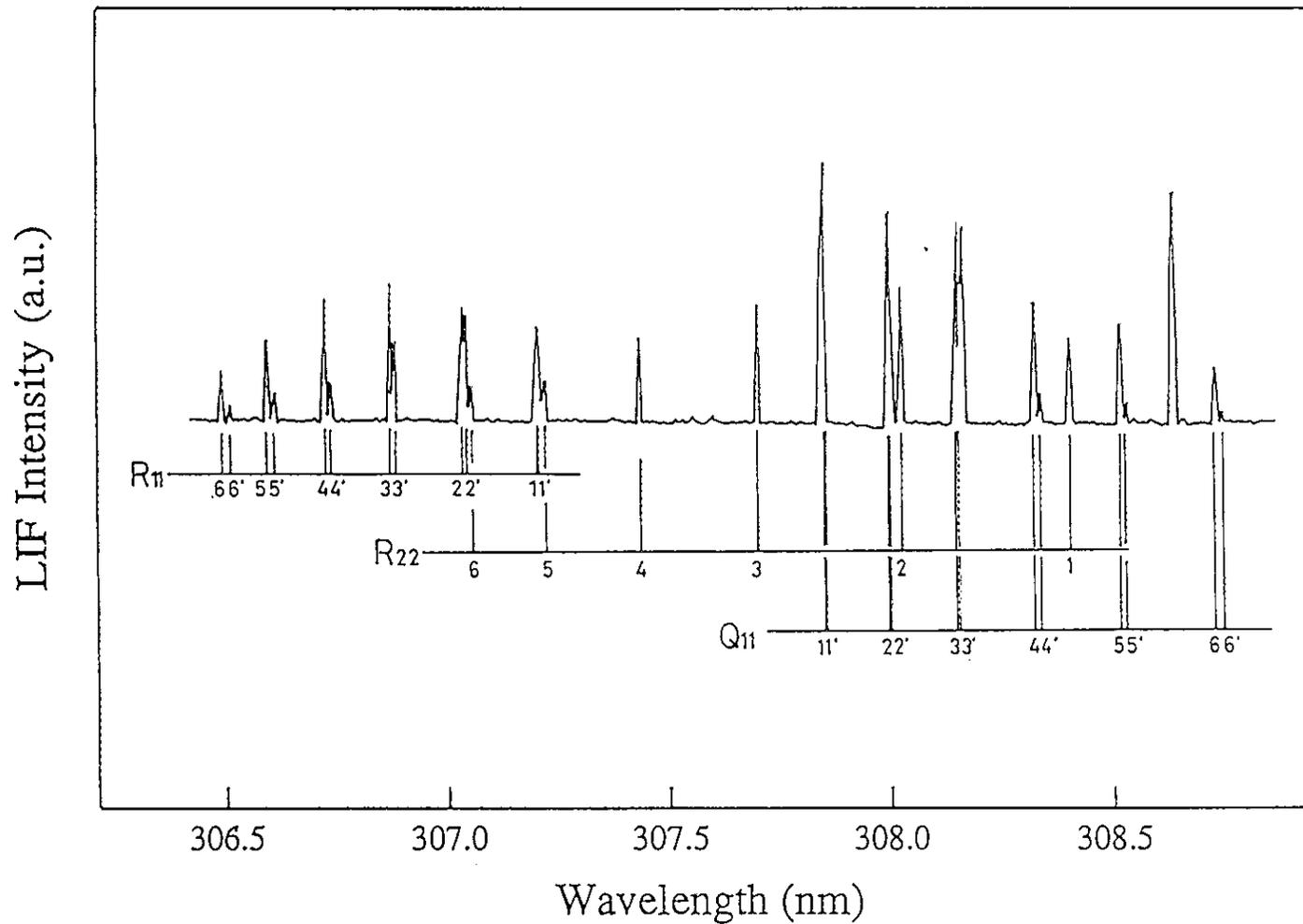
Fig.25. Part of the OH  $A^2\Sigma^+ - X^2\Pi$  ( $v''=0$ ) LIF excitation spectrum for  $O(^3P) + H_2S \rightarrow OH + HS$  under the bulk condition.
