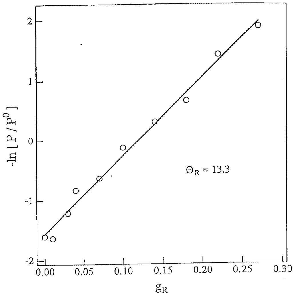
Fig.21(b). Suprisal plot of rotational distribution of OH( $v''=0$ ) for the reaction H+H<sub>2</sub>O under the bulk condition.
