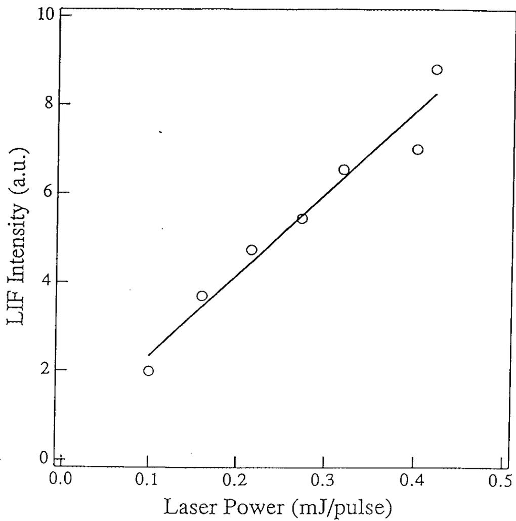
Fig.12. Laser power dependence of the LIF intensity of OH ( $X^2\Pi, v''=0$ ) for the reaction  $H+H_2O$  under the bulk condition. The data shown is for  $K=5$ .
