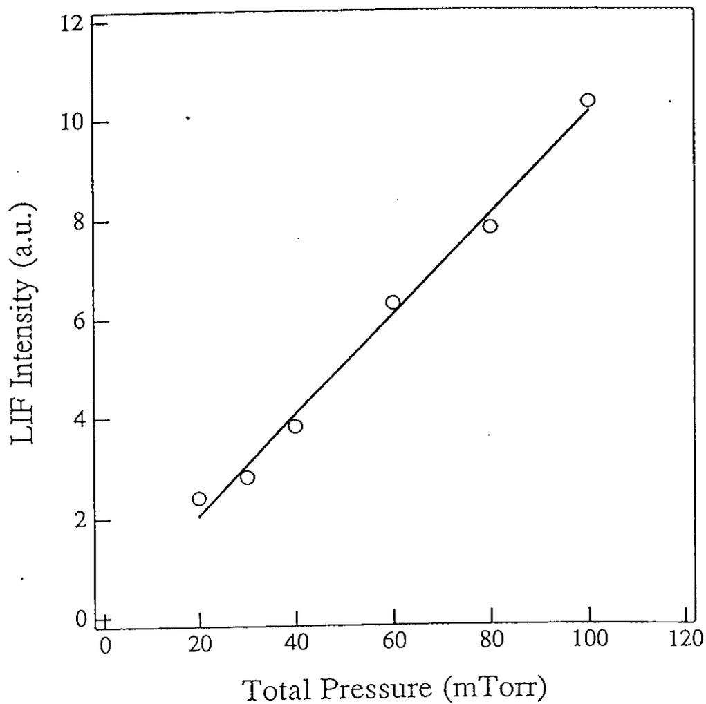
Fig. 9. Total gas pressure dependence of the LIF intensity of OH ( $X^2\Pi_{3/2}, v''=0$ ) for the reaction  $H+H_2O$  under the bulk condition.  $HI:H_2O=1:1$ . The data shown is for  $K=5$ .
