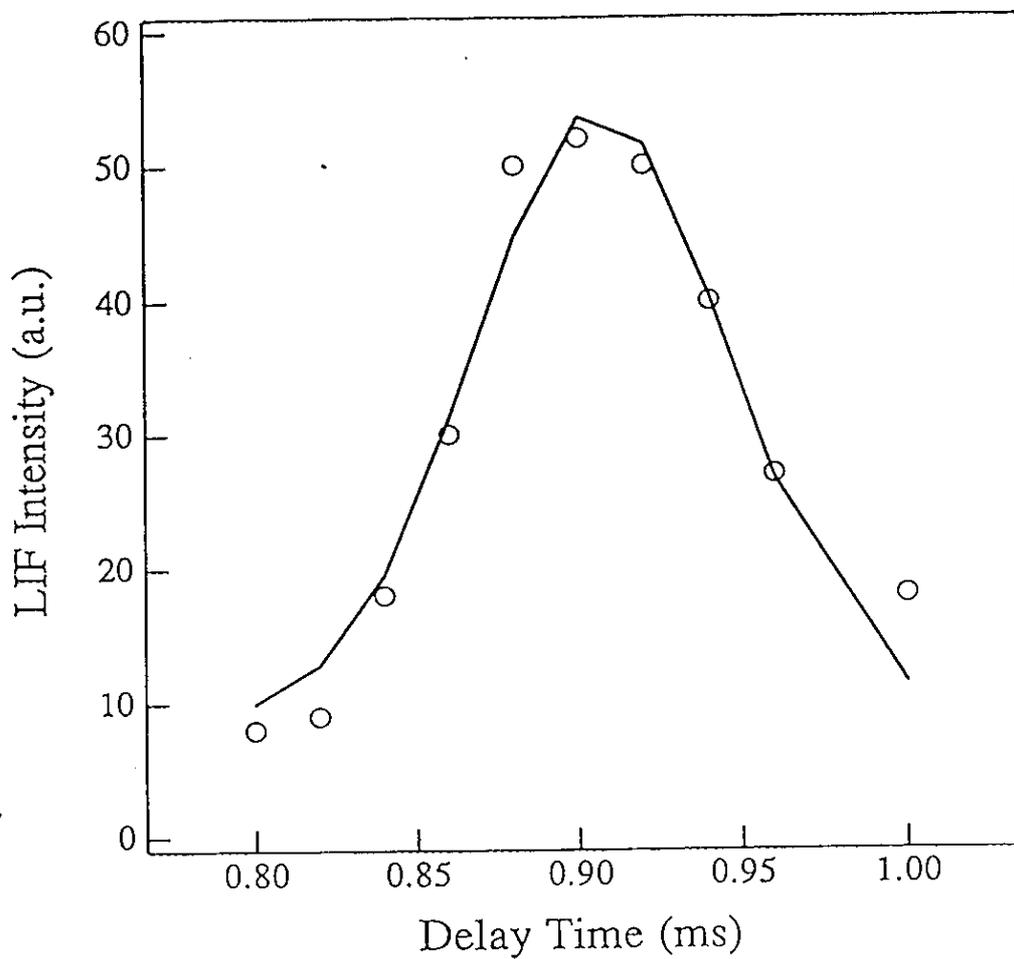
Fig.34. Injector-laser delay time dependence of the LIF intensity of  $\text{OH}(X^2\Pi_{3/2}, v''=0)$  for the reaction  $\text{HI} + \text{N}_2\text{O} \rightarrow \text{OH} + \text{N}_2 + \text{I}$  under the reactant-pair condition.
