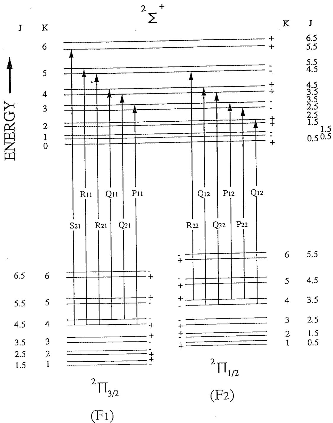
Fig. 7. Energy level diagram of OH radical.
