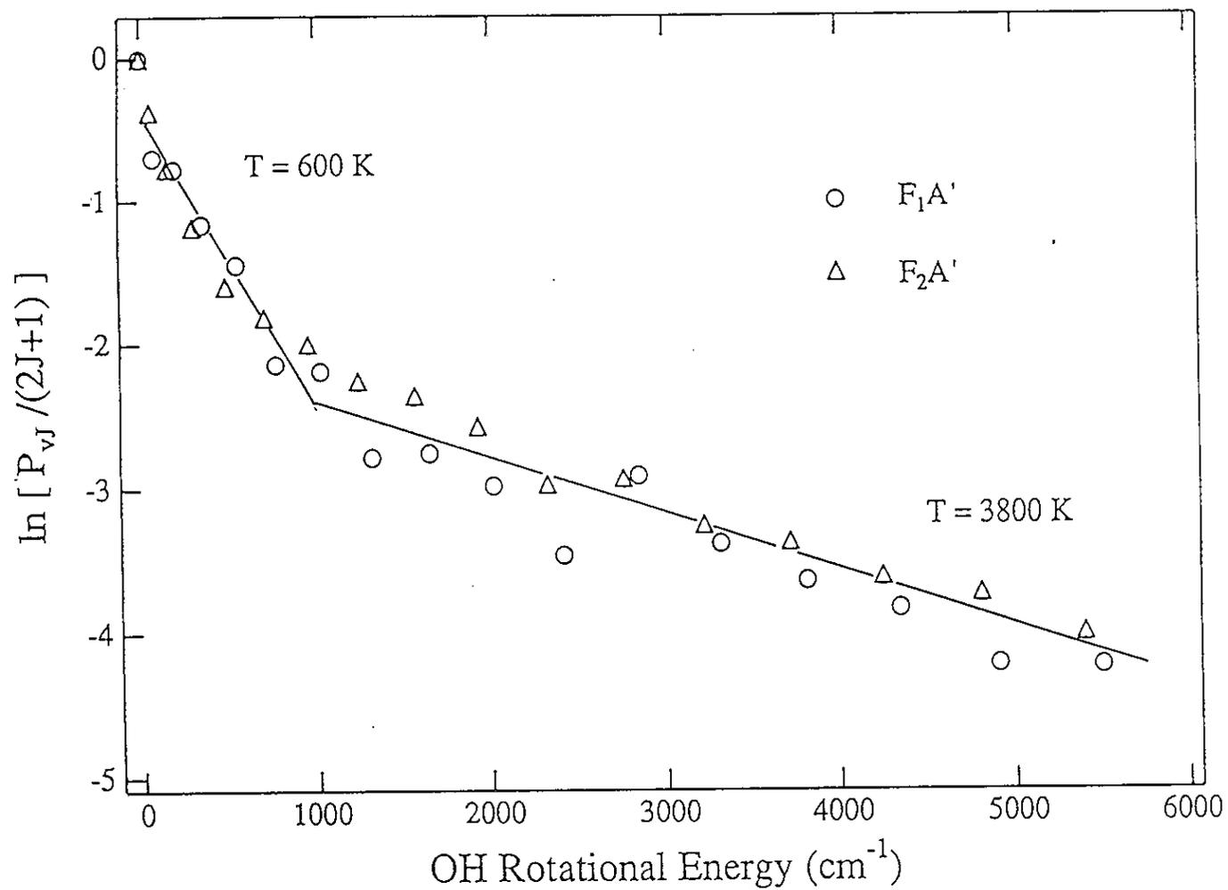
Fig.37. Boltzmann plot of the rotational distribution of  $\text{OH}(v''=0)$  for the reaction  $\text{HI}\cdot\text{N}_2\text{O} \rightarrow \text{OH} + \text{N}_2 + \text{I}$  under the reactant-pair condition.
