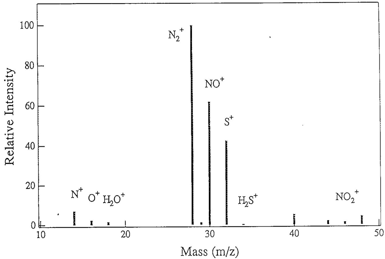
Fig.24. Mass spectrum of gas mixture of  $\text{NO}_2$  and  $\text{H}_2\text{S}$ .
