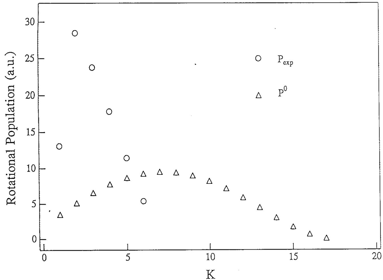
Fig.31(a). Comparison between experimental and calculated distributions of  $\text{OH}(v''=0)$  for the reaction  $\text{O}(^3\text{P})+\text{H}_2\text{S}$  under the bulk condition.
