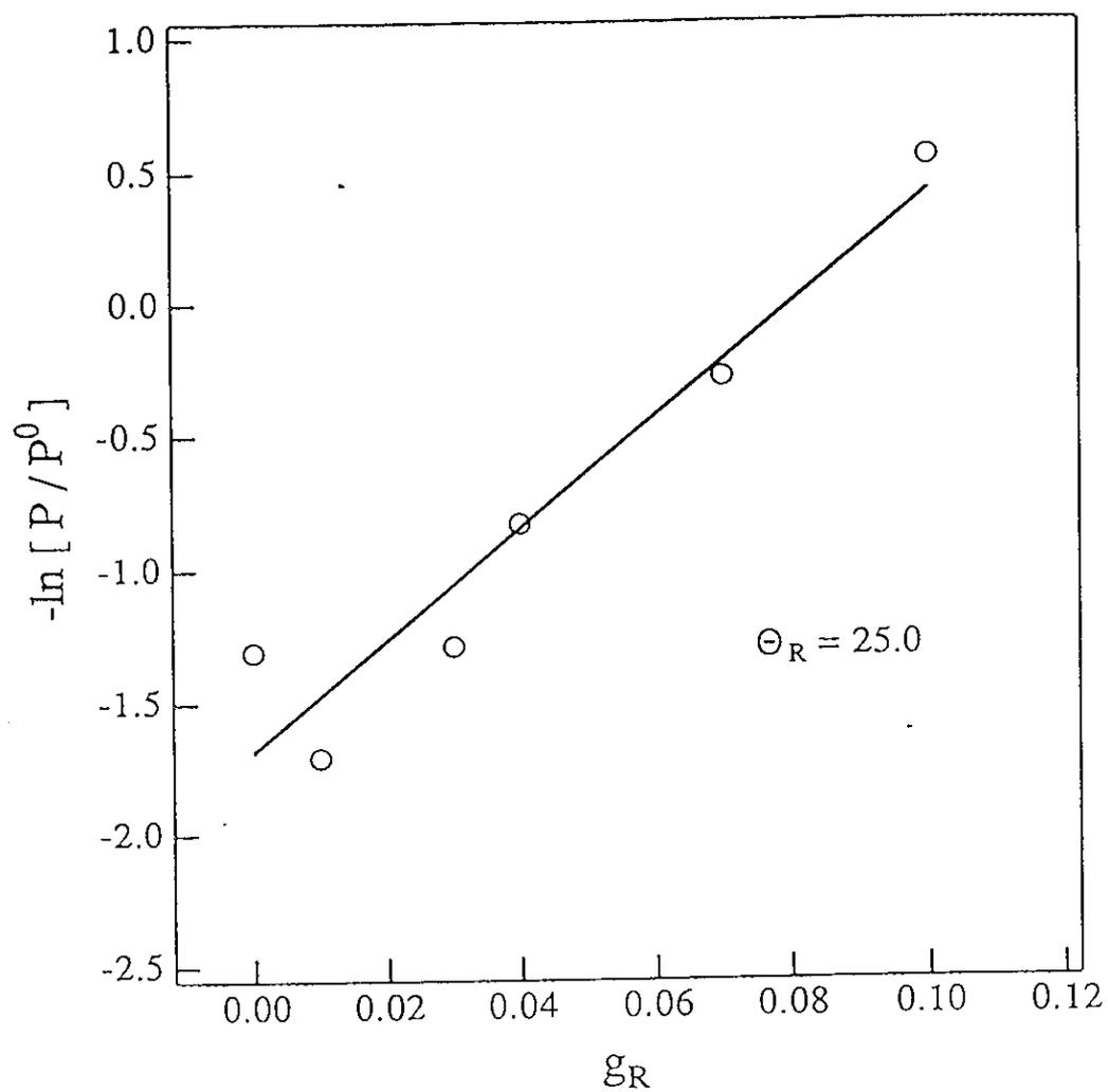
Fig.31(b). Surprisal plot of rotational distribution of OH( $v''=0$ ) for the reaction  $O(^3P)+H_2S$  under the bulk condition.
