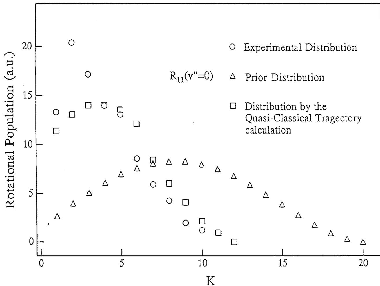
Fig.21(a). Comparison between experimental and calculated distributions of  $\text{OH}(v''=0)$  rotational states for the reaction  $\text{H}+\text{H}_2\text{O}$  under the bulk condition.
