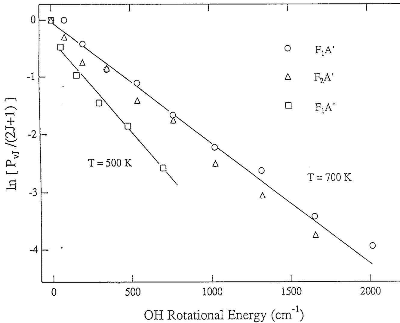
Fig.17. Boltzmann plot of the rotational distribution of  $\text{OH}(v''=0)$  for the reaction  $\text{H}+\text{H}_2\text{O}$  under the bulk condition.
