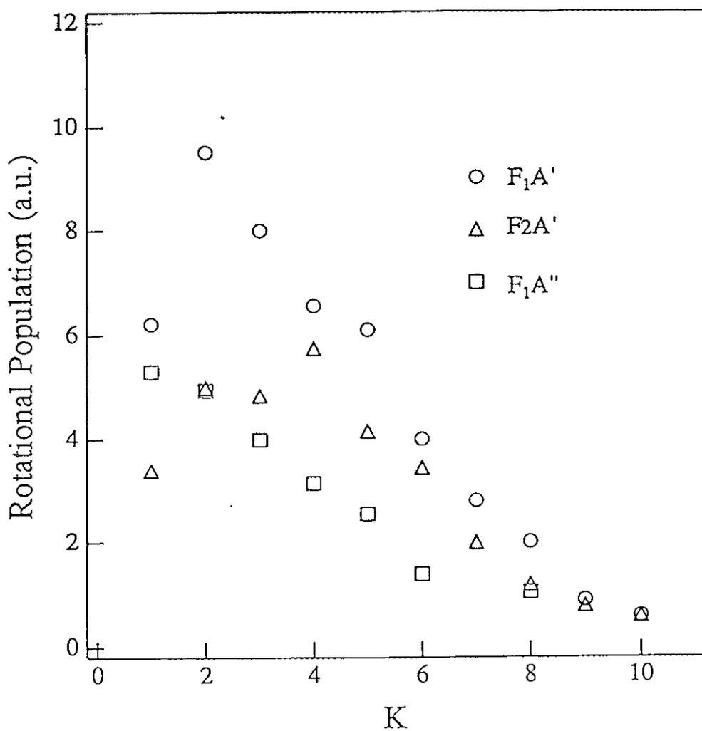
Fig.15. Nascent rotational-state distribution of OH( $v''=0$ ) for the reaction  $H+H_2O$  under the bulk condition.
