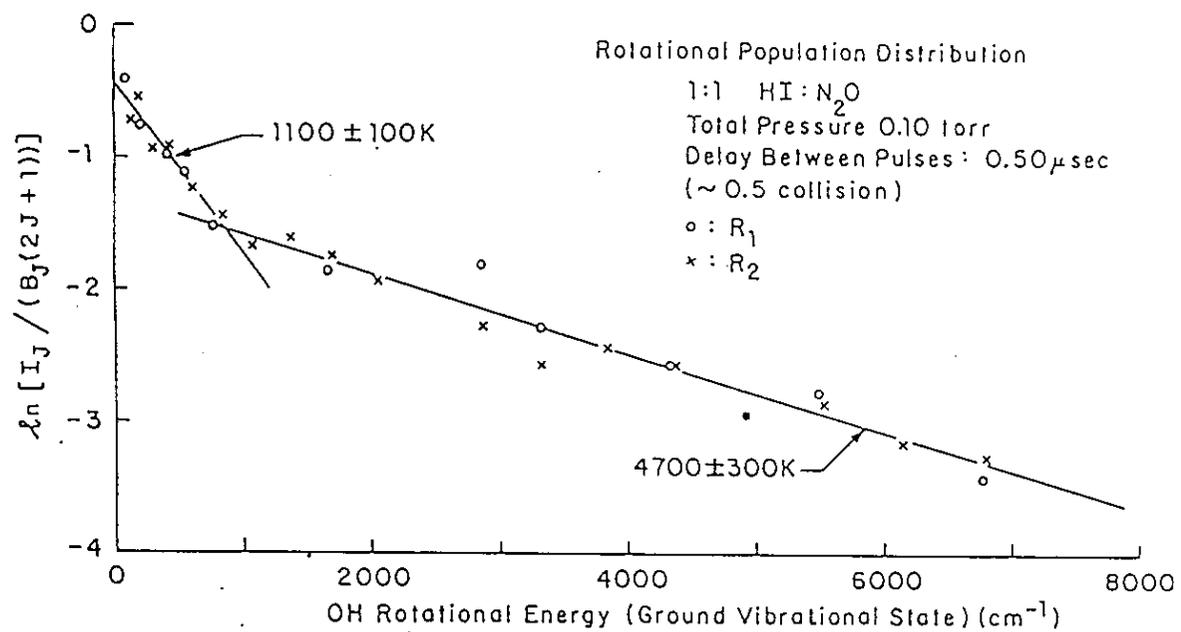
Fig.36. Boltzmann plot of the rotational distribution of OH( $v''=0$ ) for the reaction  $H+N_2O$  under the bulk condition.
