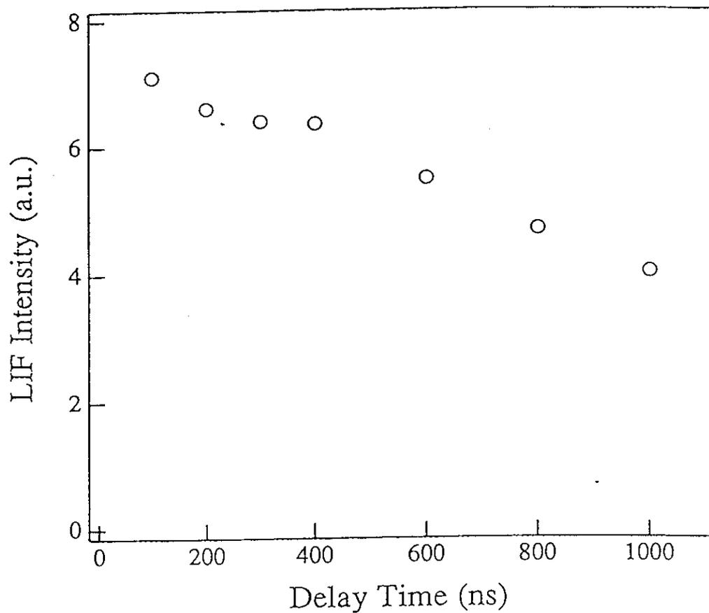
Fig.32. Delay time dependence of the LIF intensity of  $\text{OH}(X^2\Pi_{3/2}, v''=0)$  for the reaction  $\text{HI}\cdot\text{N}_2\text{O}\rightarrow\text{OH}+\text{N}_2+\text{I}$  under the reactant-pair condition.
