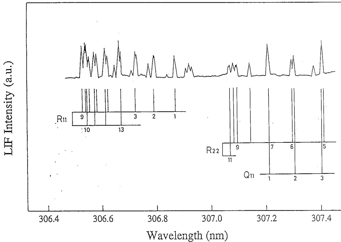
Fig.13(b). Part of the OD ( $v''=0$ ) LIF excitation spectrum for the reaction  $\text{H}+\text{D}_2\text{O}\rightarrow\text{OD}+\text{HD}$  under the same experimental condition as Fig.13(a).
