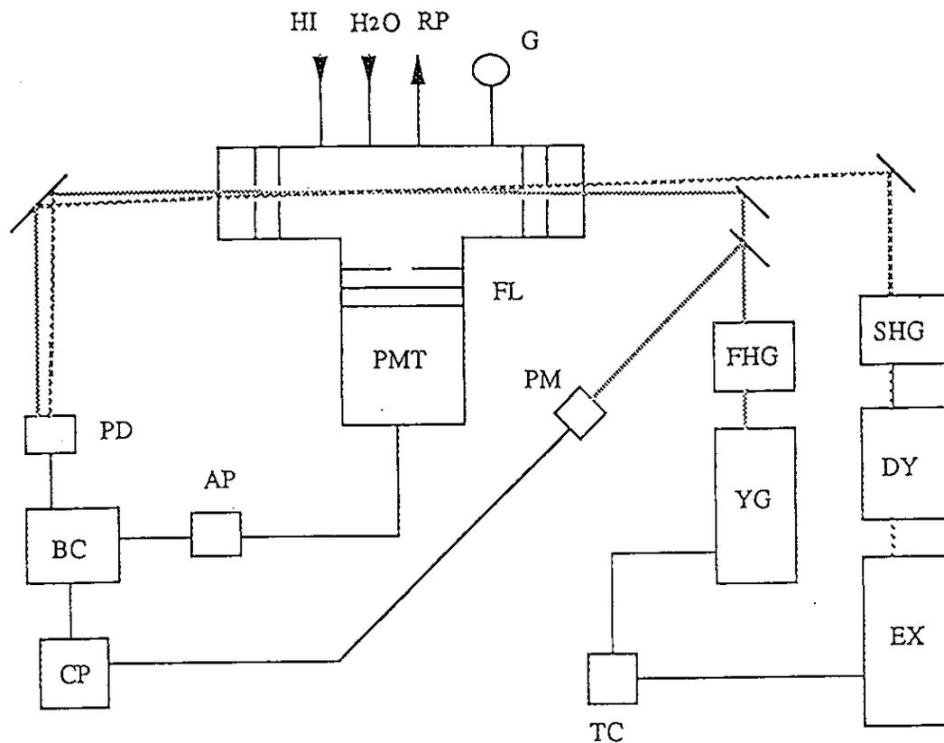
Fig. 4. Experimental setup for the bulk experiment.
