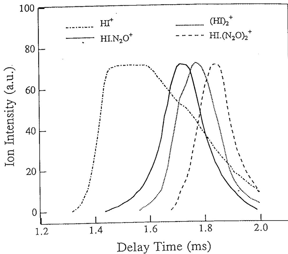
Fig.33. Time profile of  $(\text{HI})_N(\text{N}_2\text{O})_M$  clusters generated by the supersonic expansion at the stagnation pressure of 2.0 atm.
