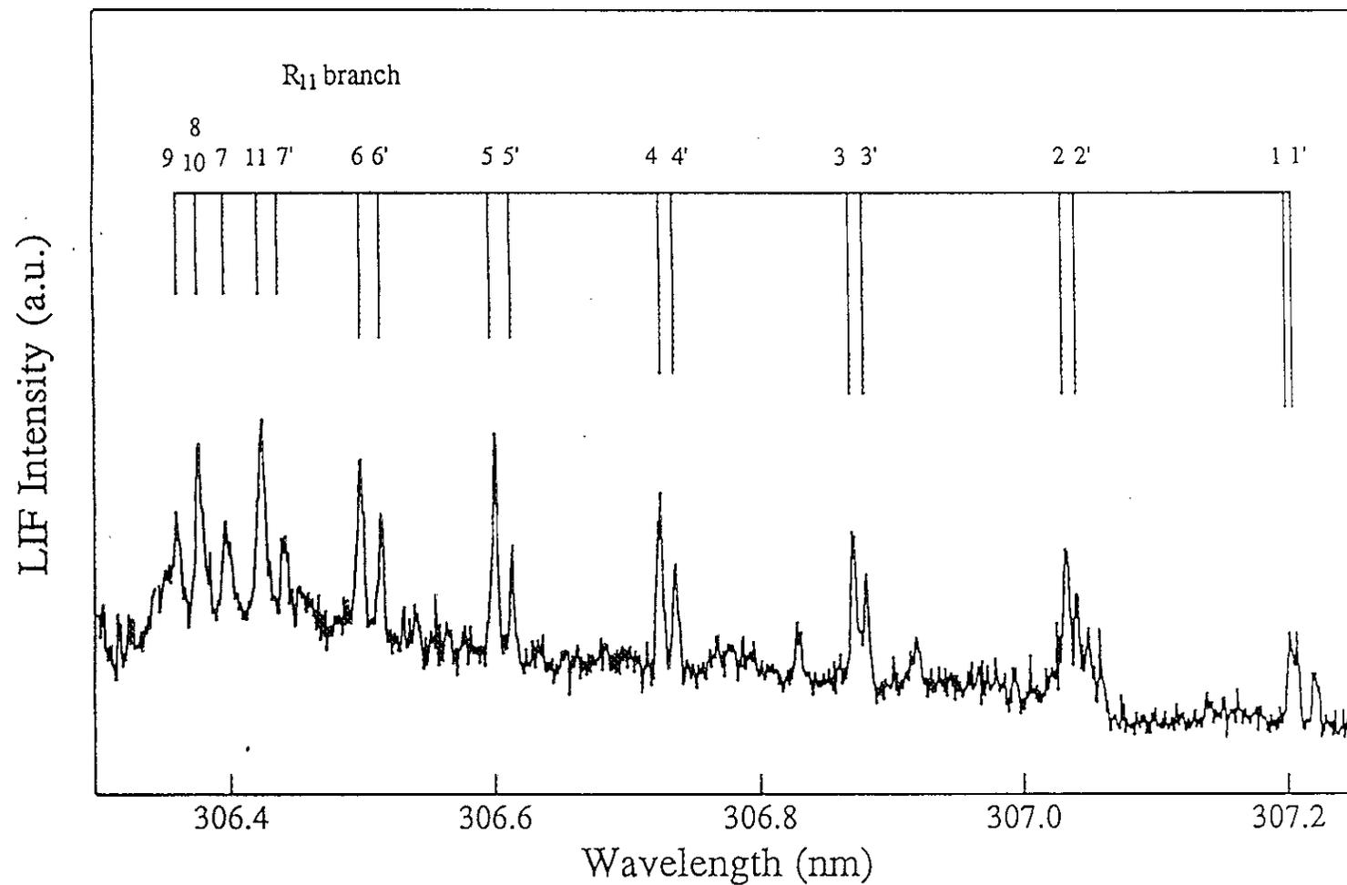
Fig.22. OH  $A^2\Sigma^+$  ( $v''=0$ ) LIF excitation spectrum for the reaction  $\text{HBr}\cdot\text{H}_2\text{O}\rightarrow\text{OH}+\text{H}_2+\text{Br}$  under the reactant-pair condition. (Stagnation pressure is 2.0 atm. Pump-probe delay time is 200 ns.  $\text{HBr}:\text{H}_2\text{O}:\text{He} = 2.6:0.9:96.5$ .)
