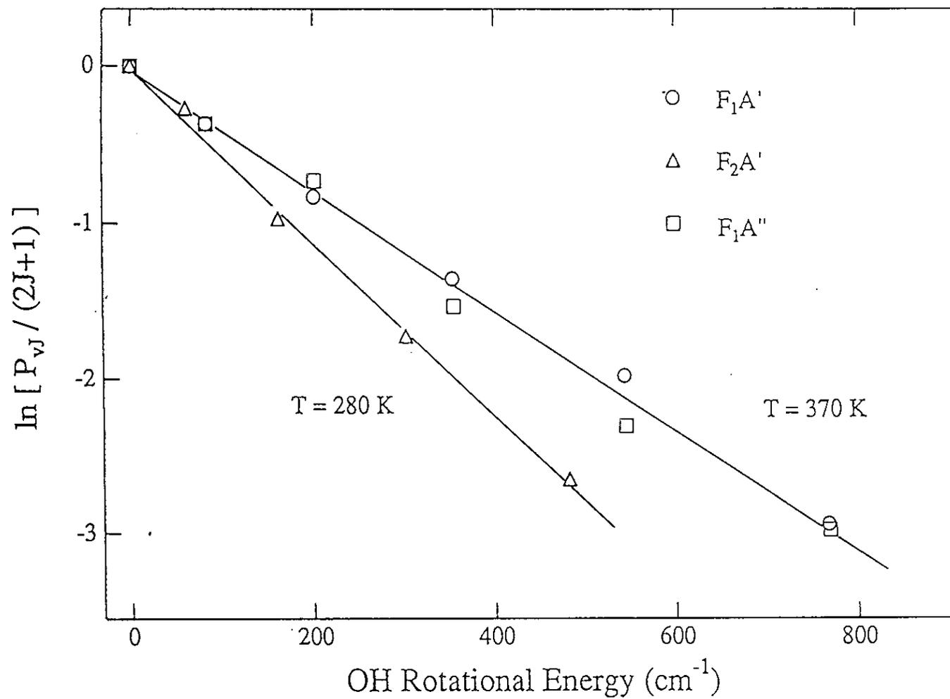
Fig.27. Boltzmann plot of the rotational distribution of  $\text{OH}(v''=0)$  for the  $\text{O}(^3\text{P})+\text{H}_2\text{S}$  reaction under the bulk condition.
