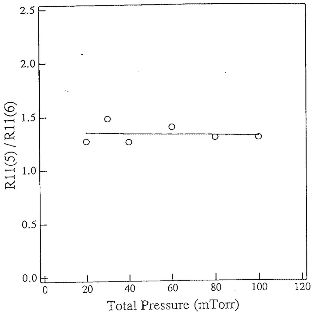
Fig.10. Total gas pressure dependence of ratio of the LIF intensities of OH ( $X^2\Pi_{3/2}, v''=0$ ) for the reaction  $H+H_2O$  under the bulk condition  $HI:H_2O=1:1$ .
