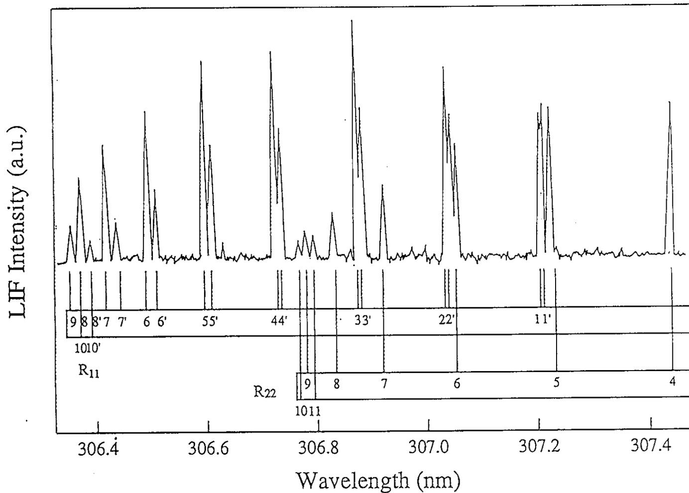
Fig.13(a). Part of the OH  $A^2\Sigma^+ - X^2\Pi$  ( $v''=0$ ) LIF excitation spectrum for the reaction  $\text{H} + \text{H}_2\text{O} \rightarrow \text{OH} + \text{H}_2$  under the bulk condition. (H atom is produced by the 266 nm photolysis of HI. Sample pressures of  $\text{H}_2\text{O}$  and HI are 30 mTorr. The delay time is 80 ns.)
