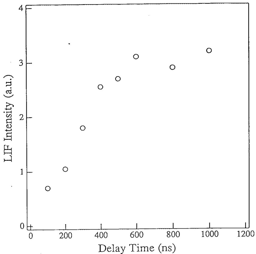
Fig.11. Pump-probe delay time dependence of the LIF intensity of OH ( $X^2\Pi_{3/2}, v''=0$ ) for the reaction  $H+H_2O$  under the bulk condition. The data shown is for  $K=5$ .
