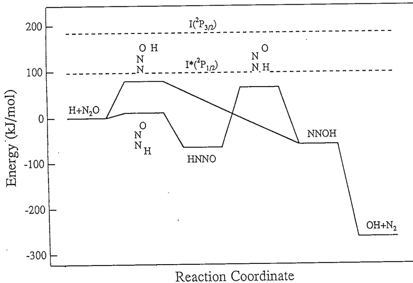
Fig.2. Potential energy diagram for the reaction  $\text{H} + \text{N}_2\text{O} \rightarrow \text{OH} + \text{N}_2$ .
