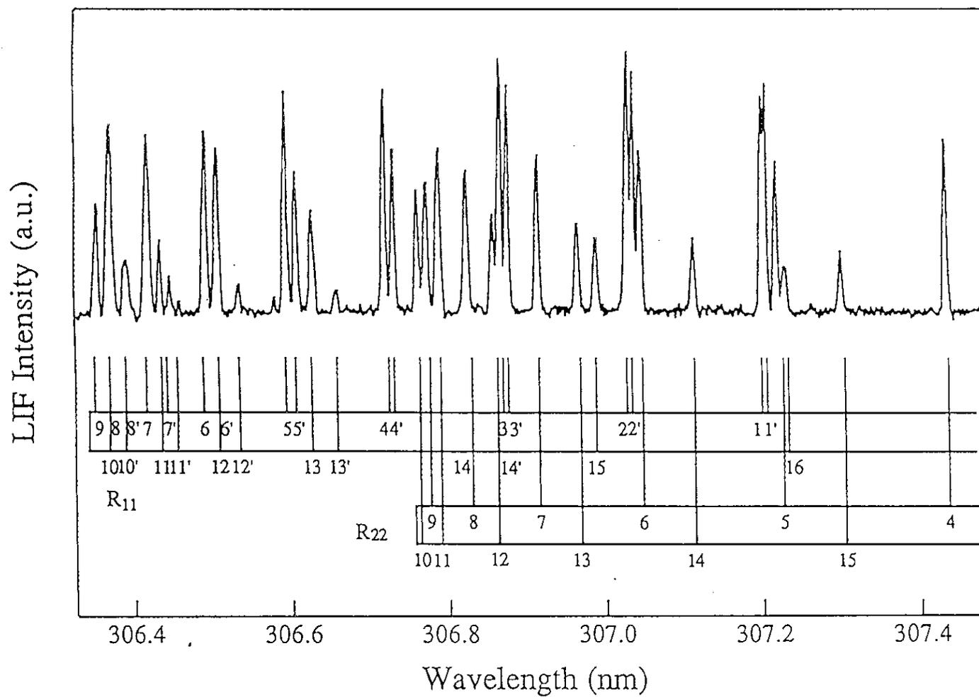
Fig.35. Part of the OH  $A^2\Sigma^+ - X^2\Pi$  ( $v''=0$ ) LIF excitation spectrum for the reaction  $HI \cdot N_2O \rightarrow OH + N_2 + I$  under the reactant-pair condition. (Stagnation pressure is 2.5 atm. Pump-probe delay time is 200 ns.  $HI:N_2O:He = 2.6:4.4:93.$ )
