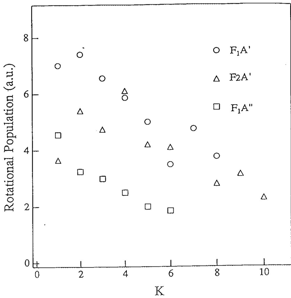
Fig.16. Nascent rotational-state distribution of OD(v''=0) for the reaction H+D<sub>2</sub>O under the bulk condition.
