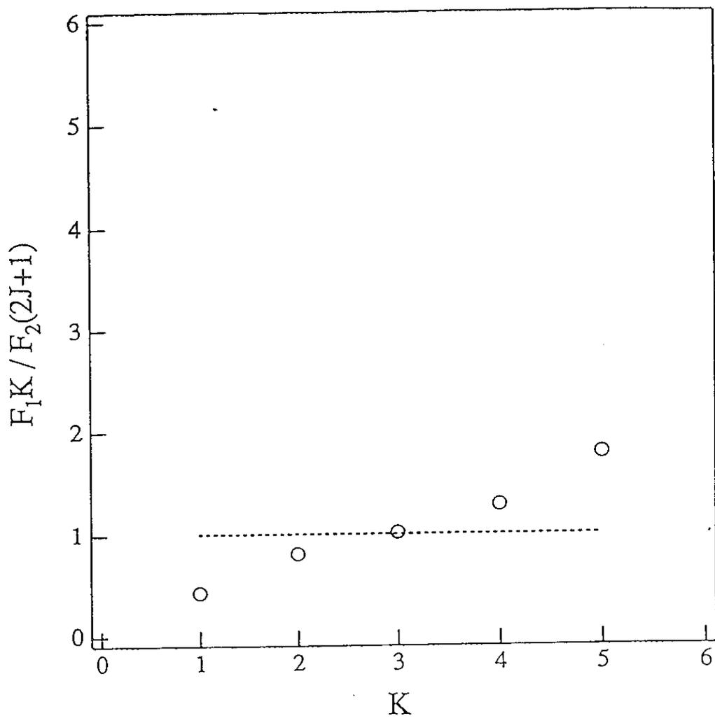
Fig.28. K dependence of spin-orbit population ratios of OH for the reaction  $O(^3P)+H_2S$  under the bulk condition.
