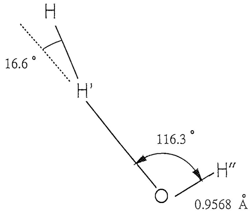
Fig.18. Transition-state geometry for the reaction  $\text{H} + \text{H}_2\text{O}$ .
