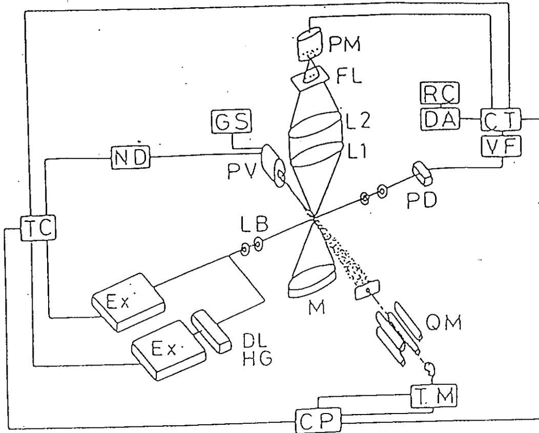
Fig. 5. Experimental setup for the free jet experiment.
