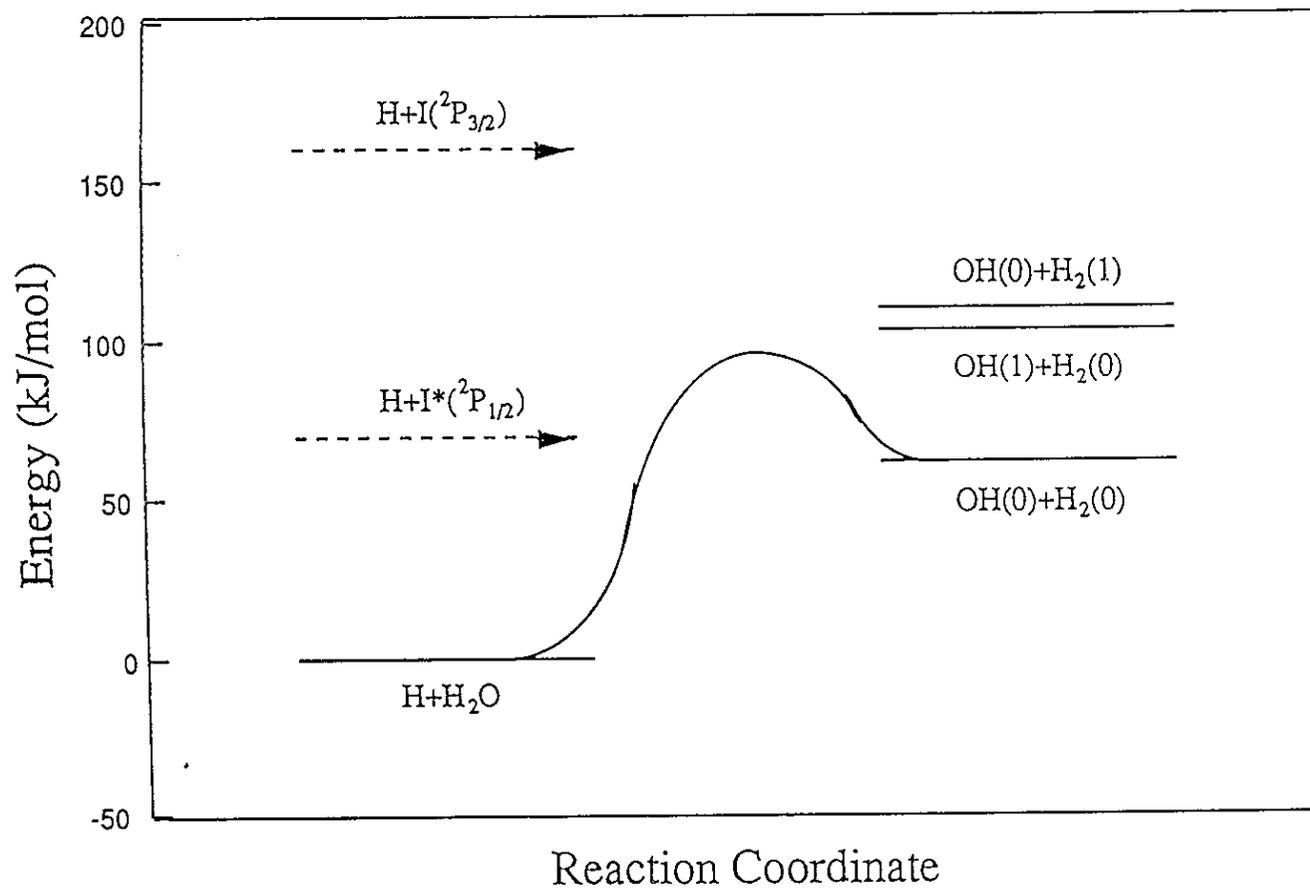
Fig. 8. Potential energy diagram for the reaction  $H+H_2O \rightarrow OH+H_2$ .
