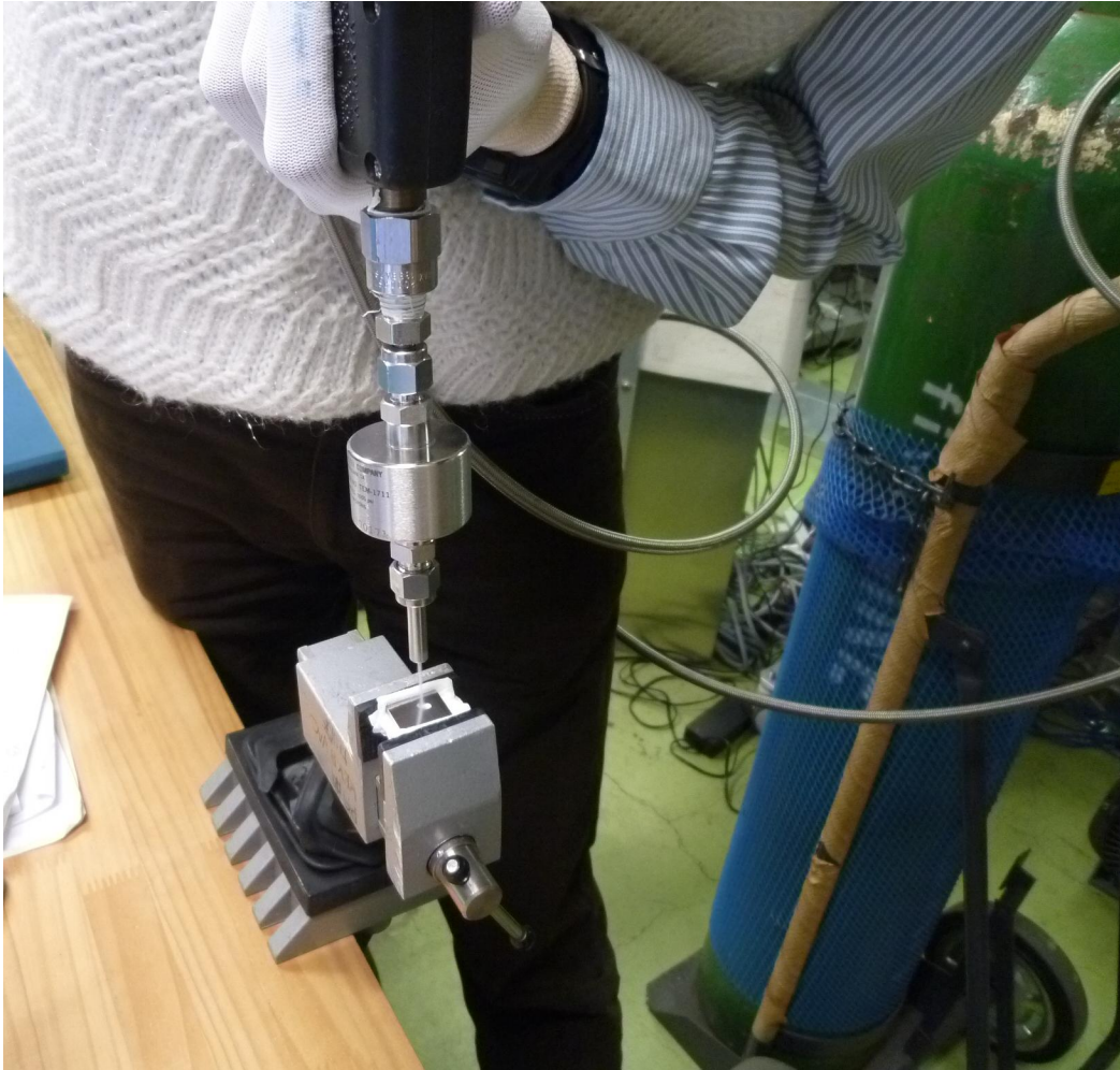
Fig. 3.7 : The dry ice cleaning of the Nb sample in air.
