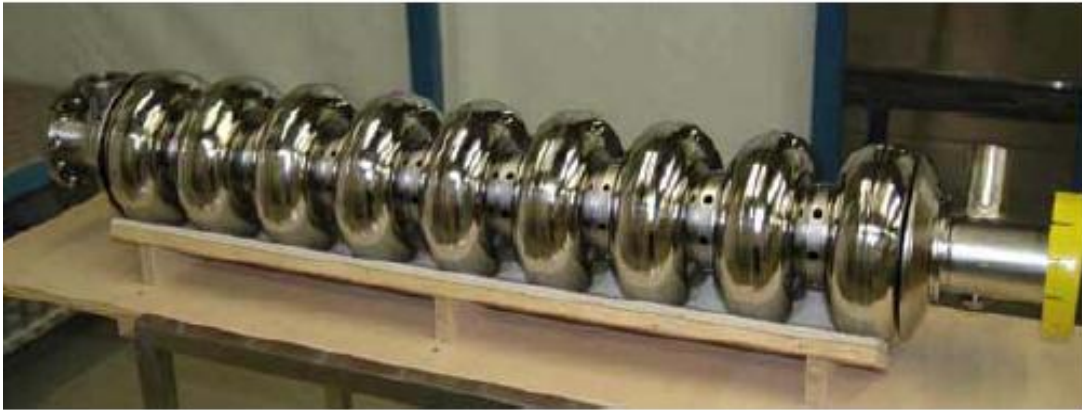
Fig. 1.9 : (a) Welded cavity parts. (b) Nine-cell cavity after welding [1.8].
