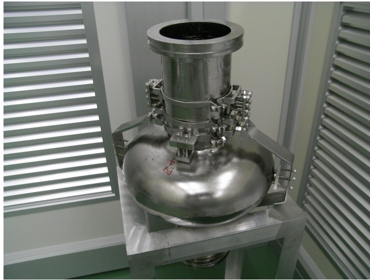
Fig. 3.3 : The cavity assembled with six Nb disc type samples.
