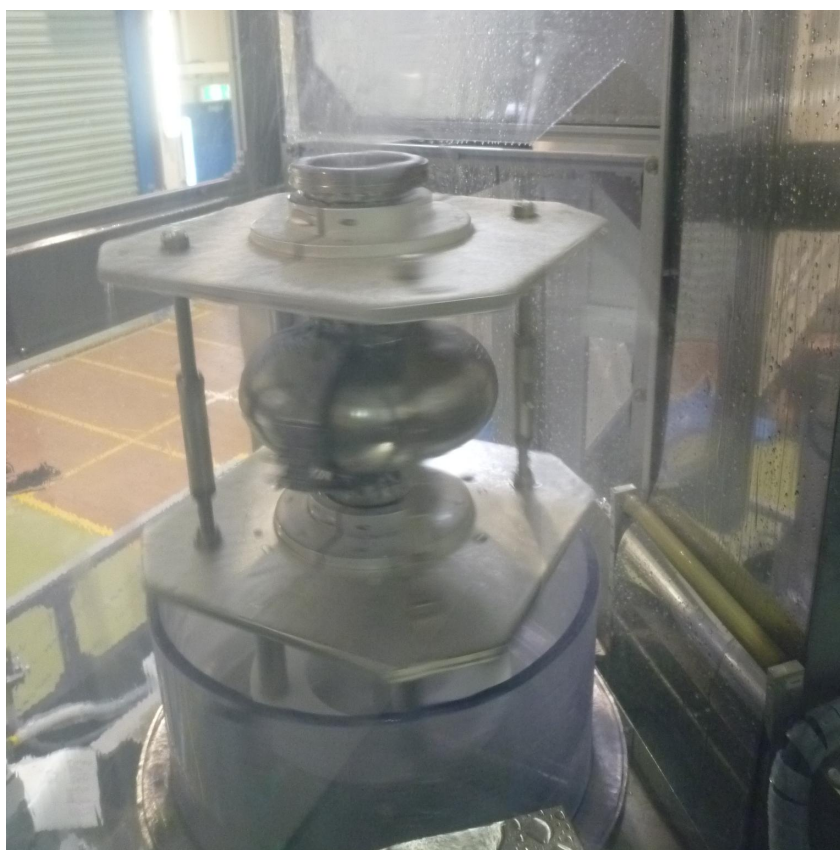
Fig. 3.6 : The Nb cavity assembled with Nb disc type samples during the cavity HPR experiment.
