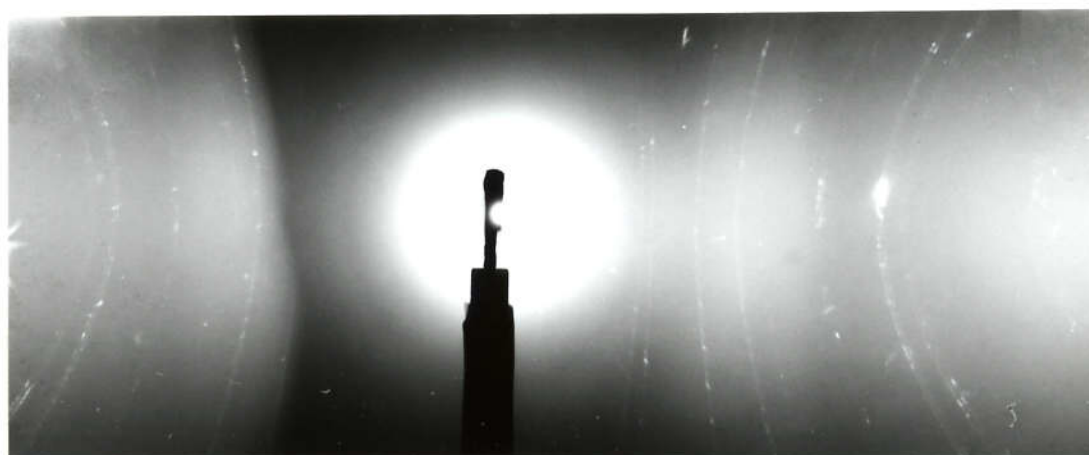
Fig.3.8. X-ray diffraction pattern of a C 60 (TDAE) crystal of 0.2 mm length by an oscillation-camera method at the vibration angle of 10° with respect to the long axis.
