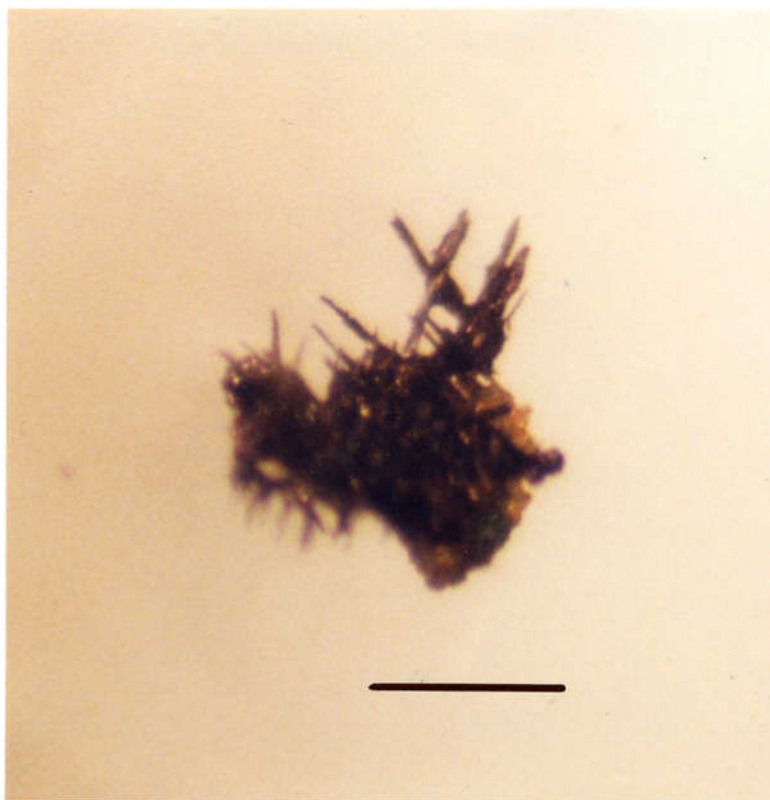
Fig.3.7. The morphology of C 60 (TDAE) conglomeration of crystals observed under an optical microscope. scale bar=0.3 mm
