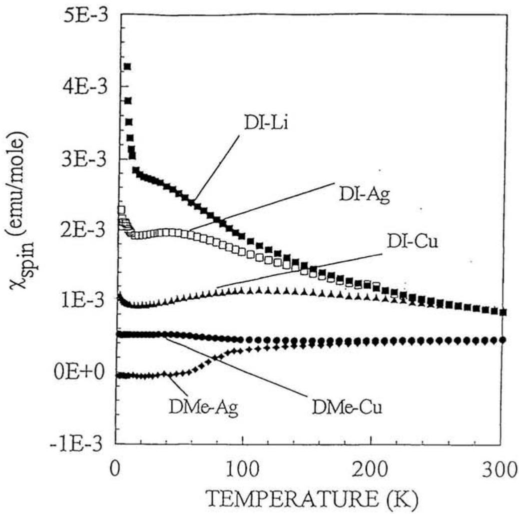
Fig 3-3-2 Temperature dependence of spin susceptibility.
