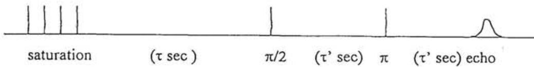
Fig. 2-2-3a) The typical pulse sequence.
