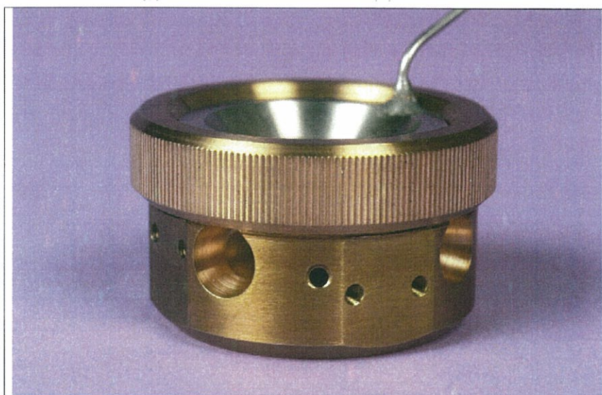
Plate 1: The WCM7B cryogenic cell showing a general view with the gas membrane inlet tube to the top right. The WCM7 cell is made of stainless steel but is otherwise identical.
