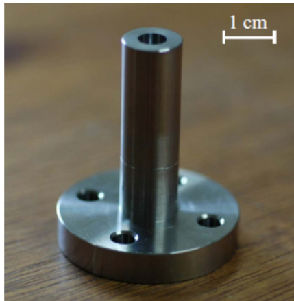
Fig. 2.9 Image of Laval nozzle with 0.3 mm throat diameter.
