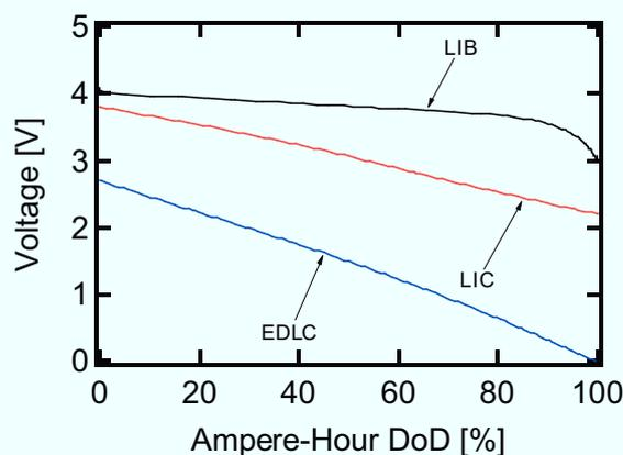
Fig. 2.4.2. Typical discharge curves of LIB, EDLC, and LIC cells.
