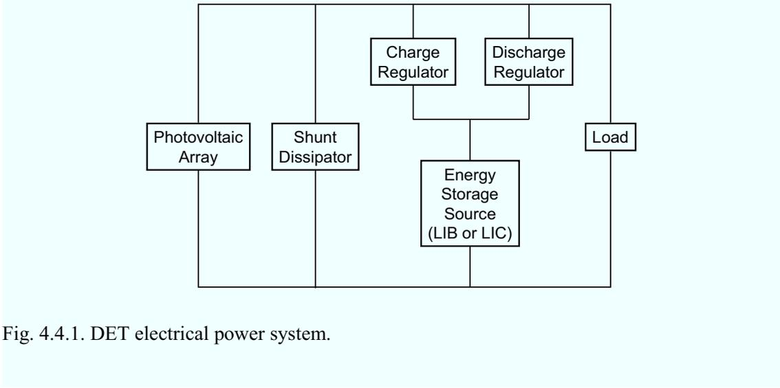
Fig. 4.4.1. DET electrical power system.
