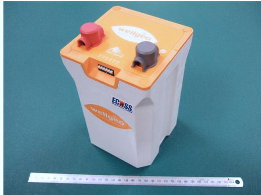
Fig. 6.4.8. A photograph of an EDLC module.
