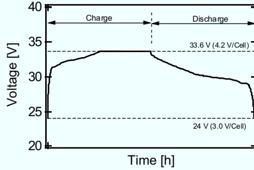
Fig. 7.3.3. Typical charge–discharge profile of a lithium-ion battery consisting of eight cells in series.
