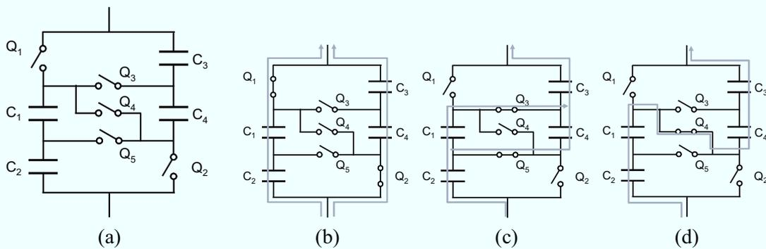
Fig. 7.2.2. Series-parallel changeover circuit. (a) Circuit description, (b) 2-series 2-parallel configuration, (c) 3-series 1- or 2-parallel configuration, and (d) 4-series 1-parallel configuration.
