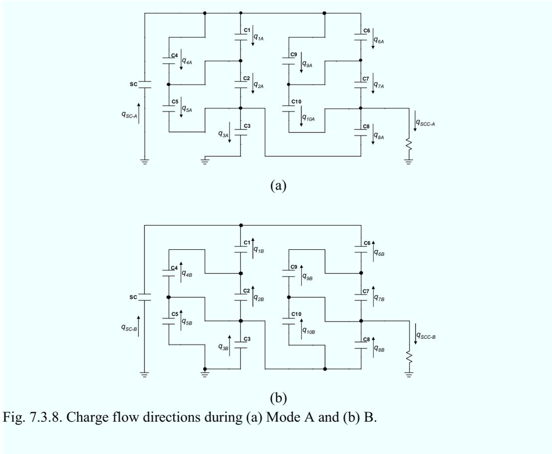
Fig. 7.3.8. Charge flow directions during (a) Mode A and (b) B.
