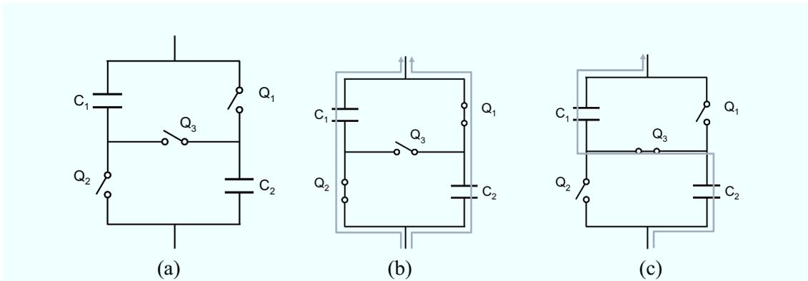
Fig. 7.2.1. Series-parallel changeover circuit. (a) Circuit description, (b) 1-series 2-parallel configuration, and (c) 2-series 1-parallel configuration.
