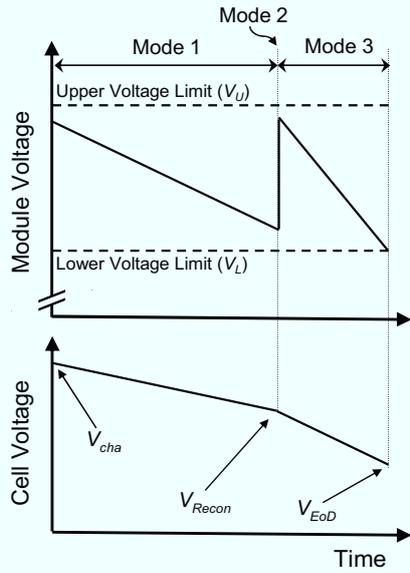
Fig. 7.4.3. Module and cell voltage curves during constant current discharging.
