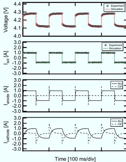
Fig. 5.4.11. Experimental and simulation waveforms of cell voltage,  $I_{sol}$ ,  $I_{anode}$ , and  $I_{cathode}$  at a cycle frequency of 10 Hz.
