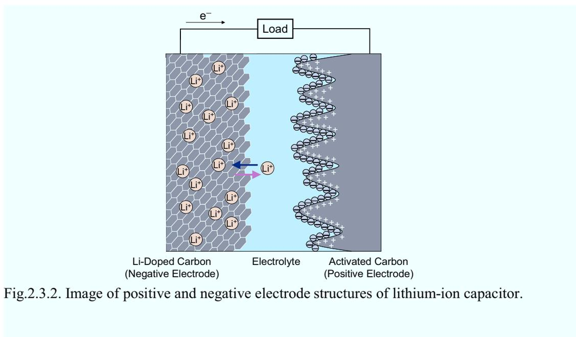
Fig.2.3.2. Image of positive and negative electrode structures of lithium-ion capacitor.
