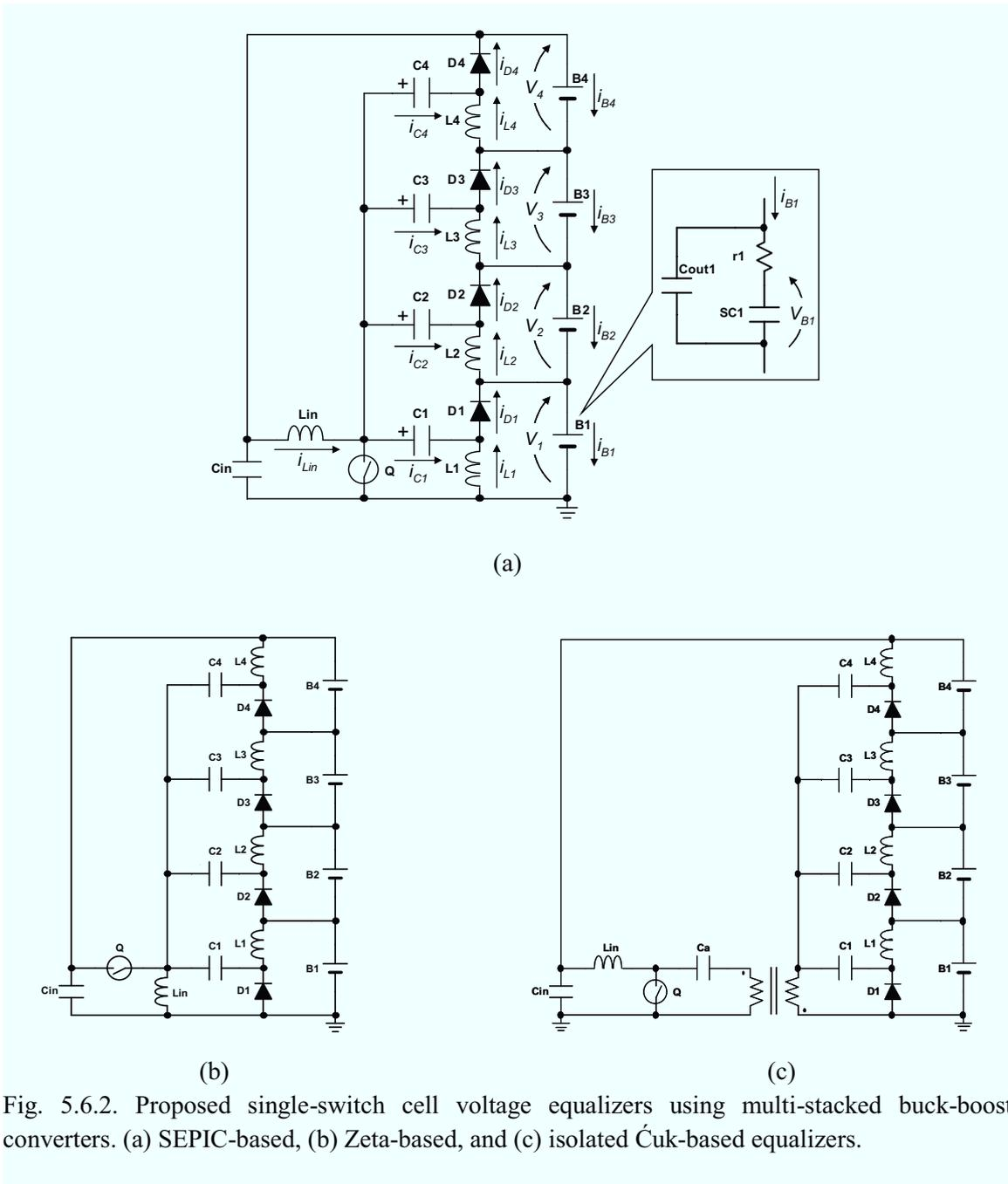
Fig. 5.6.2. Proposed single-switch cell voltage equalizers using multi-stacked buck-boost converters. (a) SEPIC-based, (b) Zeta-based, and (c) isolated Ćuk-based equalizers.
