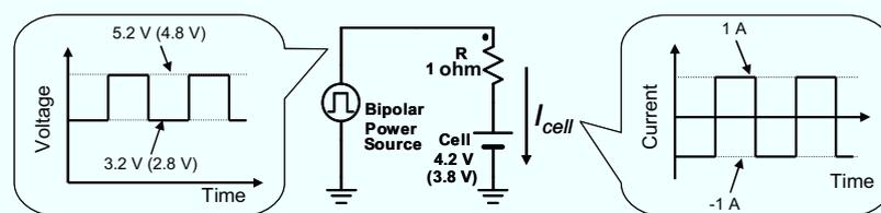
Fig. 5.4.5. Experimental setup and charge-discharge profiles for high-frequency cycling tests.
