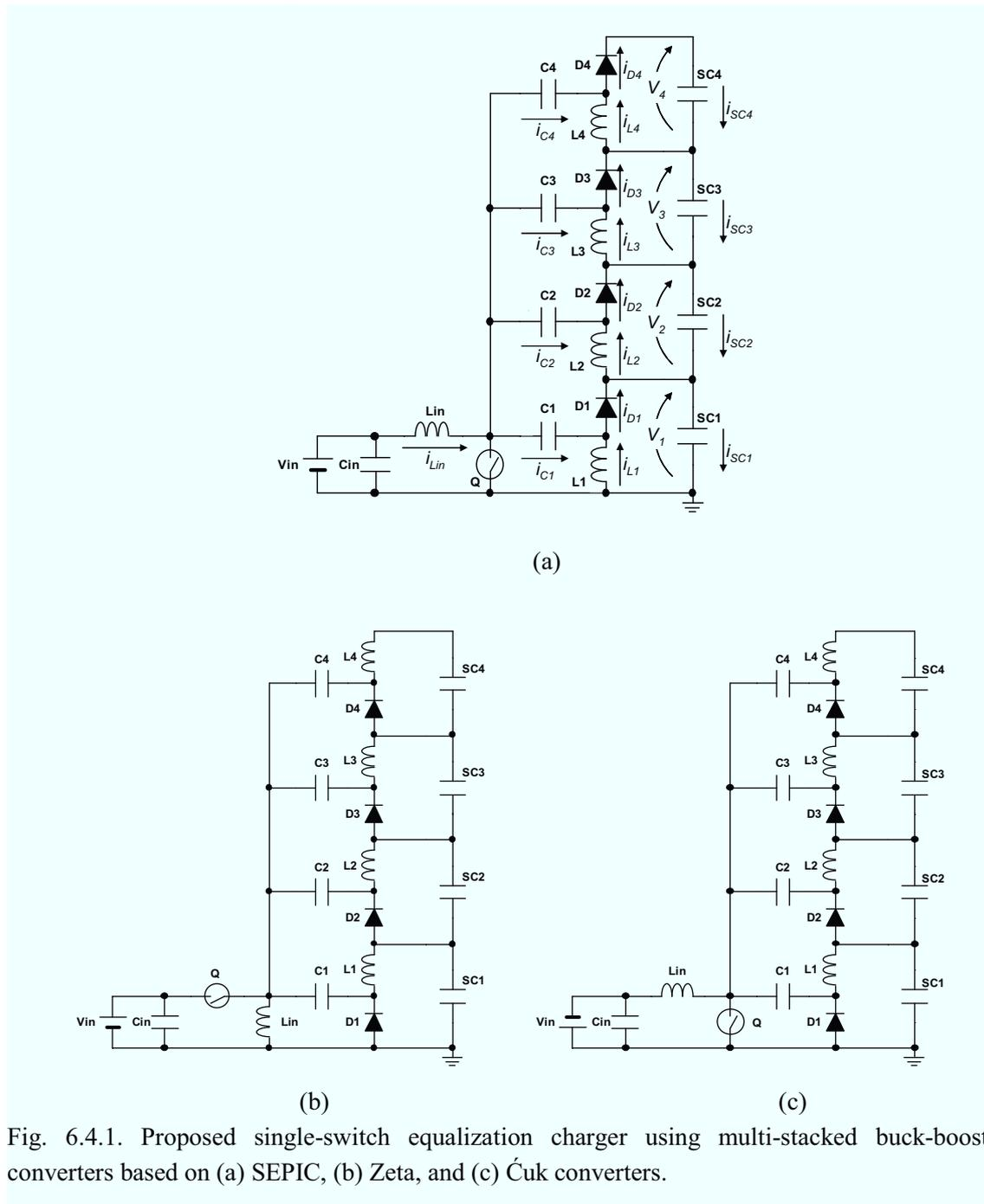
Fig. 6.4.1. Proposed single-switch equalization charger using multi-stacked buck-boost converters based on (a) SEPIC, (b) Zeta, and (c) Ćuk converters.
