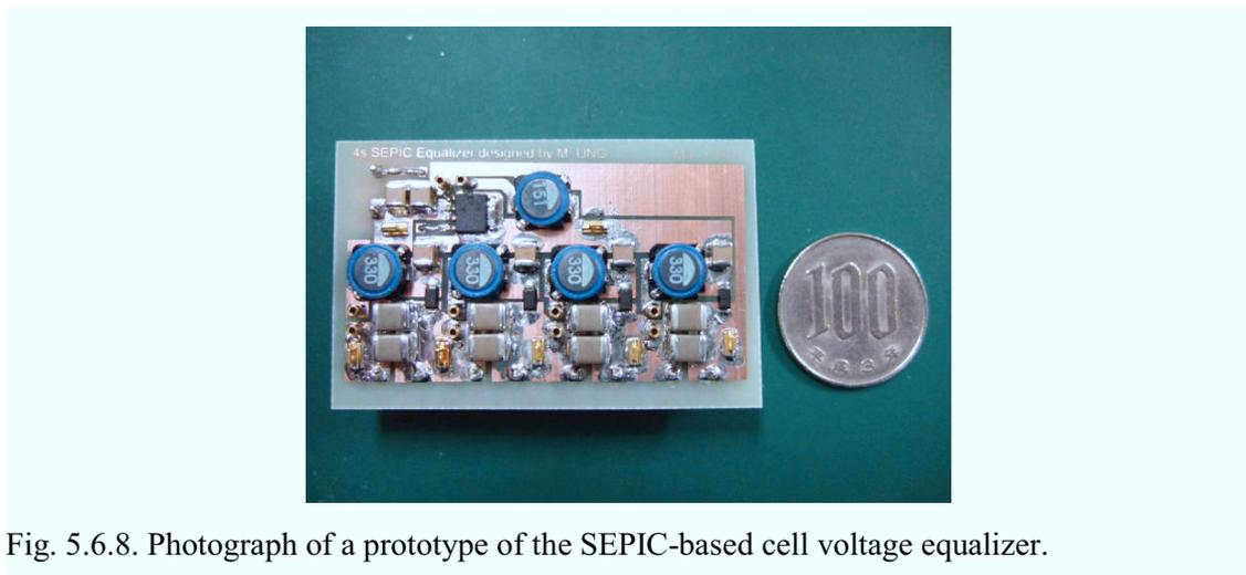
Fig. 5.6.8. Photograph of a prototype of the SEPIC-based cell voltage equalizer.
