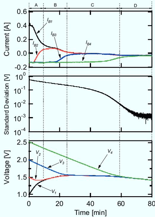
Fig. 5.6.9. Experimental equalization profiles of series-connected SCs whose initial voltages,  $V_{B1}-V_{B4}$ , were 1.0, 1.5, 2.0, and 2.5 V, respectively.
