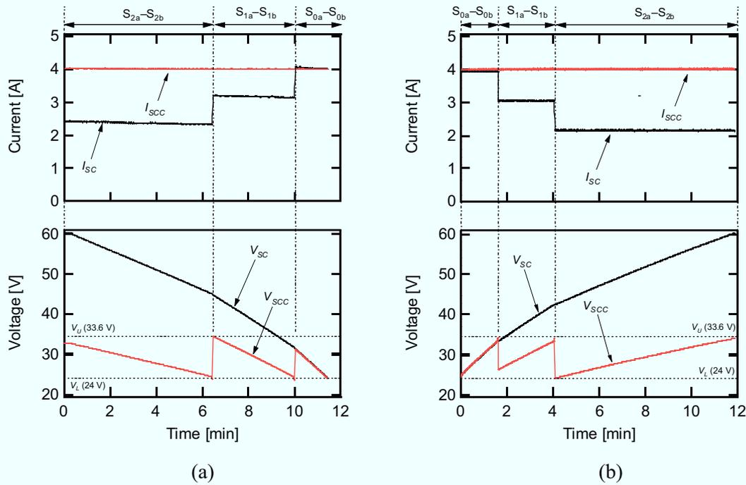
Fig. 7.3.12. Experimental (a) discharge and (b) charge curves of the EDLC module with the proposed unregulated interface converter.
