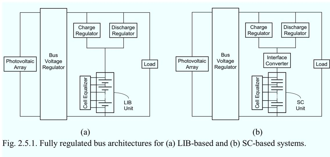
Fig. 2.5.1. Fully regulated bus architectures for (a) LIB-based and (b) SC-based systems.
