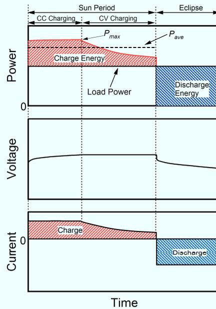
Fig. 4.3.3. Typical profiles of a LIB and PV power during LEO-emulated charge-discharge cycling.
