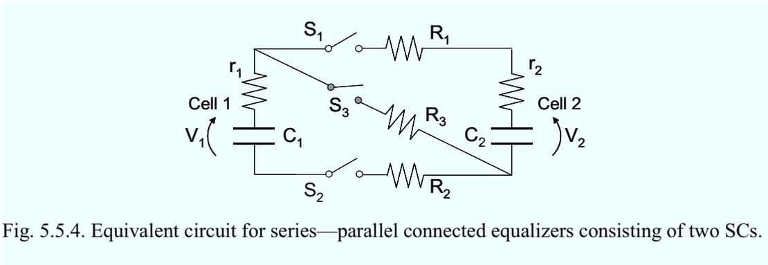
Fig. 5.5.4. Equivalent circuit for series-parallel connected equalizers consisting of two SCs.
