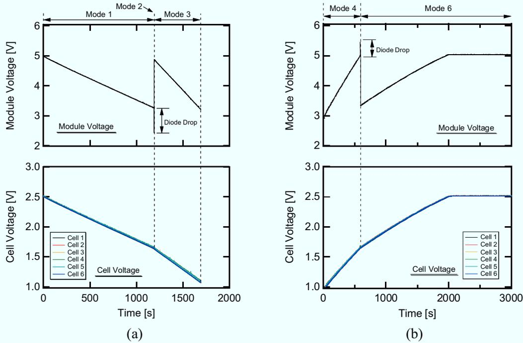
Fig. 7.4.5. Module and cell voltage curves during (a) discharging and (b) charging.
