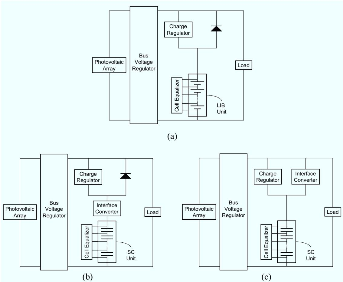
Fig. 2.5.2. Sun-regulated bus architectures for (a) LIB-based system and SC-based systems using unregulated interface converter (b) with discharge diode and (c) without discharge diode.
