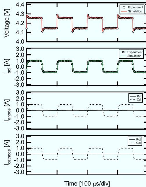
Fig. 5.4.10. Experimental and simulation waveforms of cell voltage,  $I_{sol}$ ,  $I_{anode}$ , and  $I_{cathode}$  at a cycle frequency of 10 kHz.
