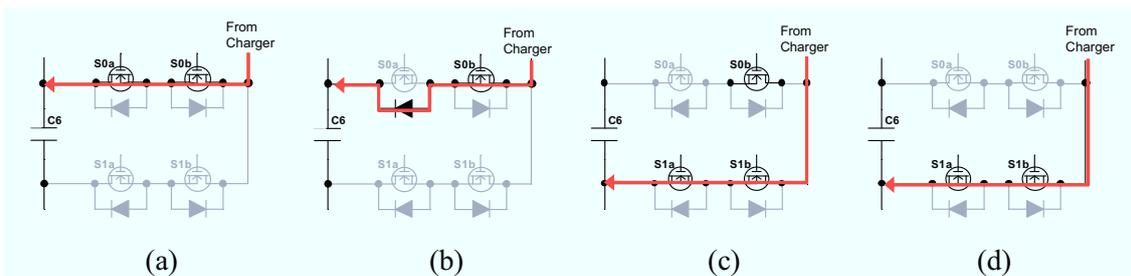
Fig. 7.3.7. Switching sequence of selectable intermediate taps for charging.
