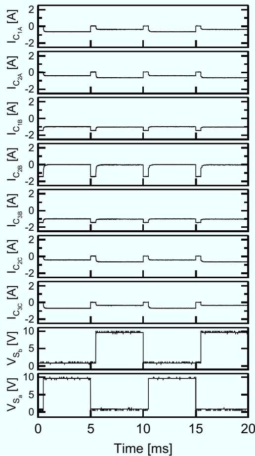
Fig. 5.5.7. Current waveforms of the cells and drive voltages for  $S_a$  and  $S_b$  during discharging.
