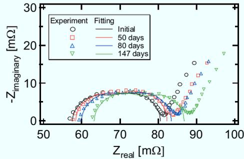
Fig. 5.4.9. Trend of measured Nyquist plots and fitting curves of the cell cycled at 1 Hz.
