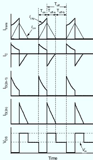
Fig. 5.7.2. Key waveforms in DCM under the cell voltage-balanced condition.
