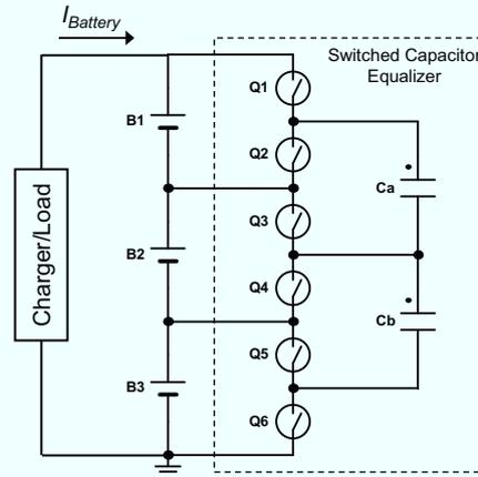
Fig. 5.4.2. Switched capacitor equalizer for a battery pack consisting of three cells connected in series.
