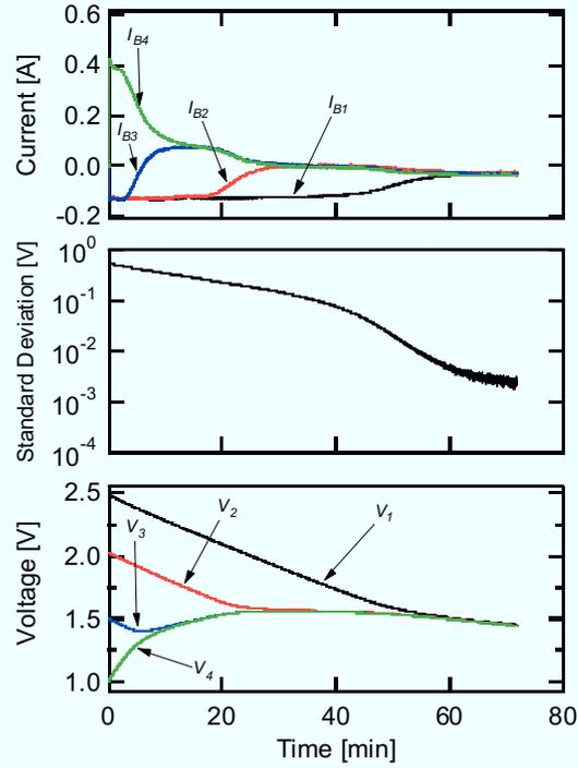
Fig. 5.6.11. Experimental equalization profiles of series-connected SCs whose initial voltages,  $V_{B1}-V_{B4}$ , were 2.5, 2.0, 1.5, and 1.0 V, respectively.
