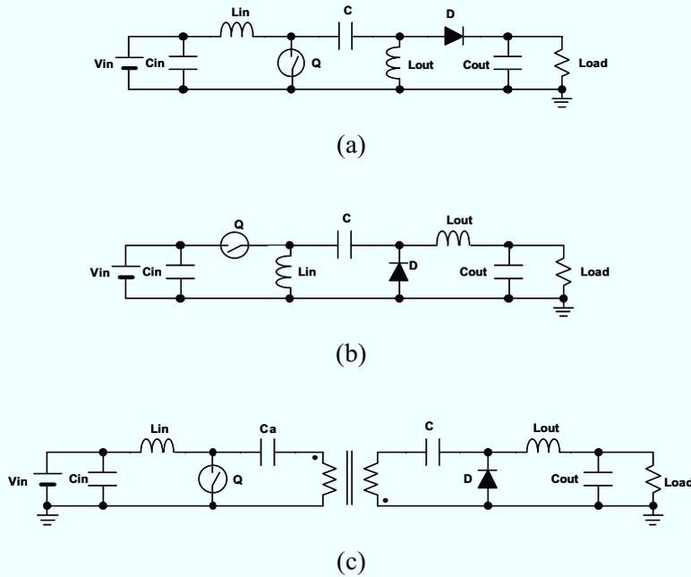
Fig. 5.6.1. Traditional buck-boost converters that can be used as the basic topology for the proposed cell voltage equalizers. (a) SEPIC, (b) Zeta, and (c) isolated Ćuk converters.
