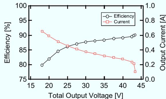
Fig. 6.5.5. Experimental efficiency performance and output current as a function of total output voltage (sum of  $V_1 - V_3$ ) when  $V_1 - V_3$  are uniform.
