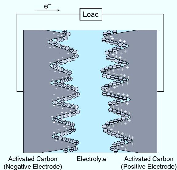
Fig.2.3.1. Image of positive and negative electrode structures of electric double-layer capacitor.
