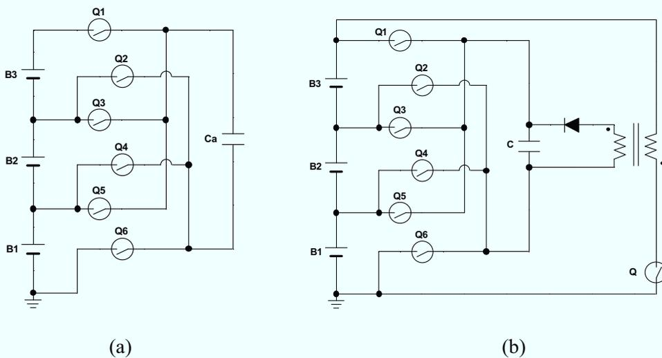
Fig. 5.3.7. Equalizers using a single converter and selection switches based on (a) flying capacitor and (b) flyback converter.
