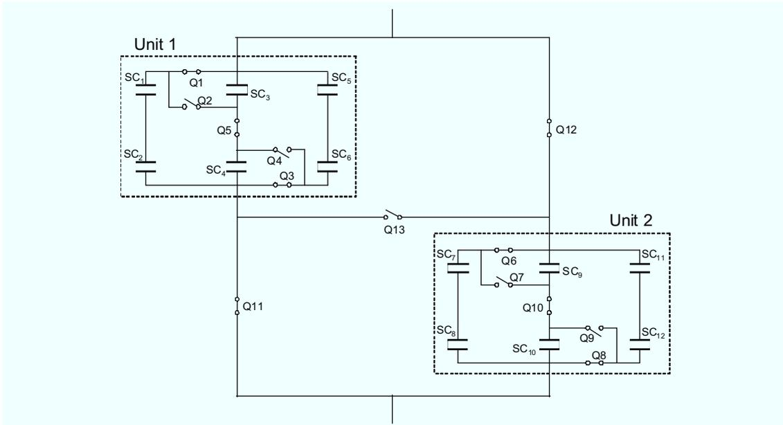
Fig. 7.4.6. Reconfigurable series-parallel SC energy storage system.
