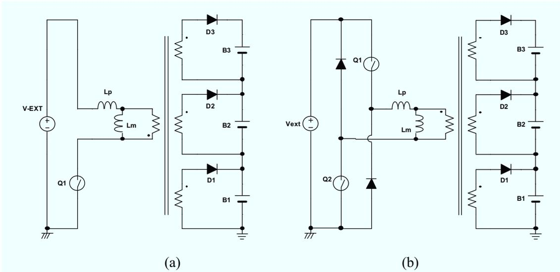
Fig. 6.3.1. Conventional equalization charger using a multi-winding transformer based on (a) flyback converter and (b) forward converter.
