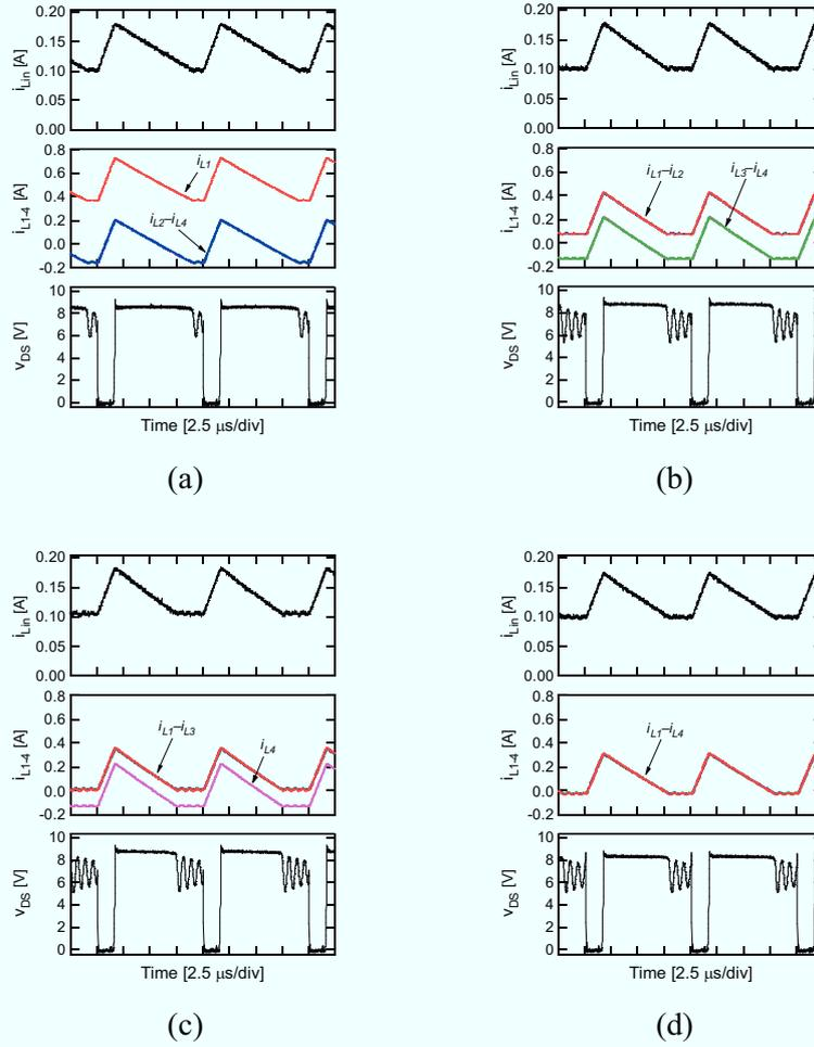
Fig. 5.6.10. Resultant waveforms during Periods (a) A, (b) B, (c) C, and (d) D.
