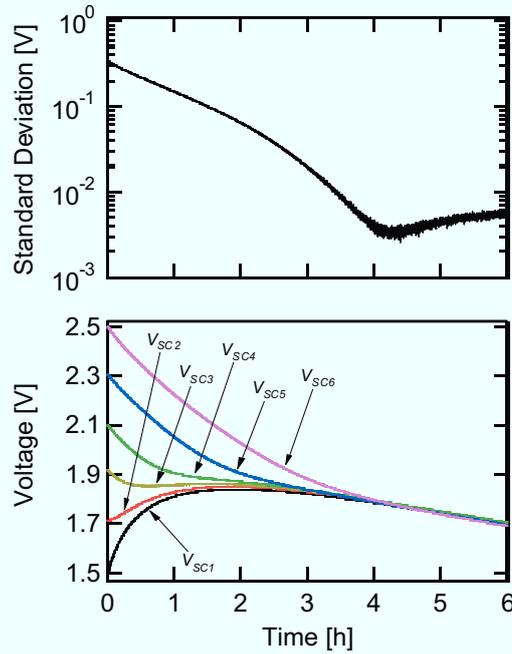
Fig. 5.7.8. Experimental equalization profiles.
