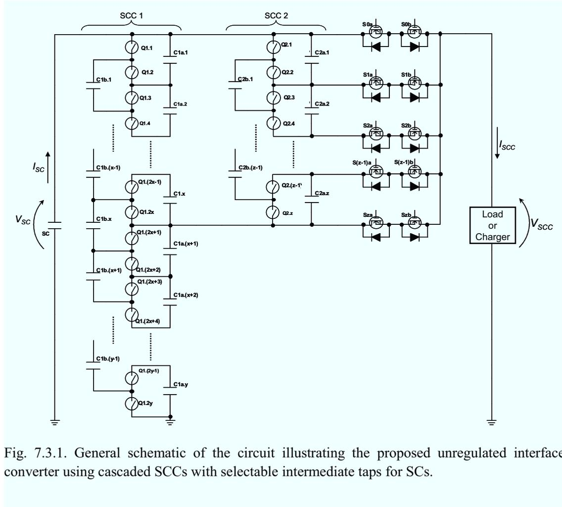
Fig. 7.3.1. General schematic of the circuit illustrating the proposed unregulated interface converter using cascaded SCCs with selectable intermediate taps for SCs.
