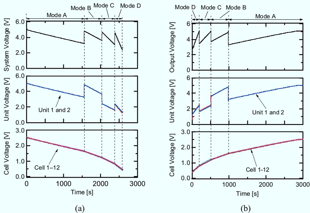
Fig. 7.4.7. System, module, and cell voltage curves during (a) discharging and (b) charging.
