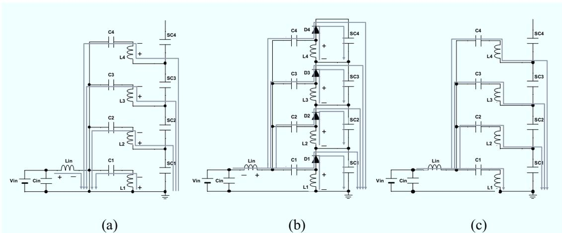
Fig. 6.4.3. Current flow directions during (a)  $T_{on}$ , (b)  $T_{off-a}$ , and (c)  $T_{off-b}$  of the SEPIC-based equalization charger under a cell-voltage-balanced condition.
