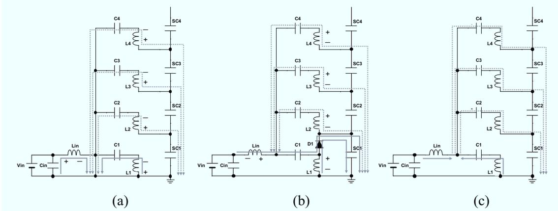
Fig. 6.4.5. Current flow directions during (a)  $T_{on}$ , (b)  $T_{off-a}$ , and (c)  $T_{off-b}$  of the SEPIC-based equalization charger under a cell voltage-imbalanced condition.
