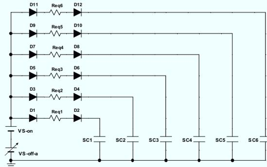
Fig. 5.7.5. DC equivalent circuit of the proposed equalizer.
