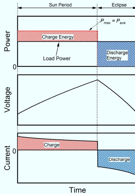
Fig. 4.3.4. Notional profiles of a LIC using CP charging scheme and PV power during LEO-emulated charge-discharge cycling.
