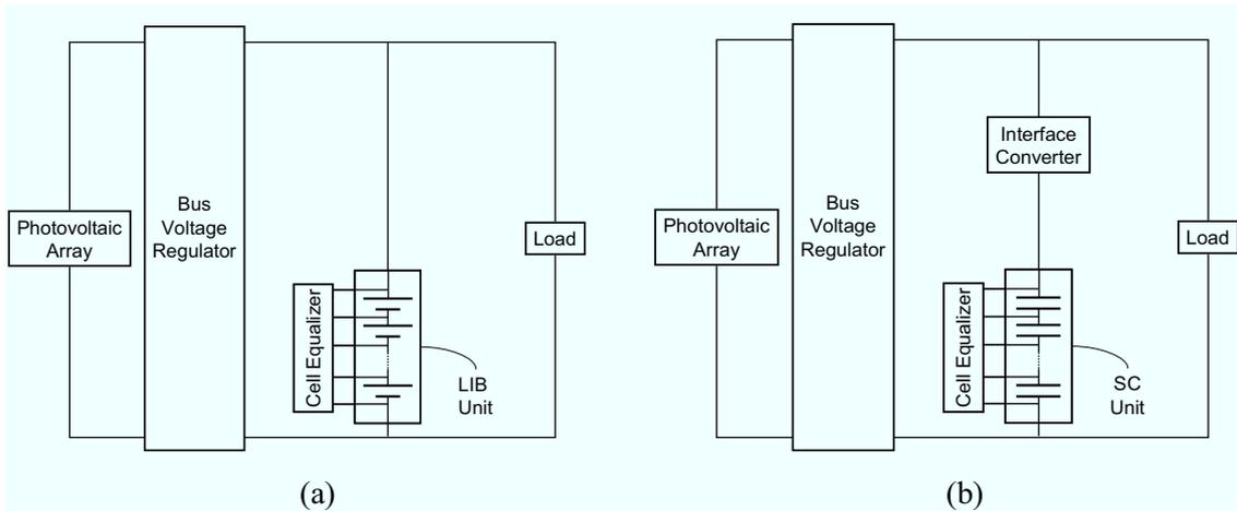
Fig. 2.5.3. Unregulated bus architectures for (a) LIB-based and (b) SC-based systems.
