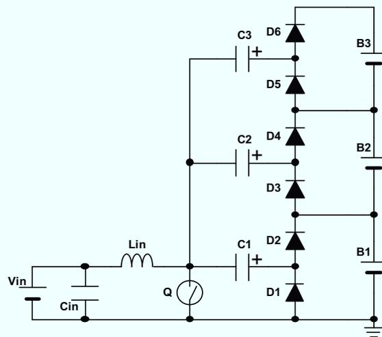
Fig. 6.5.1. Proposed single-switch single-inductor equalization charger using a voltage multiplier for series-connected energy storage modules.
