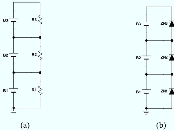
Fig. 5.3.1. Dissipative equalizers using (a) resistors and (b) Zener diodes.
