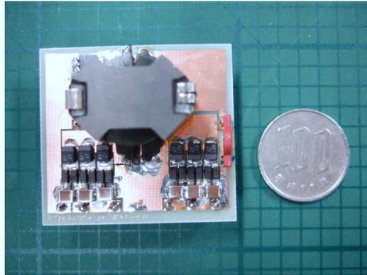
Fig. 5.7.7. Photographs of the prototype of the proposed equalizer.
