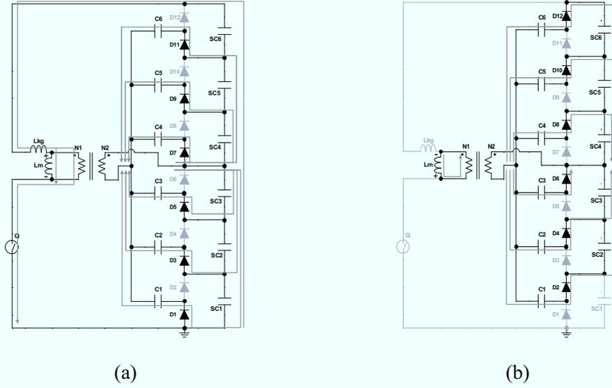
Fig. 5.7.3. Current flow directions during (a) on and (b) off period ( $T_{off-a}$ ).
