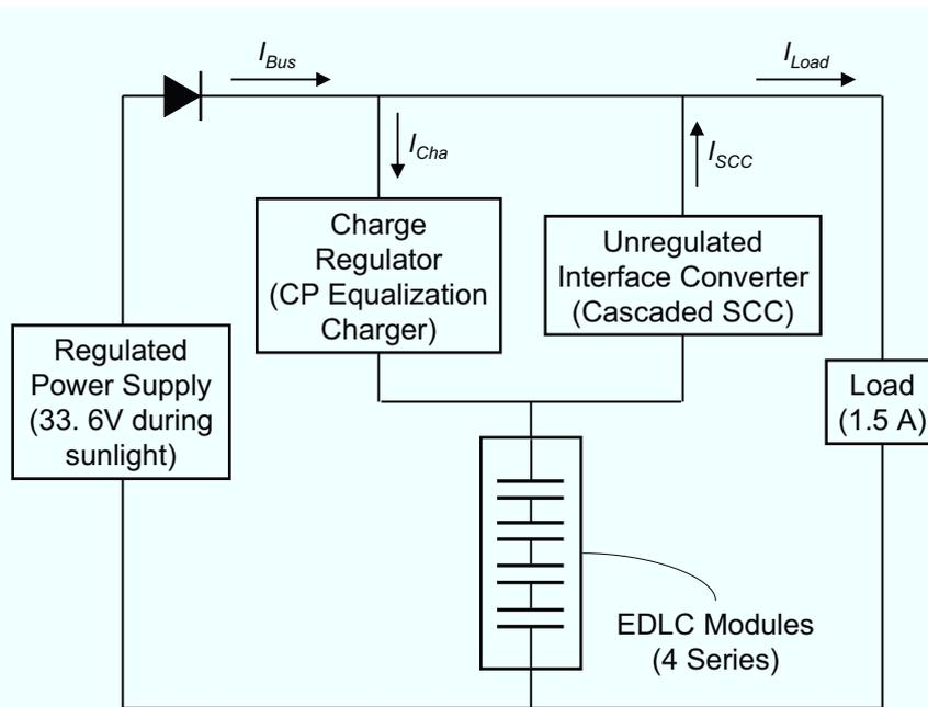
Fig. 8.5.1. System configuration for experimental SC-based sun-regulated 28-V bus system.
