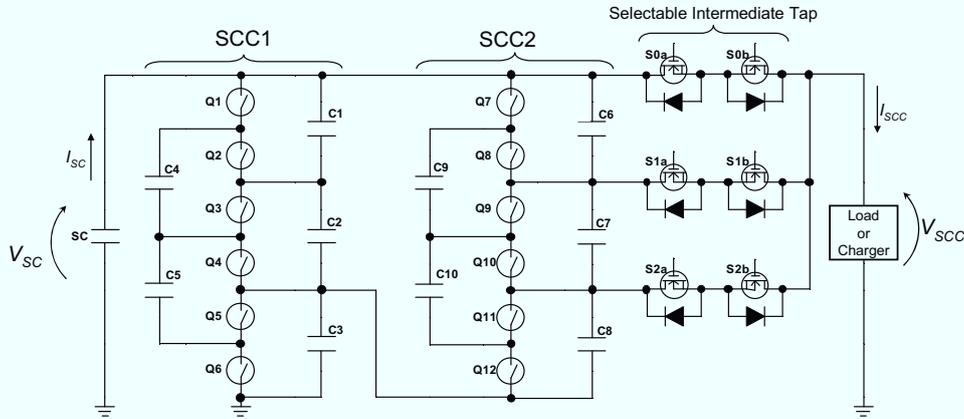
Fig. 7.3.4. Unregulated interface converter designed for an SC with  $V_{cha} = 60.0$  V to satisfy  $V_U = 33.6$  V and  $V_L = 24.0$  V.
