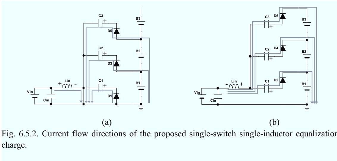
Fig. 6.5.2. Current flow directions of the proposed single-switch single-inductor equalization charge.
