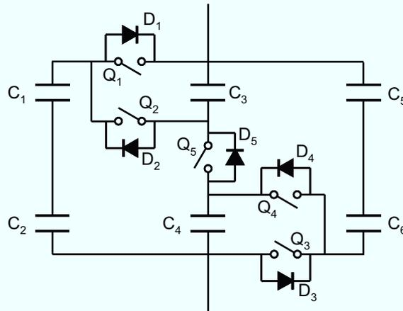
Fig. 7.4.1. Proposed SC reconfiguration circuit.
