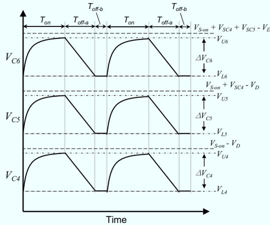
Fig. 5.7.4. Voltage waveforms of capacitors,  $C_4-C_6$ , under cell-voltage-balanced condition.
