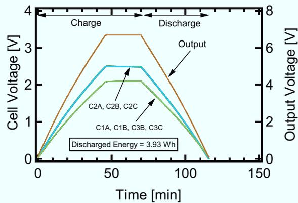
Fig. 5.5.5. Experimental charge/discharge curves of the output and cell voltages without equalization.
