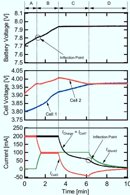
Fig. 5.3.4. Experimental charging profiles of two series LIB cells using shunting equalizers with a 100 mA shunt current.
