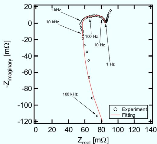
Fig. 5.4.8. Experimental Nyquist plot and corresponding fitting curve of a fresh cell.
