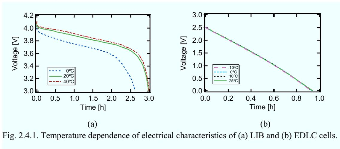
Fig. 2.4.1. Temperature dependence of electrical characteristics of (a) LIB and (b) EDLC cells.
