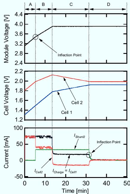
Fig. 5.3.3. Experimental charging profiles of two series EDLCs using shunting equalizers with a 30 mA shunt current.
