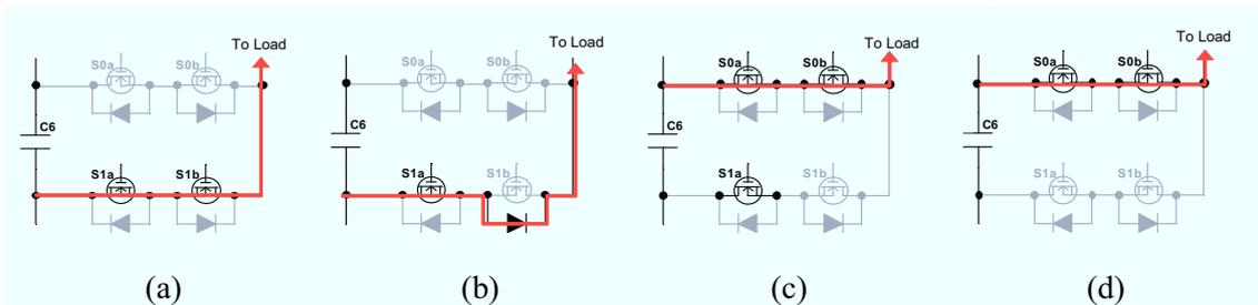
Fig. 7.3.6. Switching sequence of selectable intermediate taps for discharging.
