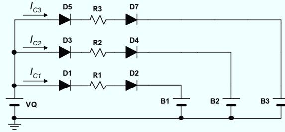
Fig. 6.5.3. Equivalent circuit of the proposed equalization charger for three-series-connected energy storage modules.
