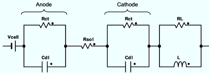
Fig. 5.4.7. Equivalent circuit of a lithium-ion cell for simulation analysis.
