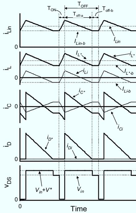
Fig. 5.6.5. Operating waveforms of the SEPIC-based equalizer under cell-voltage-imbalanced condition.
