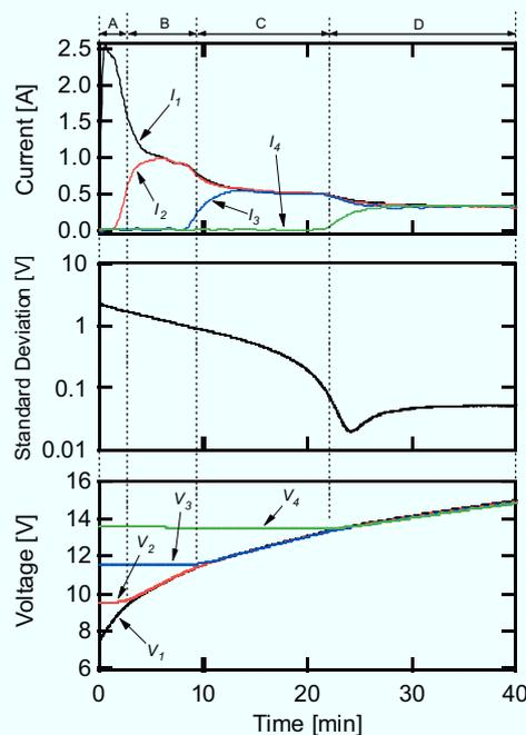
Fig. 6.4.9. Experimental charge profiles of the series-connected EDLC modules.
