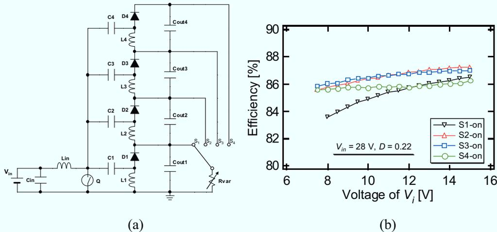
Fig. 6.4.7. (a) Experimental setup for efficiency measurement and (b) the measured power conversion efficiencies.
