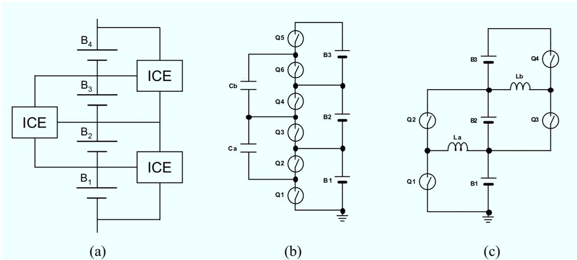
Fig. 5.3.5. Schematic drawing of (a) individual cell equalizers, (b) switched capacitor-based equalizer, and (c) buck-boost converter-based equalizer.
