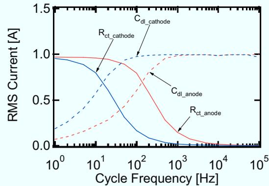
Fig. 5.4.12. Frequency dependence of RMS currents distributing to  $C_{dl}$  and  $R_{ct}$  in the anode and cathode during high-frequency cycling.
