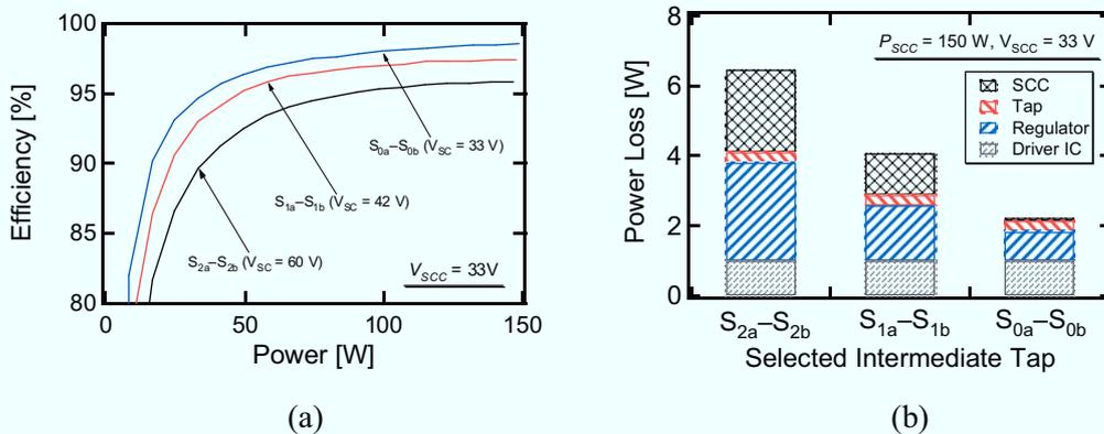
Fig. 7.3.11. (a) Experimental power conversion efficiencies and (b) power loss breakdown at  $V_{SCC} = 33$  V and  $P_{SCC} = 150$  W.
