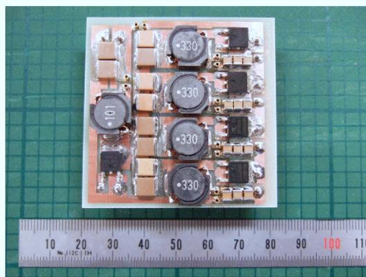
Fig. 6.4.6. A photograph of a 25 W prototype of the SEPIC-based CP equalization charger.
