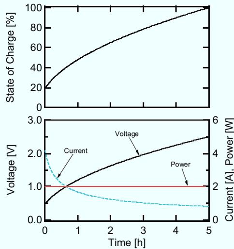
Fig. 4.3.2. Notional charge profiles of an EDLC cell charged with a constant-power (CP) charging scheme.
