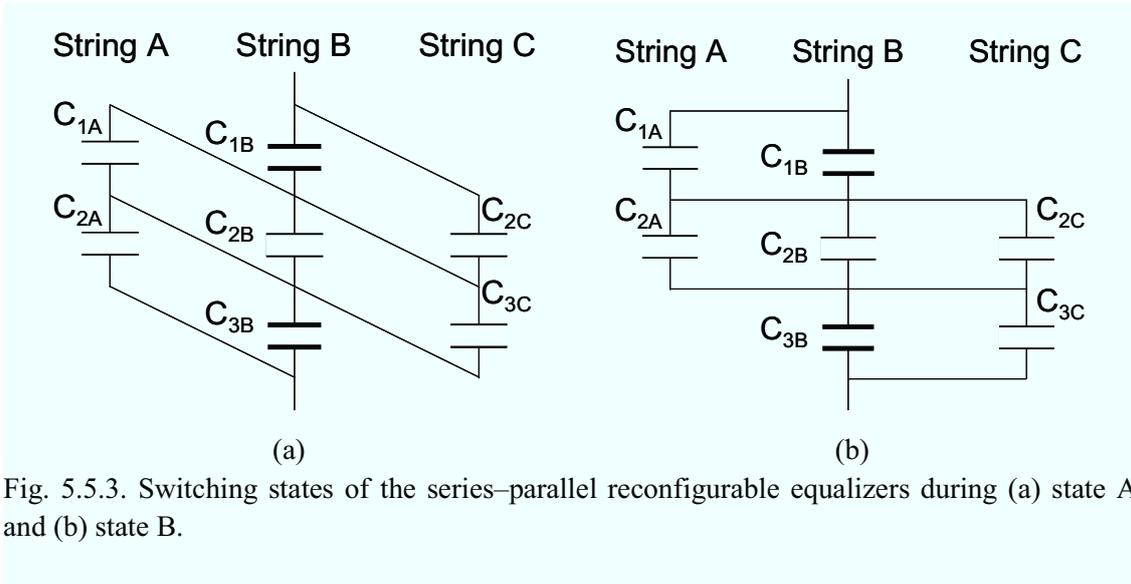
Fig. 5.5.3. Switching states of the series-parallel reconfigurable equalizers during (a) state A and (b) state B.
