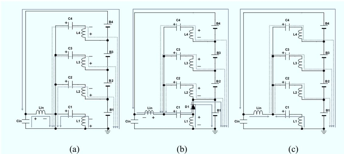
Fig. 5.6.6. Current flow directions during (a)  $T_{on}$ , (b)  $T_{off-a}$ , and (c)  $T_{off-b}$  of the SEPIC-based equalizer under cell-voltage-imbalanced condition.
