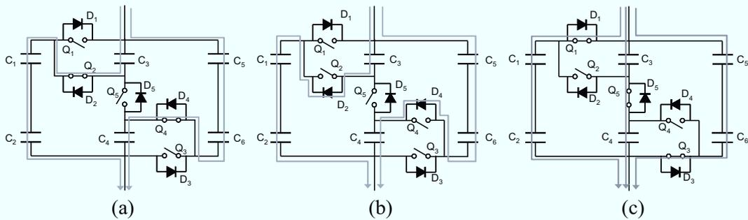
Fig. 7.4.4. Current flow directions during charging in modes (a) 4, (b) 5, and (c) 6 of the proposed circuit.
