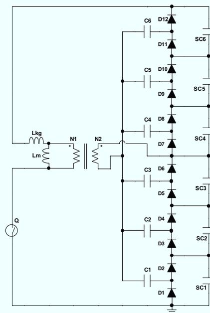
Fig. 5.7.1. Single-switch cell voltage equalizer using voltage multiplier for six SCs connected in series.
