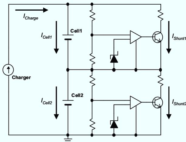
Fig. 5.3.2. Schematic drawing of shunting equalizer.
