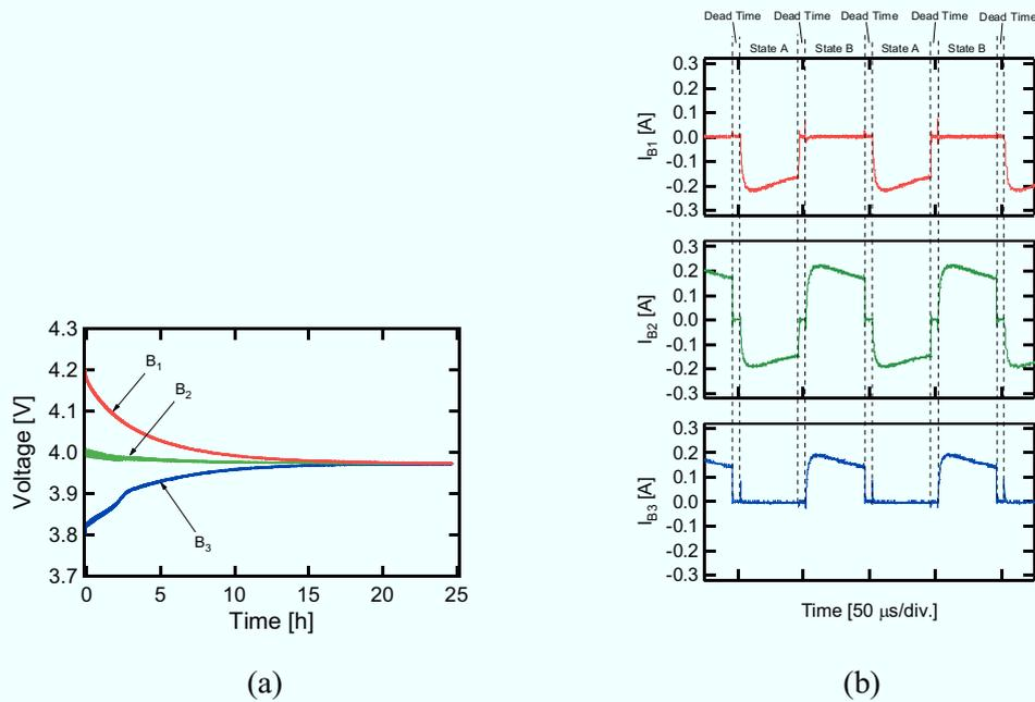
Fig. 5.4.4. Experimental equalization using switched capacitor equalizers. (a) equalization profiles and (b) current waveforms 2 h after the start of equalization.
