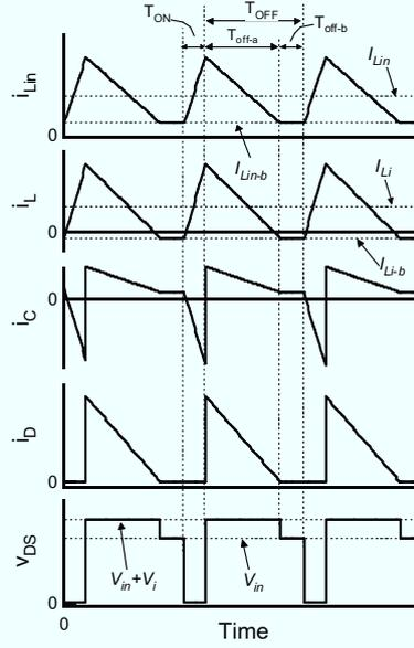
Fig. 6.4.2. Operation waveforms of the SEPIC-based equalization charger under a voltage-balanced condition.
