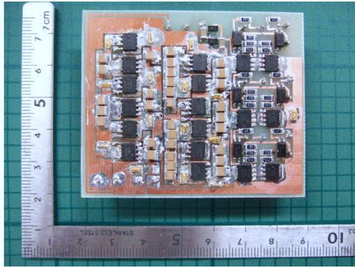
Fig. 7.3.10. Photograph of a 150 W prototype of the proposed unregulated interface converter.
