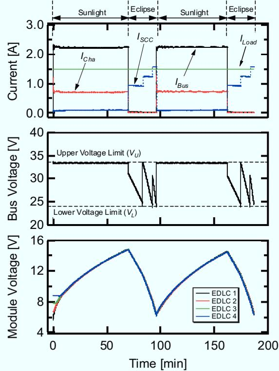
Fig. 8.5.2. Resultant sunlight-eclipse cycling profiles of the experimental SC-based sun-regulated 28-V bus system.
