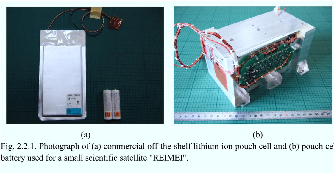
Fig. 2.2.1. Photograph of (a) commercial off-the-shelf lithium-ion pouch cell and (b) pouch cell battery used for a small scientific satellite "REIMEI".
