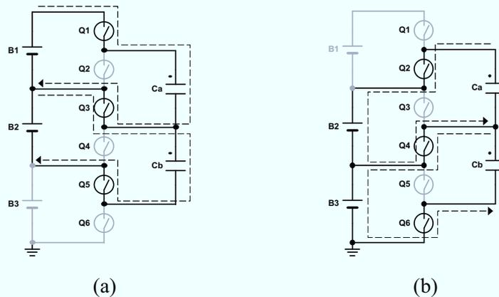
Fig. 5.4.3. Switching states of a switched capacitor equalizer, (a) state A and (b) state B.
