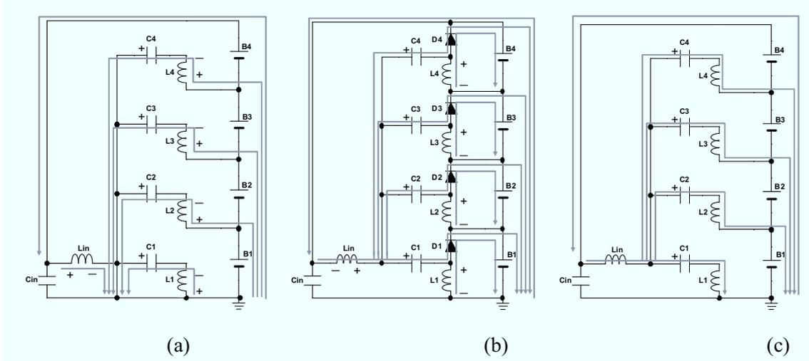
Fig. 5.6.4. Current flow directions during (a)  $T_{on}$ , (b)  $T_{off-a}$ , and (c)  $T_{off-b}$  of the SEPIC-based equalizer under cell-voltage-balanced condition.
