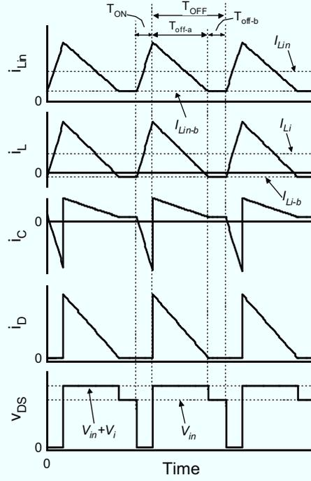
Fig. 5.6.3. Operating waveforms of the SEPIC-based equalizer under cell-voltage-balanced condition.
