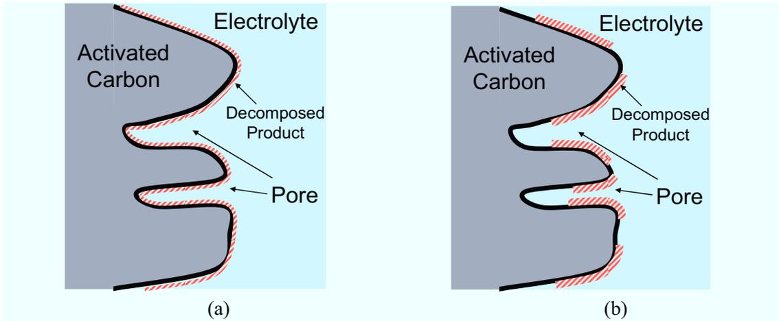
Fig. 3.4.3. Deposition of decomposed products on activated carbon electrode during (a) floating conditions and (b) cycling.
