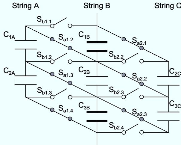
Fig. 5.5.1. Series-parallel reconfigurable equalization circuit.
