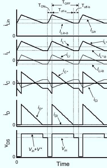
Fig. 6.4.4. Operation waveforms of the SEPIC-based equalization charger under a voltage-imbalanced condition.
