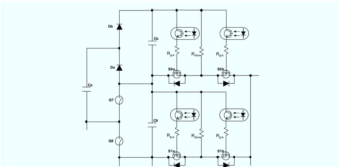
Fig. 7.3.5. Drive circuits for selectable intermediate taps.
