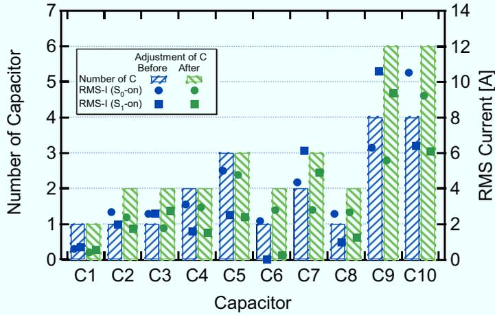
Fig. 7.3.9. The number of MLCCs and the RMS current of each capacitor before and after adjustment of the number of MLCCs.
