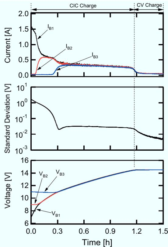
Fig. 6.5.6. Experimental charge profiles of series-connected EDLCs charged from an initially voltage-imbalanced condition.
