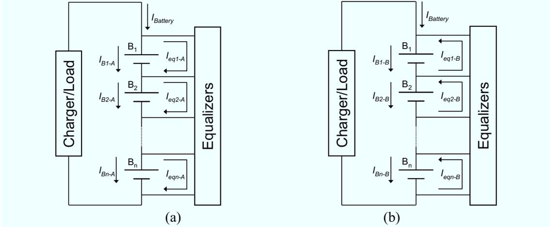
Fig. 5.4.1. Schematic drawing of a battery comprising  $n$  cells connected in series with cell equalizers in (a) state A and (b) state B.
