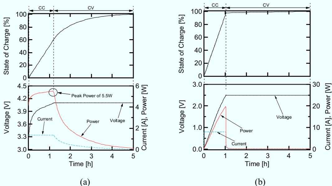
Fig. 4.3.1. Typical charge profiles of (a) a 10-Wh LIB cell and (b) a 10-Wh EDLC cell charged with a constant current–constant voltage (CC–CV) charging scheme.
