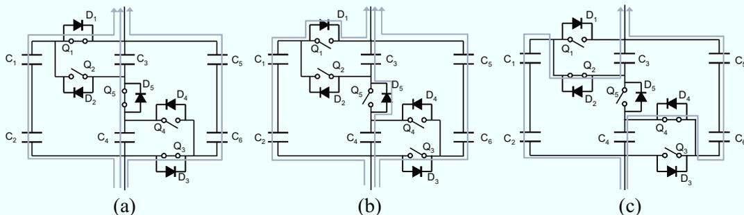
Fig. 7.4.2. Current flow directions during discharging in modes (a) 1, (b) 2, and (c) 3 of the proposed circuit.
