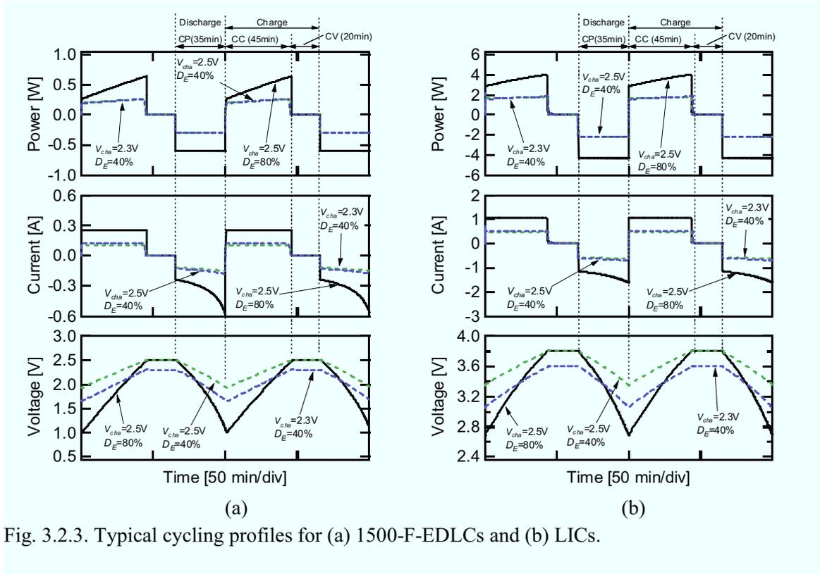
Fig. 3.2.3. Typical cycling profiles for (a) 1500-F-EDLCs and (b) LICs.
