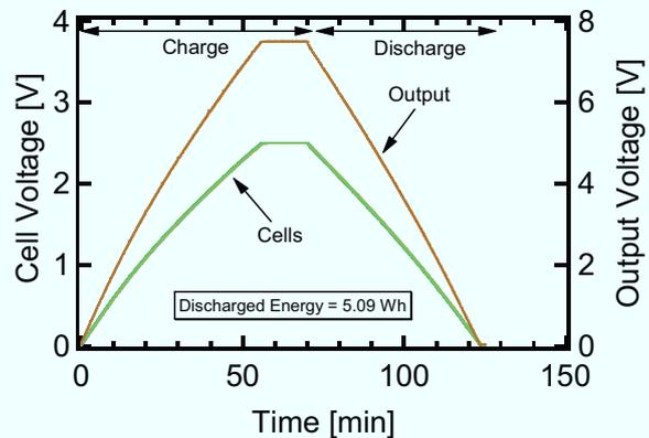
Fig. 5.5.6. Experimental charge/discharge curves of the output and cell voltages with equalization.
