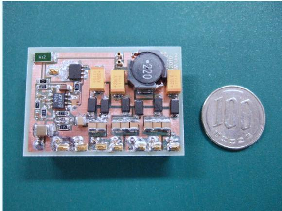
Fig. 6.5.4. Photograph of a 10-W prototype of the proposed equalization charger for three-series-connected energy storage modules.
