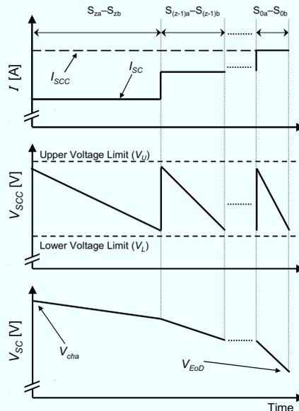
Fig. 7.3.2. Discharging characteristics of an SC with the proposed interface converter using cascaded SCCs with selectable intermediate taps.
