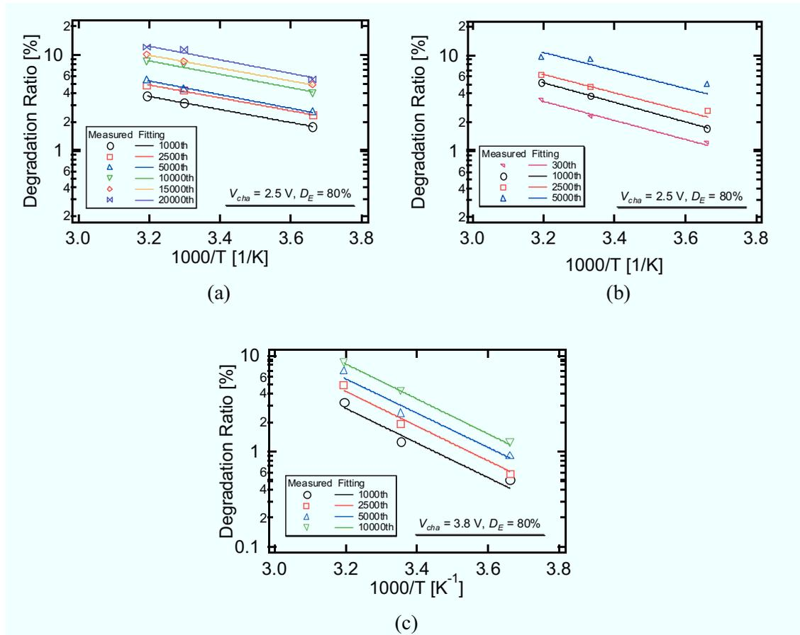
Fig. 3.4.1. Arrhenius plot trends of (a) 1500-F- and (b) 500-F-EDLCs cycled at  $V_{cha} = 2.5 \text{ V}$   $D_E = 80\%$ , and LICs cycled at  $V_{cha} = 3.8 \text{ V}$   $D_E = 80\%$ .
