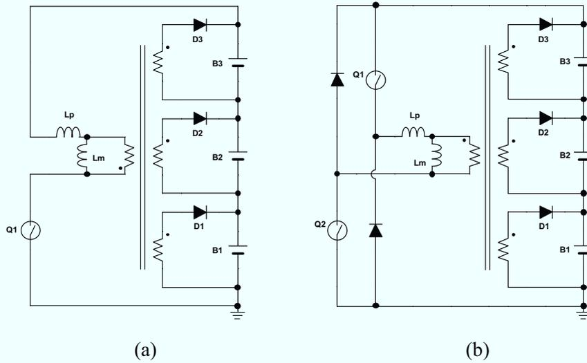
Fig. 5.3.6. (a) Flyback converter- and (b) forward converter-based cell voltage equalizers using a multi-winding transformer.
