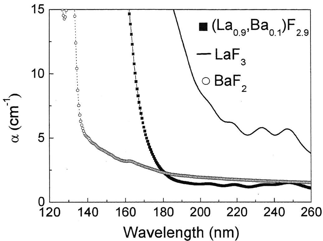
Fig. 6.10. Absorption spectra of 1-mm thick  $(\text{La}_{0.9}, \text{Ba}_{0.1})\text{F}_3$ ,  $\text{LaF}_3$ , and  $\text{BaF}_2$  hosts with absorption edges at 180 nm, 210 nm, and 138 nm, respectively.
