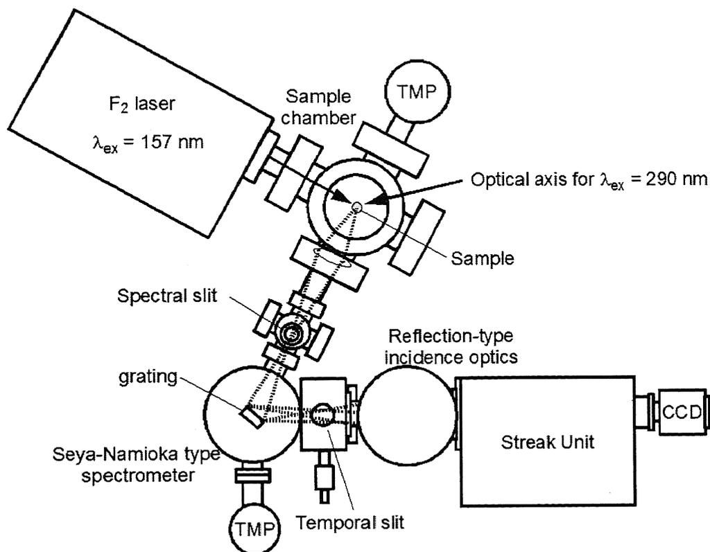
Fig. 5.3. Schematic diagram of the Seya-Namioka spectrometer and streak camera combination used to capture the streak camera image as well as to measure the temporal profile of the fluorescence. The crystal is pumped with the  $F_2$  laser and the third harmonics of a Ti:sapphire regenerative amplifier during independent experiments.
