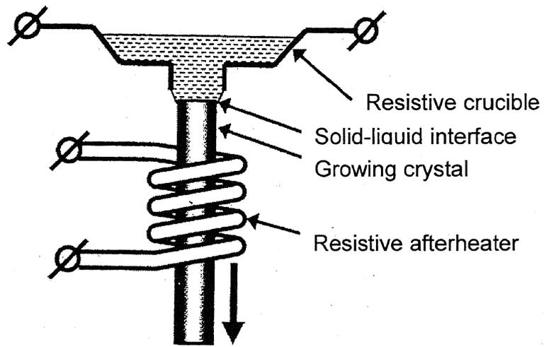
Fig. 4.4. The original resistively-heated  $\mu$ -PD apparatus [3].
