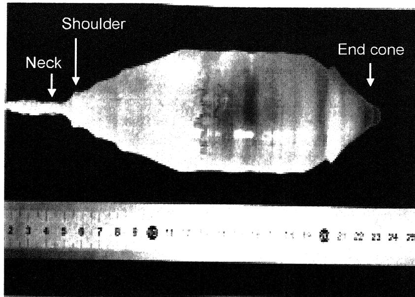
Fig. 4.3. Ce:LiCAF crystal grown by the CZ process. The neck and the conical end are clearly seen.
