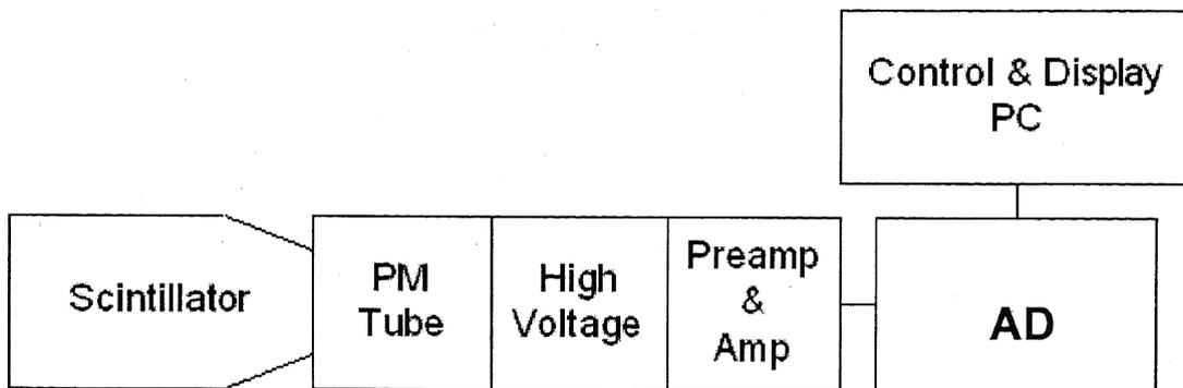
Fig. 3.1. Schematic diagram for the detection of radiation by a scintillator. The scintillator absorbs high-energy radiation and fluoresces at a characteristic Stokes-shifted wavelength, which is readily detectable by conventional detectors such as an avalanche photodiode or a photomultiplier (PMT) tube. The signal is then digitized by an analog-digital converter (AD).
