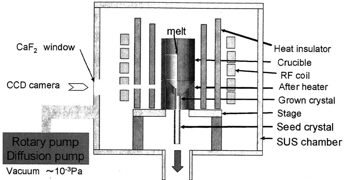
Fig. 4.8. The  $\mu$ -PD apparatus modified for fluoride crystal growth.
