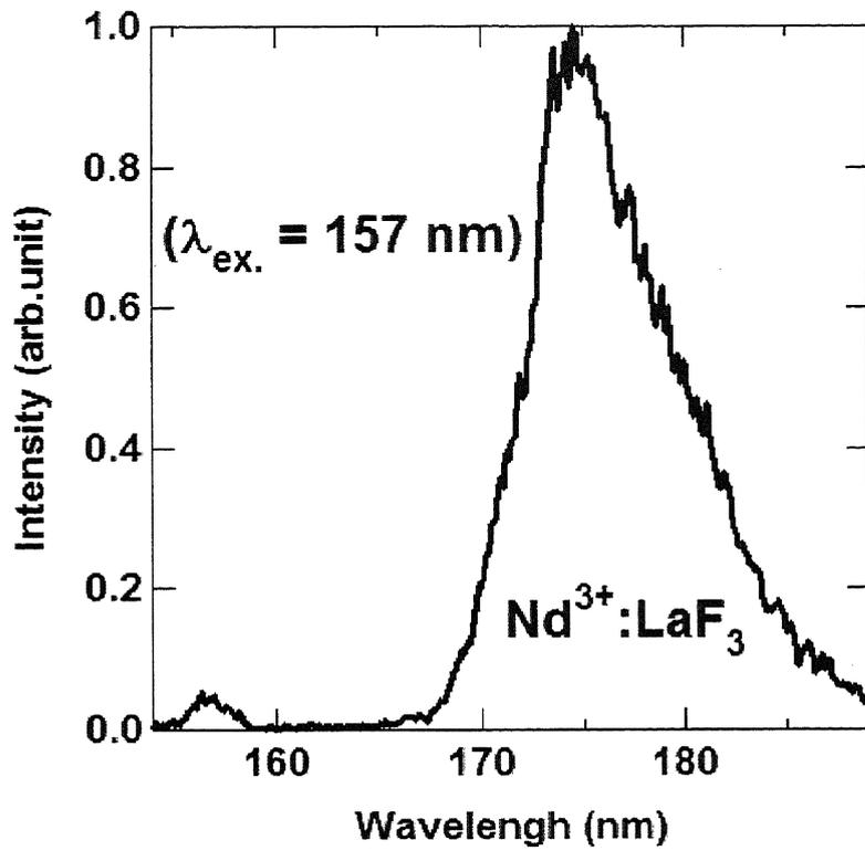
Fig. 6.23. Spectral profile of fluorescence from a cuboid Nd<sup>3+</sup>:LaF<sub>3</sub> excited by 157-nm pulses from an F<sub>2</sub> laser.
