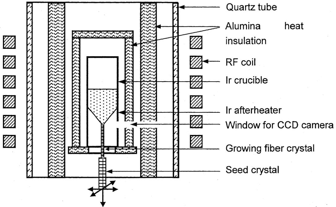
Fig. 4.5. Schematic diagram of the RF heated  $\mu$ -PD apparatus with an Ir crucible. A window for CCD camera allows *in situ* observation of the crystal growth process [3].
