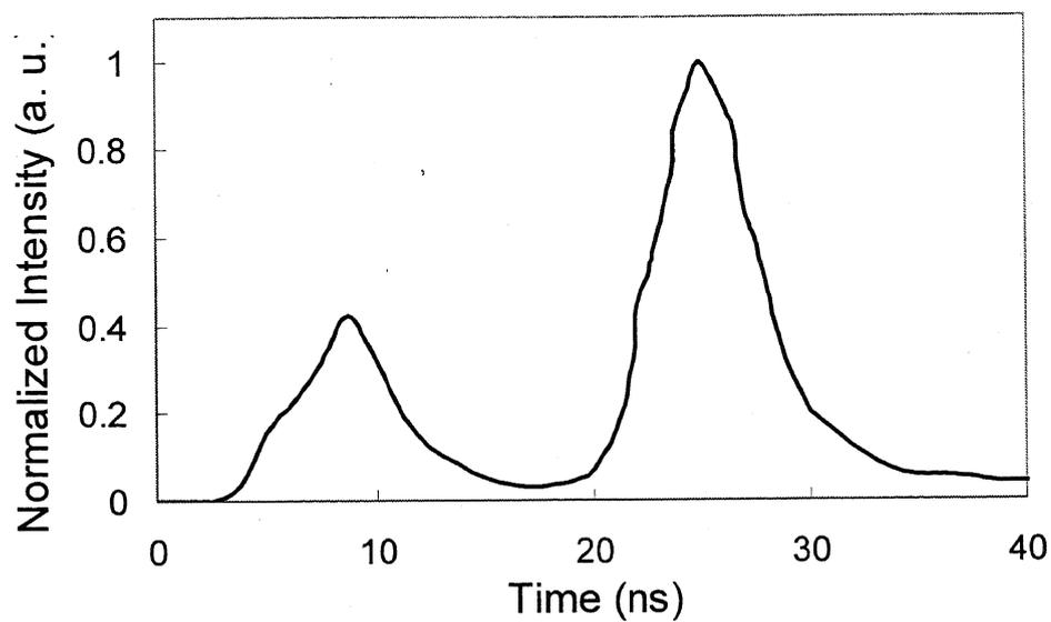
Fig. 5.2. Temporal profile of the F<sub>2</sub> excitation laser. The stronger peak is the 157-nm excitation pulse with a pulse width of 5 ns. The weaker peak comes from the inherent red light (700 nm) emission from fluorine ions.
