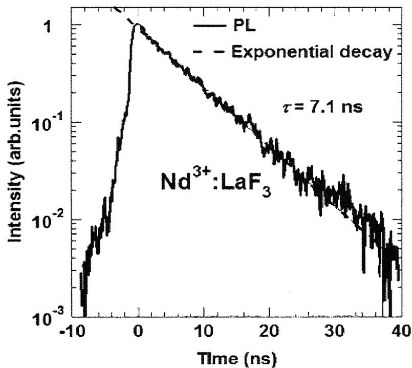
Fig. 6.18. Temporal profile of the fluorescence from a cuboid  $\text{Nd}^{3+}:\text{LaF}_3$  excited by 290-nm femtosecond pulses.
