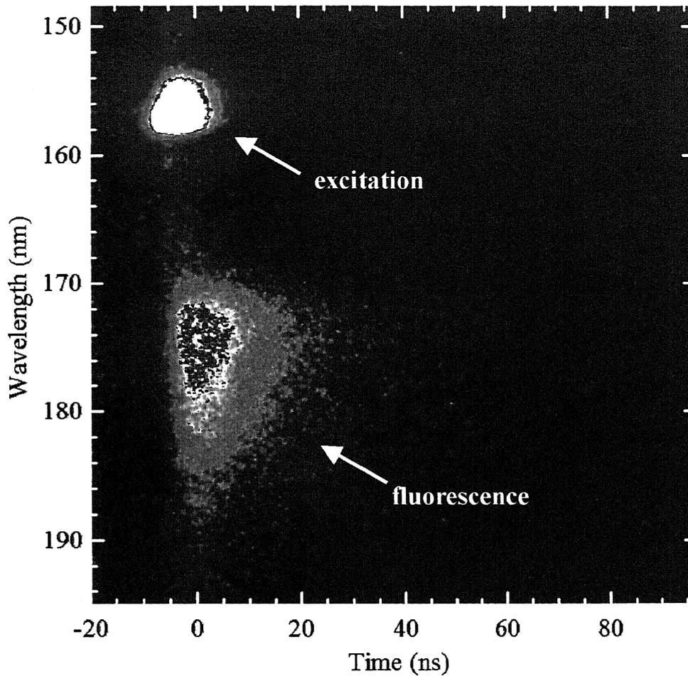
Fig. 6.14. Vacuum ultraviolet streak camera image of the fluorescence from a Nd<sup>3+</sup>:LaF<sub>3</sub> crystal when excited by a F<sub>2</sub> laser. Also shown is the streak camera image of the 157-nm excitation pulse. The image is temporally and spectrally calibrated.
