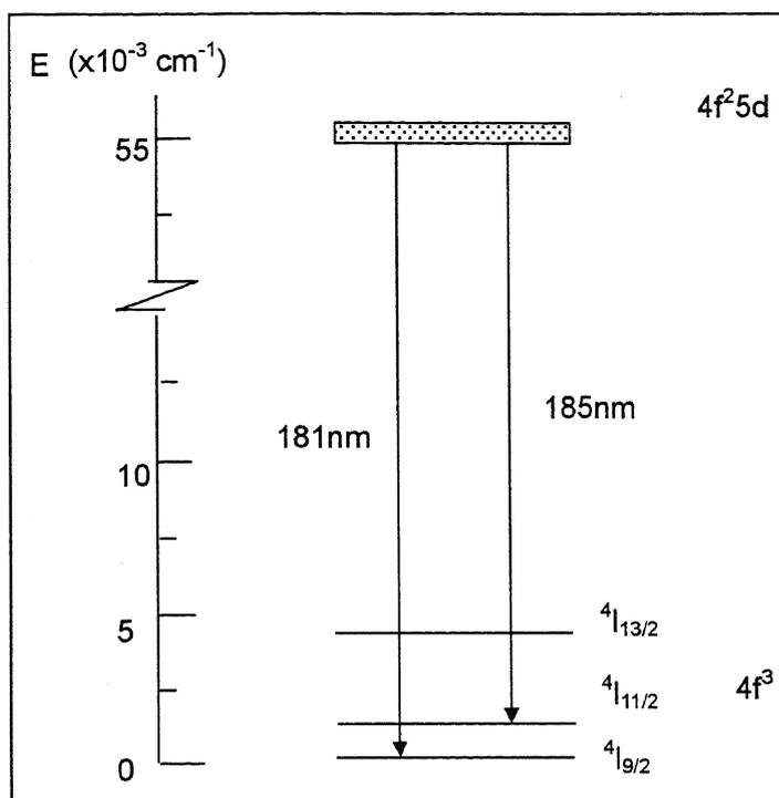
Fig. 6.7. Energy level diagram of Nd<sup>3+</sup>: YLiF<sub>4</sub> showing allowed transition giving rise to fluorescence at 181 nm and 185 nm.
