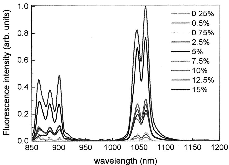
Fig. 6.27. Fluorescence spectra in the near-IR region for different Nd concentrations. Fluorescence intensity decreases for highly doped LaF<sub>3</sub> hosts despite the fact that absorption increases with doping.
