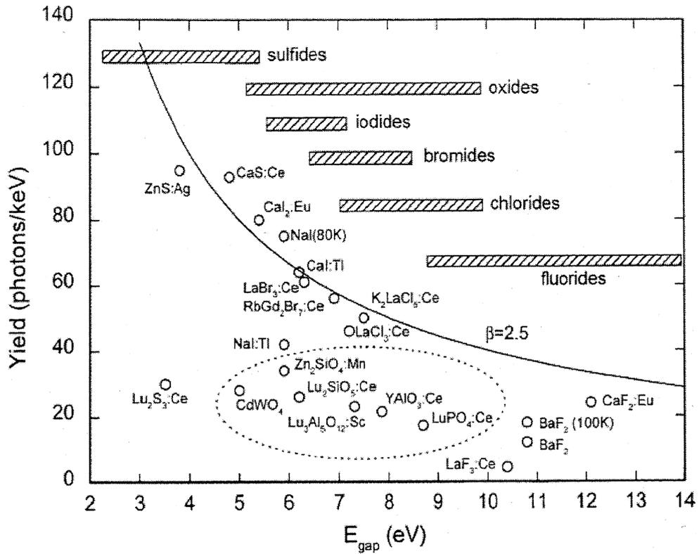
Fig. 3.3. Light yield of different scintillators and cathode ray tube phosphors. The dashed circle indicates some of the most commonly used scintillators.
