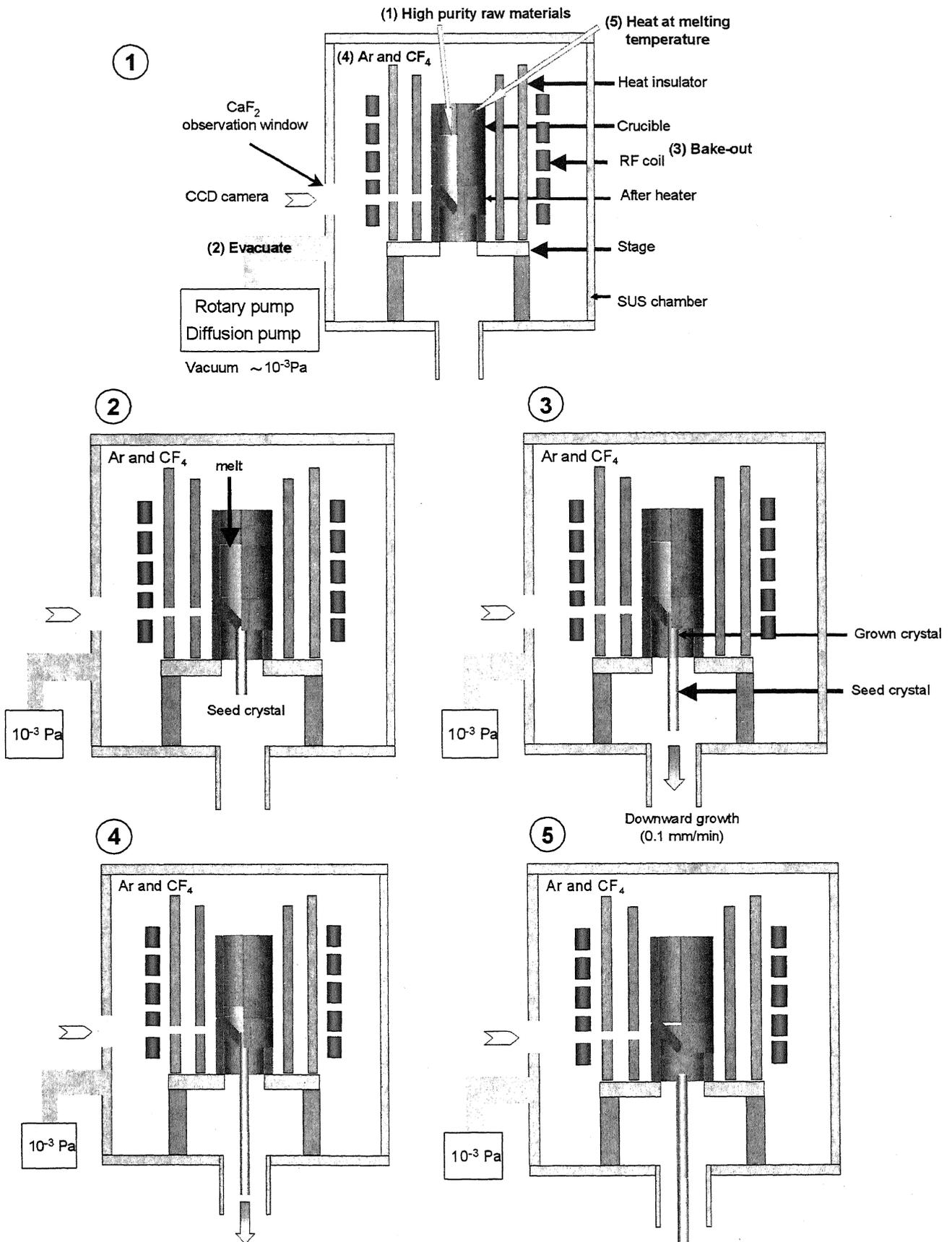
Fig. 5.4. Growth of fluoride crystals by the  $\mu$ -PD method.
