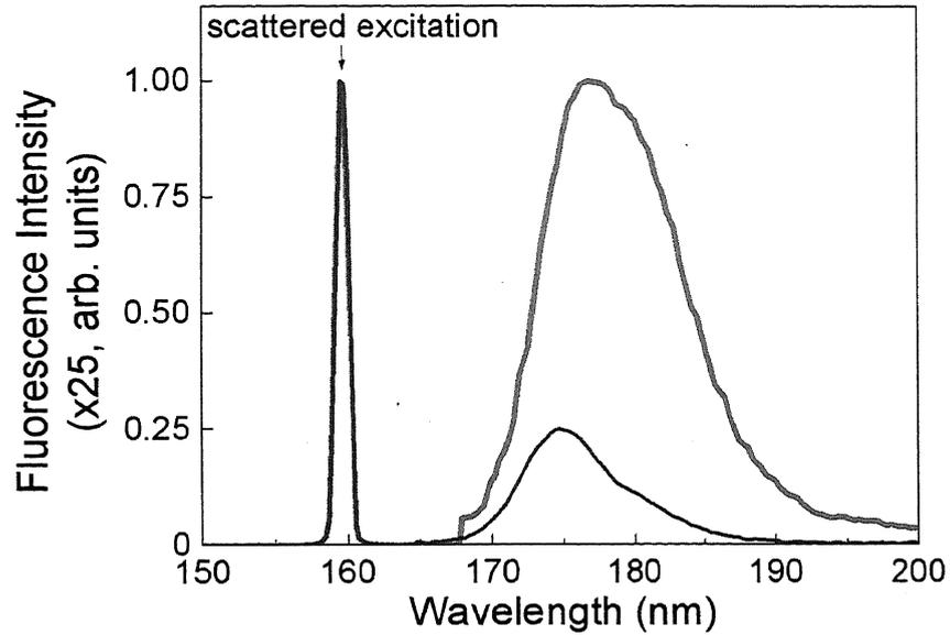
Fig. 6.13. VUV fluorescence spectra of the two samples emphasizing the broader fluorescence bandwidth from Nd<sup>3+</sup>:(La<sub>0.9</sub>Ba<sub>0.1</sub>)F<sub>2.9</sub> with full width at half maximum (FWHM) of 12 nm compared with 8 nm for Nd<sup>3+</sup>:LaF<sub>3</sub>.
