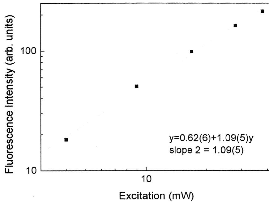
Fig. 6.19. Fluorescence intensity as a function of pump power. The linear dependence with a unity slope implies that fluorescence mechanism may be due to a single photon phenomenon.
