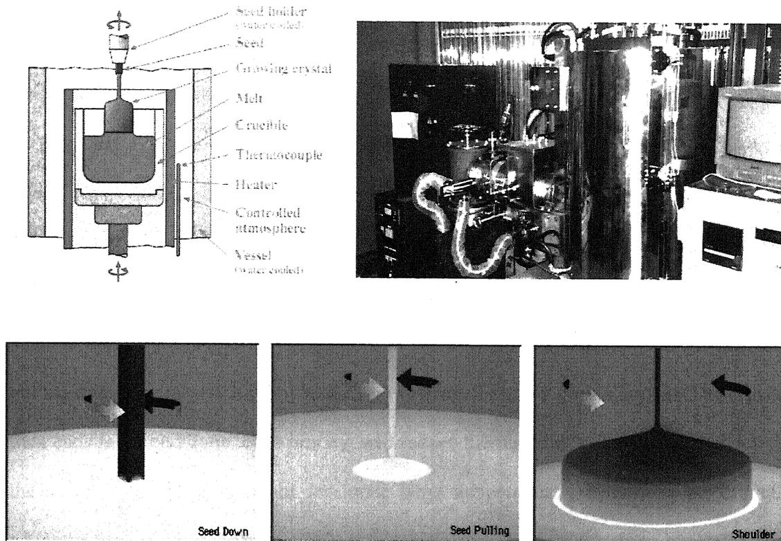
Fig. 4.2. Schematic diagram of the CZ process of pulling a crystal from the melt. Large single crystals are grown by inserting a small seed crystal into a crucible filled with molten raw material. The seed is rotated while slowly pulled up from the melt.
