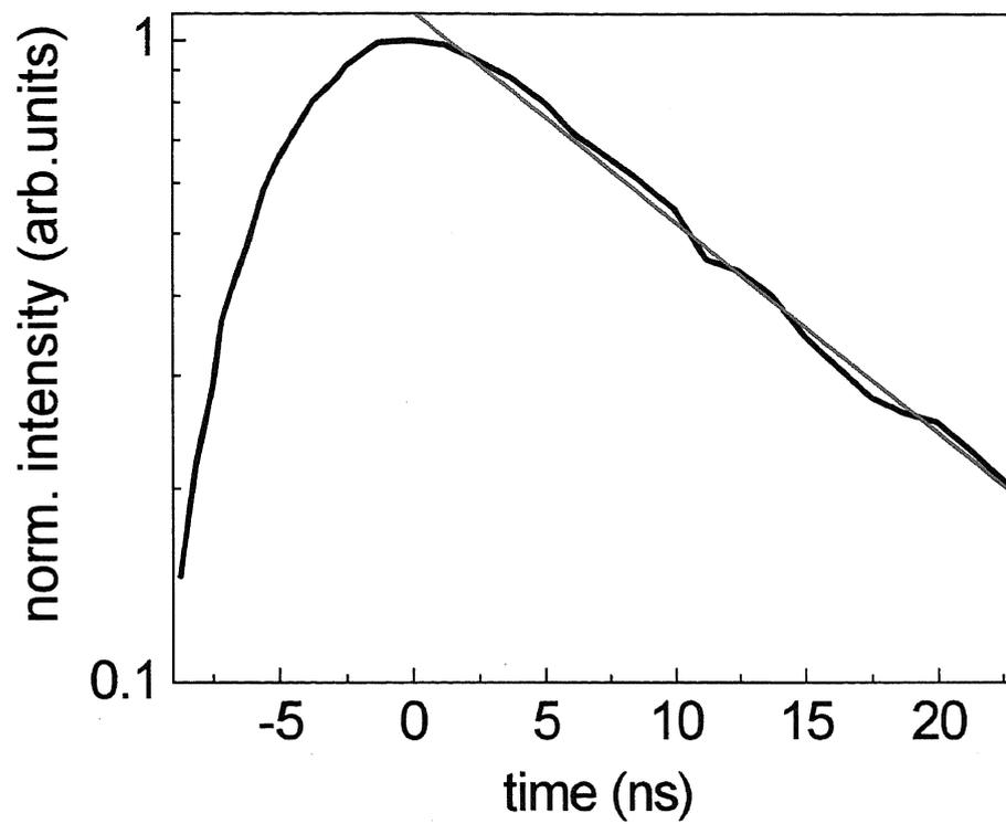
Fig. 6.4. Temporal profile for the decay of Nd<sup>3+</sup>: LaF<sub>3</sub> fluorescence. Lifetime is 9.85 ns.
