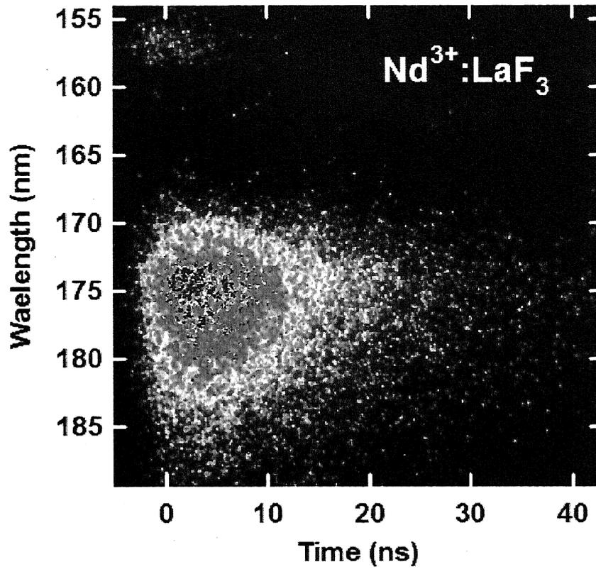
Fig. 6.20. Streak camera image of fluorescence from a cuboid  $\text{Nd}^{3+}:\text{LaF}_3$  excited by 157-nm pulses from an  $\text{F}_2$  laser.
