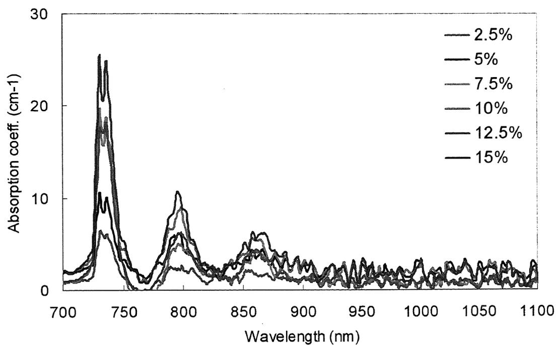
Fig. 6.26. Absorption coefficient in the near-IR region for different Nd concentrations.
