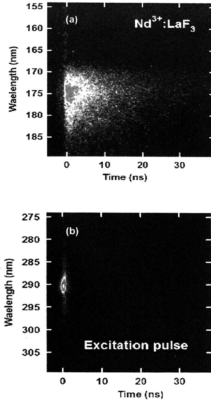
Fig. 6.16. (a) Streak camera image of fluorescence from a cuboid Nd<sup>3+</sup>:LaF<sub>3</sub> excited by 290-nm femtosecond pulses shown in (b).
