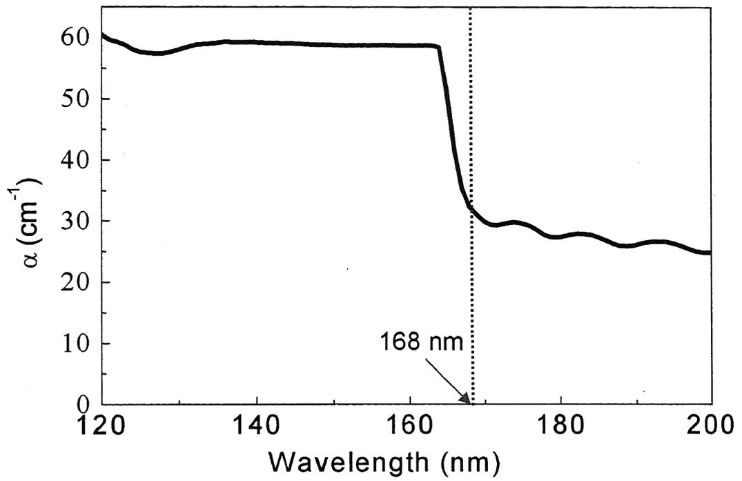
Fig. 6.1. Absorption spectra of a 1 mm thick, CZ method-grown Nd<sup>3+</sup>:LaF<sub>3</sub>.
