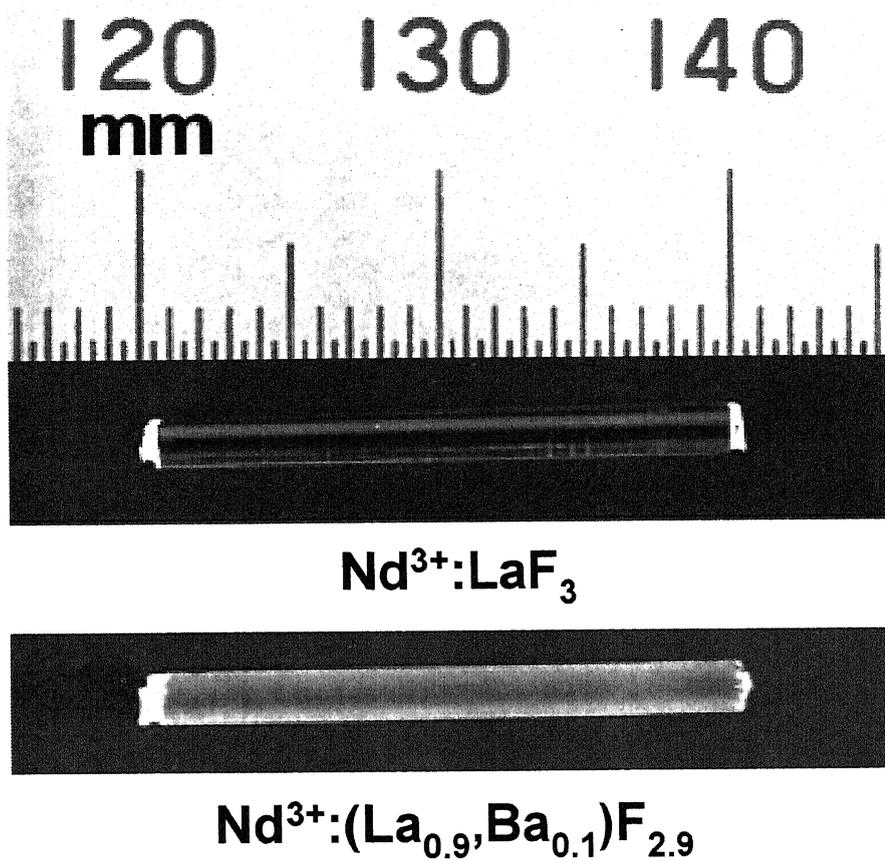
Fig. 6.9. Photographs of (a) Nd<sup>3+</sup>:(La<sub>0.9</sub>Ba<sub>0.1</sub>)F<sub>2.9</sub> and (b) Nd<sup>3+</sup>:LaF<sub>3</sub> crystals. Both samples are 20 mm in length and 2 mm in diameter. Neither has visible cracks nor inclusions.
