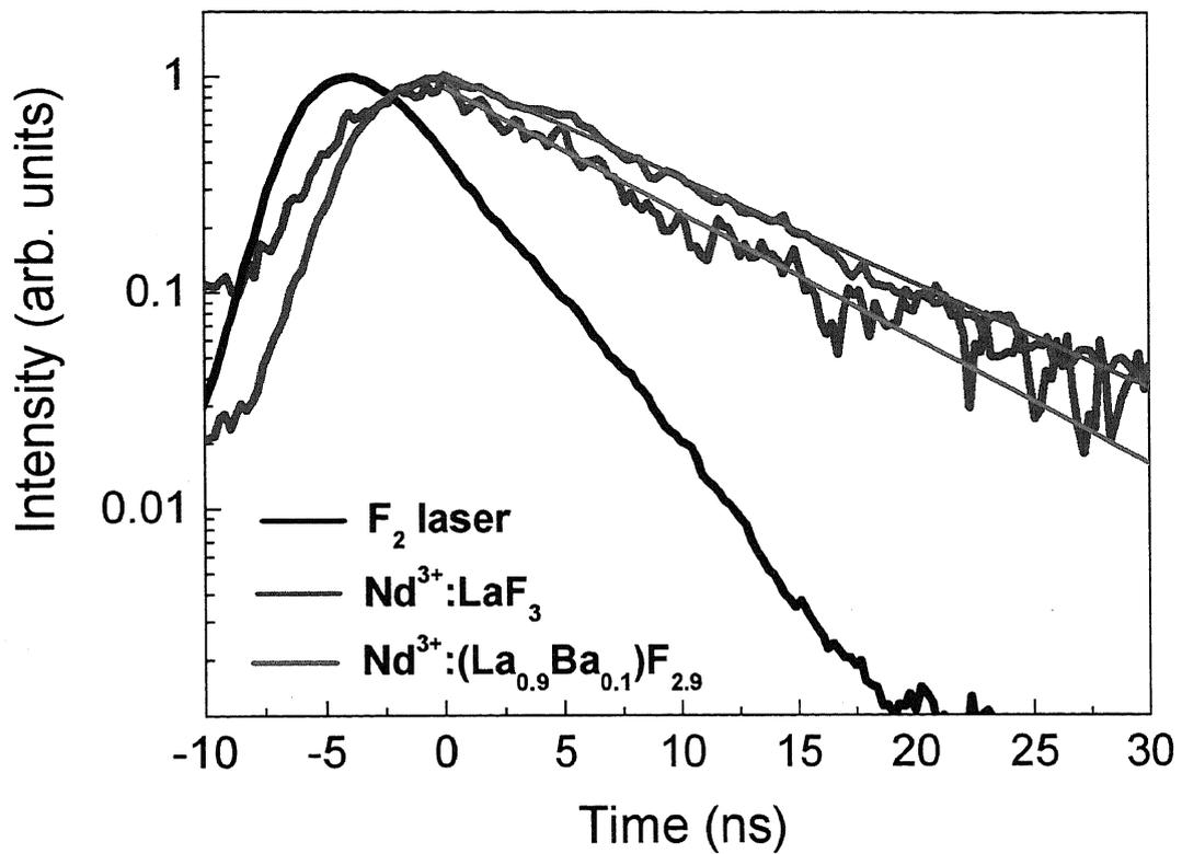
Fig. 6.15. The fluorescence from  $\text{Nd}^{3+}:\text{LaF}_3$  has a lifetime,  $\tau$ , of 8.9 ns while the fluorescence from  $\text{Nd}^{3+}:(\text{La}_{0.9}\text{Ba}_{0.1})\text{F}_{2.9}$  decays faster with a lifetime of 6.1 ns. Also shown is the temporal profile of the excitation pulse with a pulsewidth of 5 ns.
