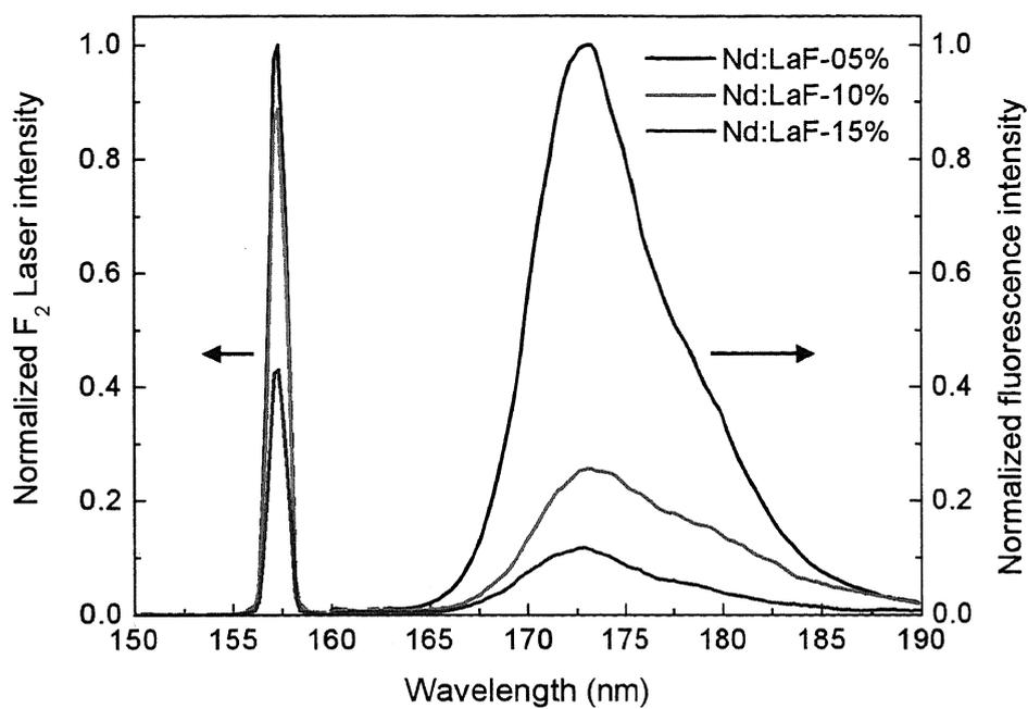
Fig. 6.25. Nd concentration dependence of fluorescence intensity.
