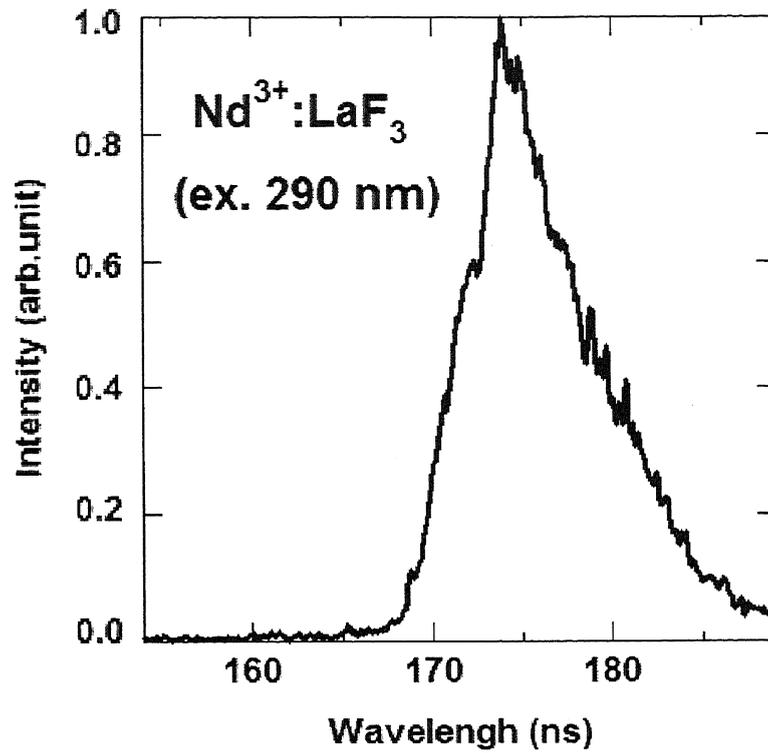
Fig. 6.17. Spectral profile of the fluorescence from a cuboid Nd<sup>3+</sup>:LaF<sub>3</sub> excited by 290-nm femtosecond pulses.
