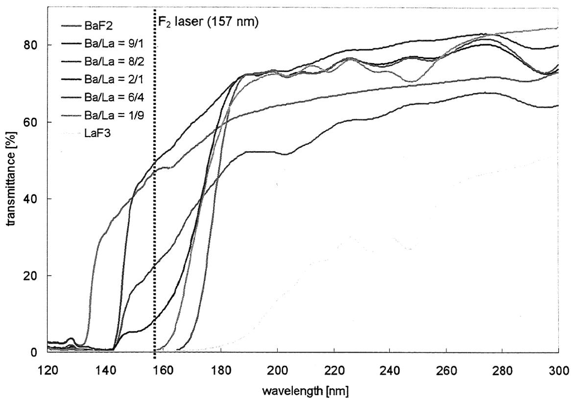
Fig. 5.6. Effect of different Barium/Lanthanum ratios on the transmission characteristics of  $\text{La}_{(1-x)}\text{Ba}_x\text{F}_{3-x}$ . The  $\text{LaF}_3$  curve is included to provide a measure on its transmission range that starts from 170nm.
