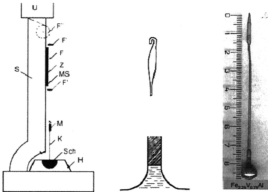
Fig. 4.1. The first CZ apparatus utilized by J. Czochralski. It was used for the growth of metals by immersion of a narrow capillary in the crucible containing the melt.
