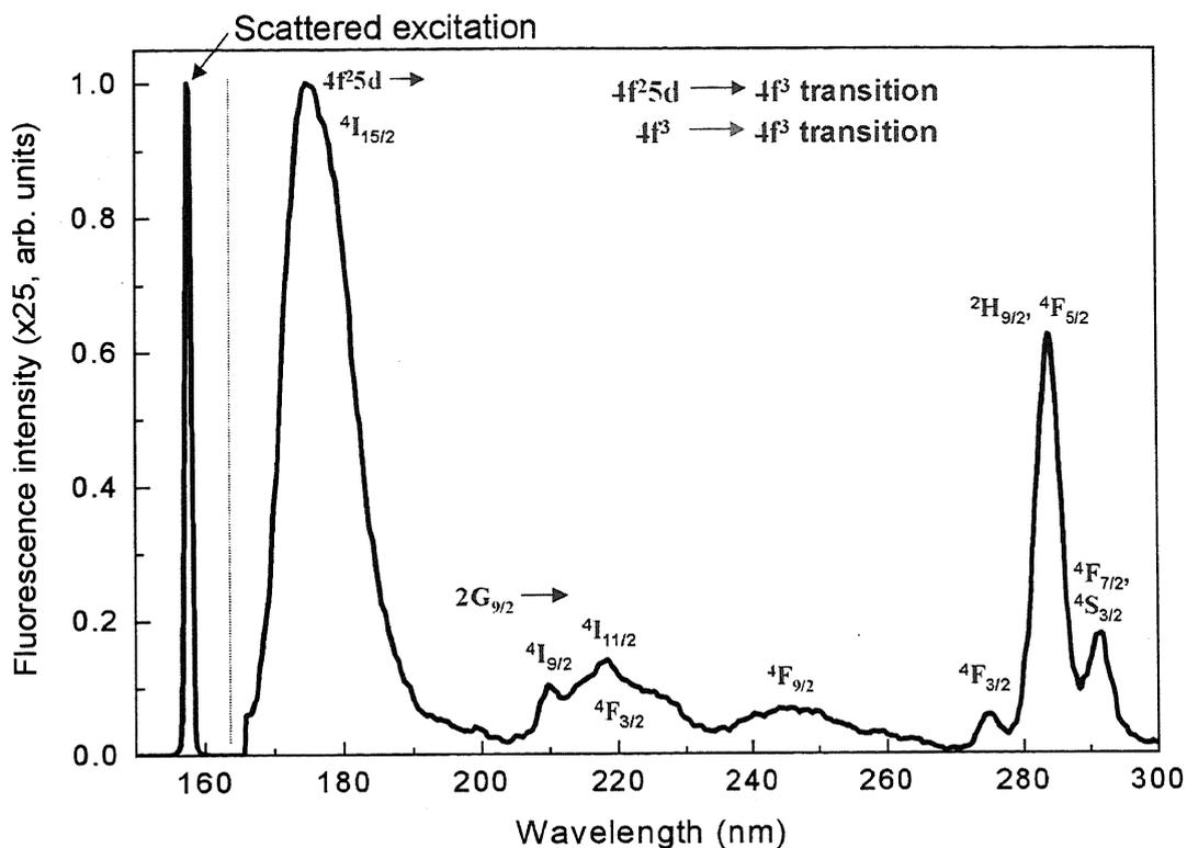
Fig. 6.11.  $\text{F}_2$  laser-induced fluorescence spectra of  $\text{Nd}^{3+}:(\text{La}_{0.9}\text{Ba}_{0.1})\text{F}_{2.9}$ . It has a dominant peak located at 178 nm. The broad peaks can be attributed to interconfigurational transitions from the  $4f^25d$  excited state configuration to the different manifolds of the  $4f^3$  ground state configuration while the sharp peaks are characteristic of intraconfigurational transitions within the manifolds of the  $4f^3$  configuration.
