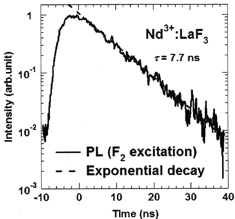
Fig. 6.24. Temporal profile of fluorescence from a cuboid Nd<sup>3+</sup>:LaF<sub>3</sub> excited by 157-nm pulses from an F<sub>2</sub> laser.
