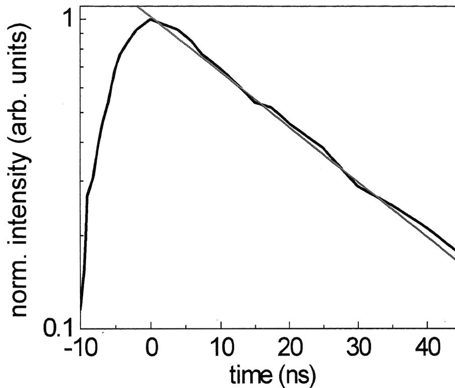
Fig. 6.8. Temporal profile for the decay of Nd<sup>3+</sup>: YLiF<sub>4</sub> fluorescence. It has a lifetime of 21.79 ns.
