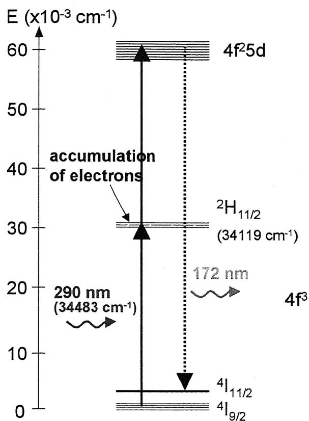
Fig. 6.21. Schematic diagram of the energy level transitions arising to 175-nm fluorescence when pumped with 290-nm femtosecond pulses.
