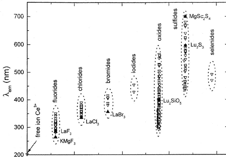
Fig. 3.2. The emission wavelength for the transition between 5d and the ground state of  $Ce^{3+}$  in different compounds. Fluorides are among the hosts that have the shortest emission wavelengths and hence, are among the fastest scintillators.
