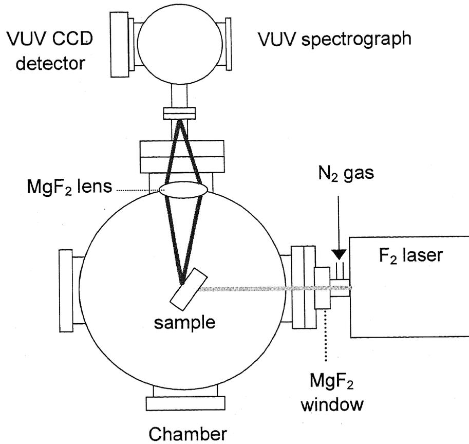
Fig. 5.1. Schematic diagram for measuring the fluorescence spectrum using an F<sub>2</sub> laser excitation.
