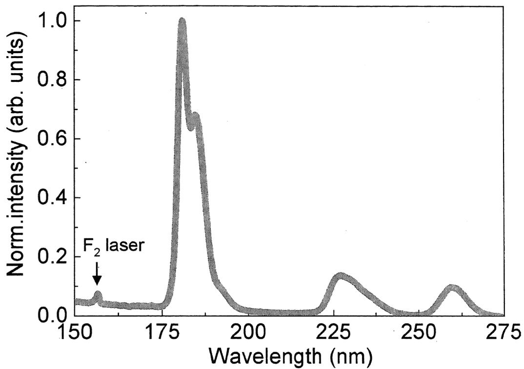
Fig. 6.6. Fluorescence spectra of Nd<sup>3+</sup>: YLiF<sub>4</sub>. Strongest fluorescence peak is located at 181 nm.
