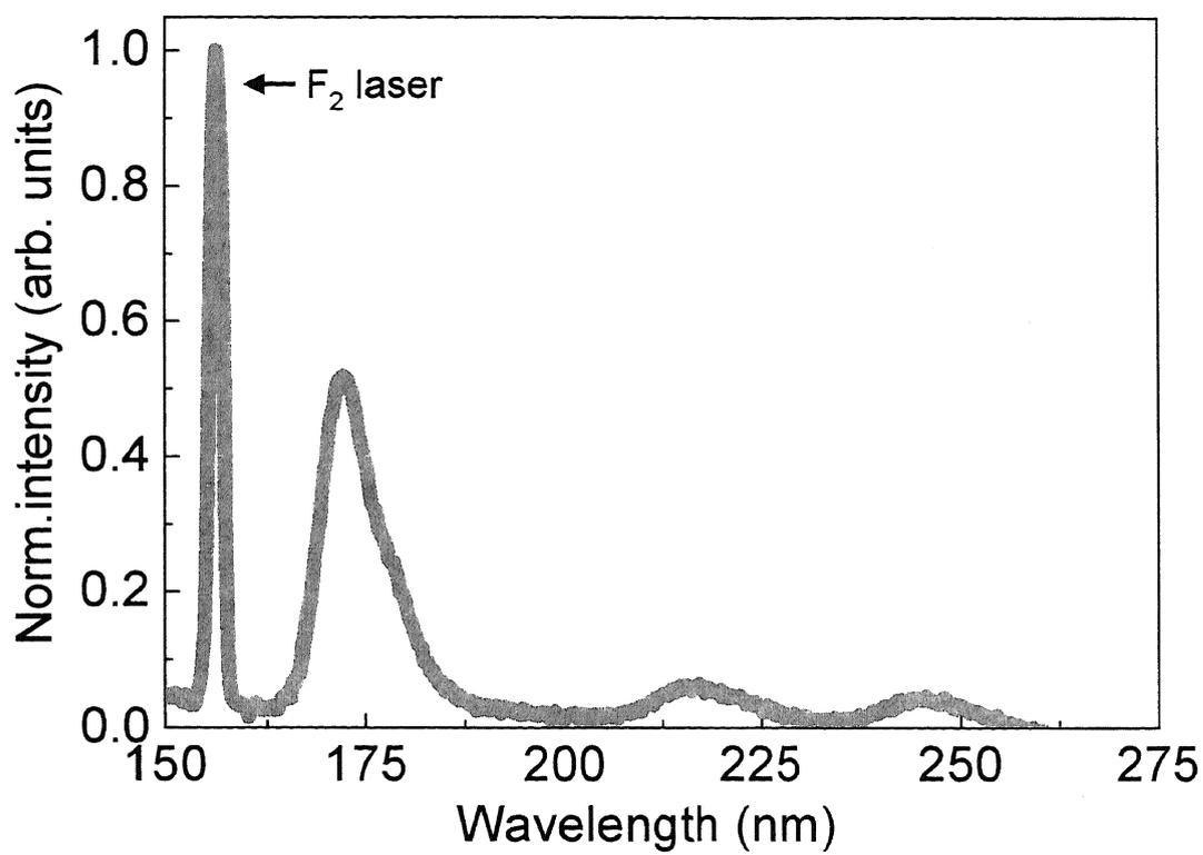
Fig. 6.2. Fluorescence spectra of Nd<sup>3+</sup>: LaF<sub>3</sub>. Strongest fluorescence peak is located at 172 nm.
