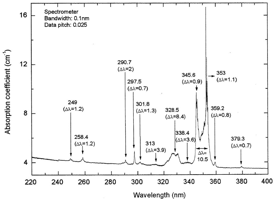
Fig. 6.20. Absorption spectra of a cuboid Nd<sup>3+</sup>:LaF<sub>3</sub> showing multiple absorption bands from 200-400 nm. The sample has an absorption peak at the 290-nm excitatin wavelength.
