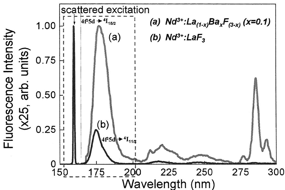
Fig. 6.12.  $\text{F}_2$  laser-induced fluorescence spectra of  $\text{Nd}^{3+}:(\text{La}_{0.9}\text{Ba}_{0.1})\text{F}_{2.9}$  and  $\text{Nd}^{3+}:\text{LaF}_3$ .
