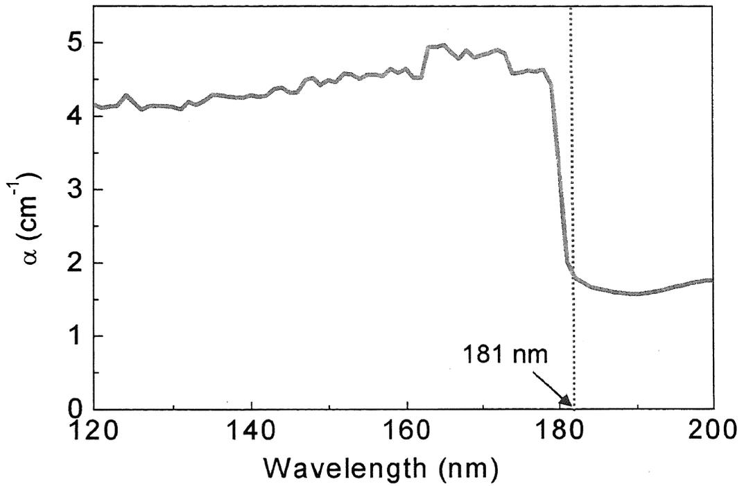
Fig. 6.5. Absorption spectra of a 13 mm thick, CZ method-grown  $\text{Nd}^{3+}:\text{YLiF}_4$ .
