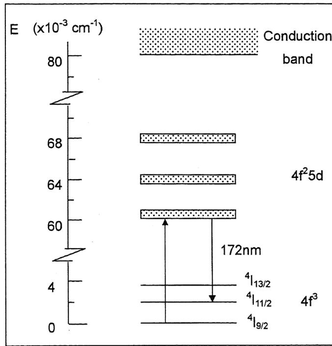
Fig. 6.3. Energy level diagram of Nd<sup>3+</sup>: LaF<sub>3</sub> showing the allowed transition resulting to fluorescence at 172 nm.
