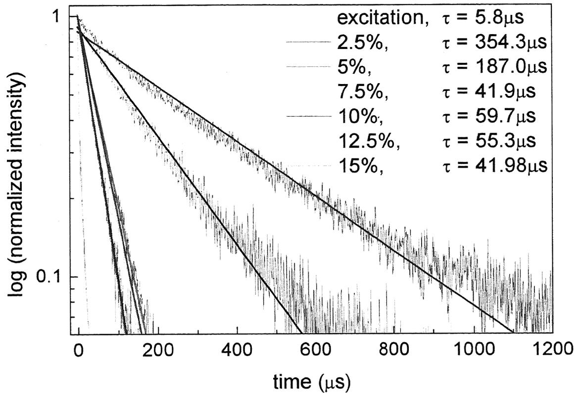
Fig. 6.28. Fluorescence lifetime decreases as doping level increases. This is indicative of fluorescence quenching for highly doped LaF<sub>3</sub> hosts.
