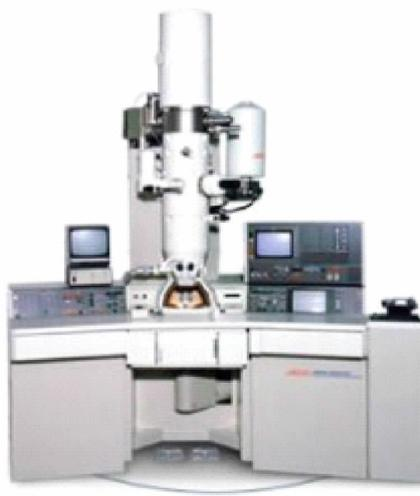
Fig. 3-12 TEM equipment (JEOL-2000 FX)
