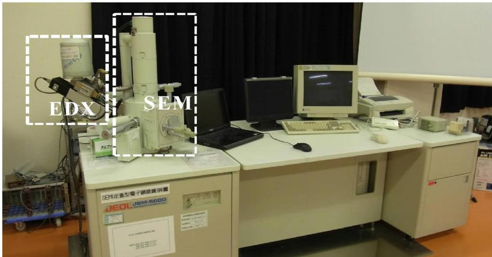
Fig. 3-11 SEM (JSM-5600) with an EDX
