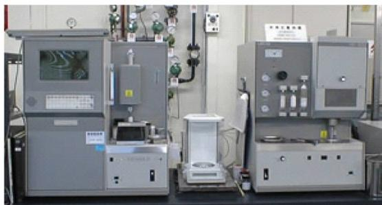
Fig. 3-1 Carbon/Sulfur analyzer (LECO CS-444LS)
