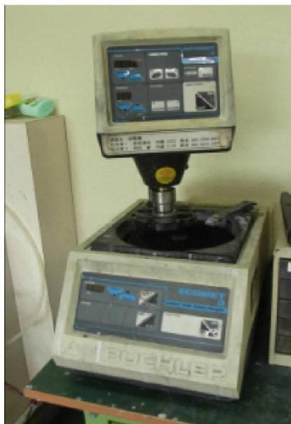
Fig. 3-4 Grinding machine
