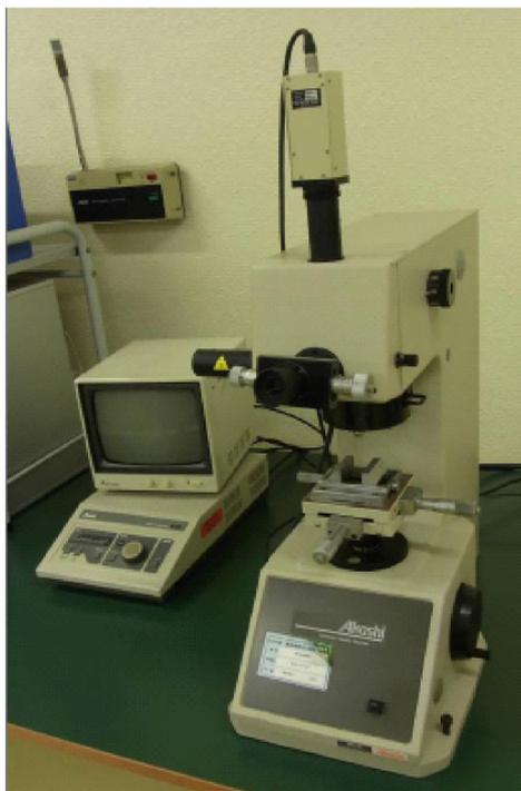
Fig. 3-5 Micro-hardness tester (in Vickers' hardness)
