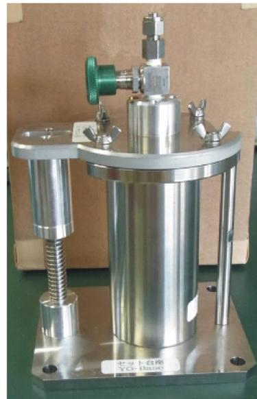
Fig. 6-6 Vacuum container for transporting packed capsules
