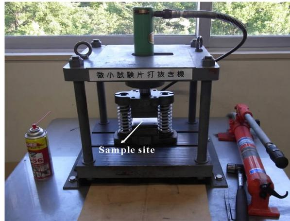
Fig. 3-8 Punch mold for tensile/creep samples
