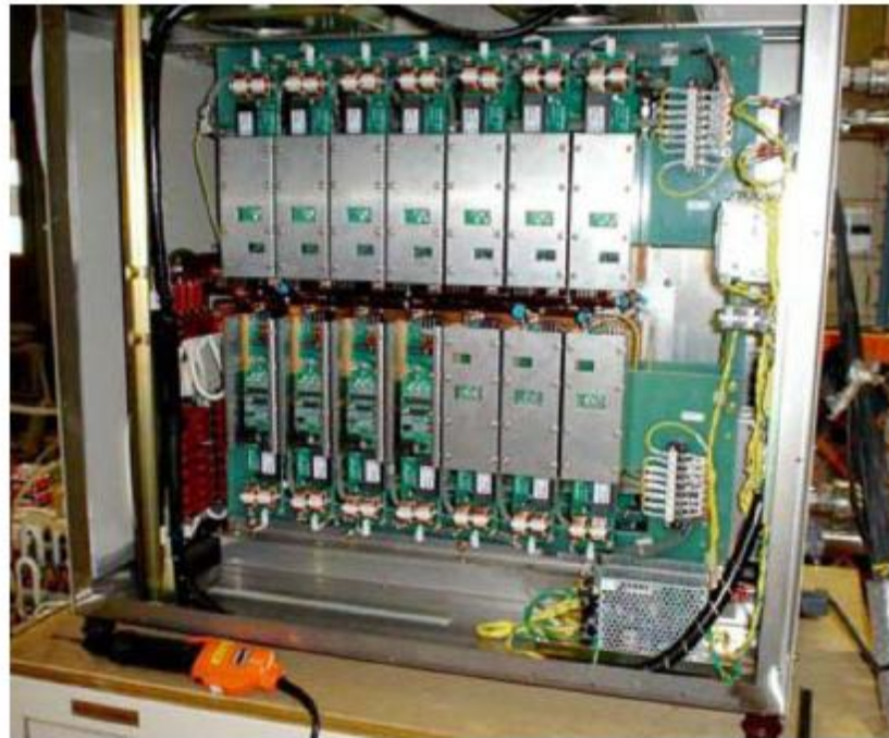
Fig. 2.2.4.2a: A photo of the SPS with seven MOSFETS in a single arm
