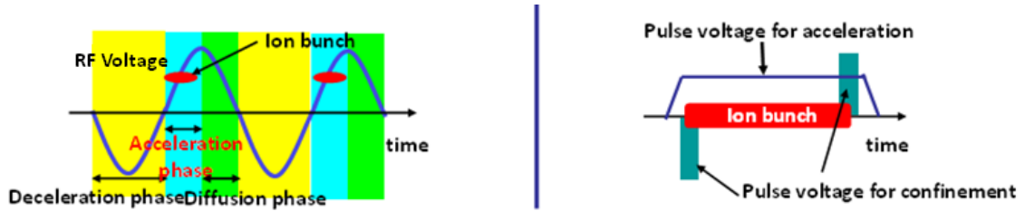
Figure 2.1c: Voltage profile in the conventional RF synchrotron and induction synchrotron
