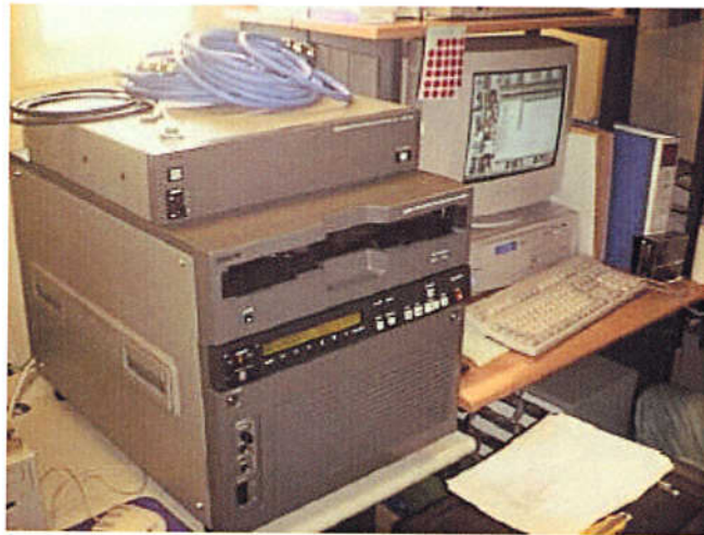
Figure 3.14 The VLBI back-end system in the satellite data reception room. Upper: The K4 terminal, TCU and delay-calibrator. Lower: The recorder, computer for the field system to control the recorder and the SCSI interface to VLBI raw data.
