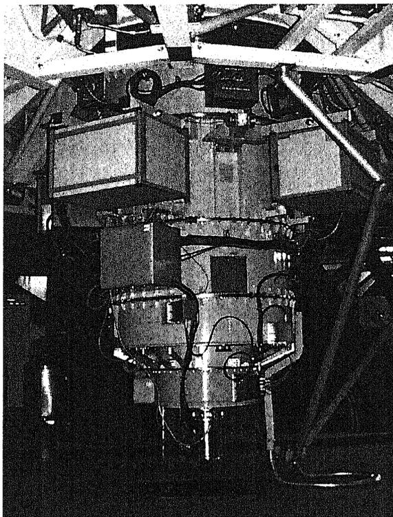
Figure 2.10: CCD array of FORS (FOcal Reducer and low dispersion Spectrograph). This instrument supports 2 image scales depending on the collimator used. The high resolution mode has a pixel scale of  $0.''1$  on the  $24 \mu\text{m}$  of  $2048 \times 2048$  pixels CCD array.
