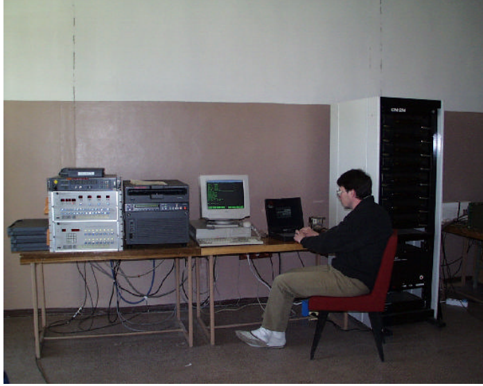
Figure 2.3: The K4 data acquisition system (Type-1) used for Japan-Russia pulsar VLBI observation. The K4 video converter, K4 local oscillator, and data input interface (DFC-1100) are seen on the left side of the desk. The K4 recorder (DIR-1000L) and the control computer are in the middle of the desk. The S2 type VLBI recording terminal (S2-RT) is seen on the right-most side of the picture.
