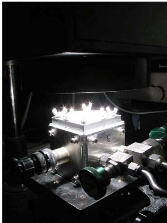
Fig. 2.9 Irradiation of simulated solar light to the cell.
