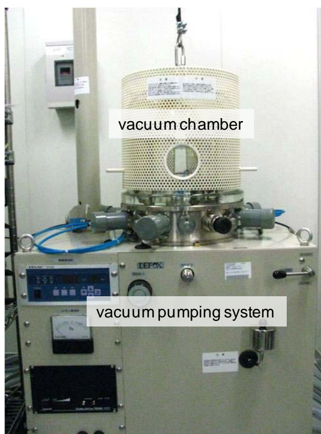
Fig. 2.4 Vacuum evaporator.
