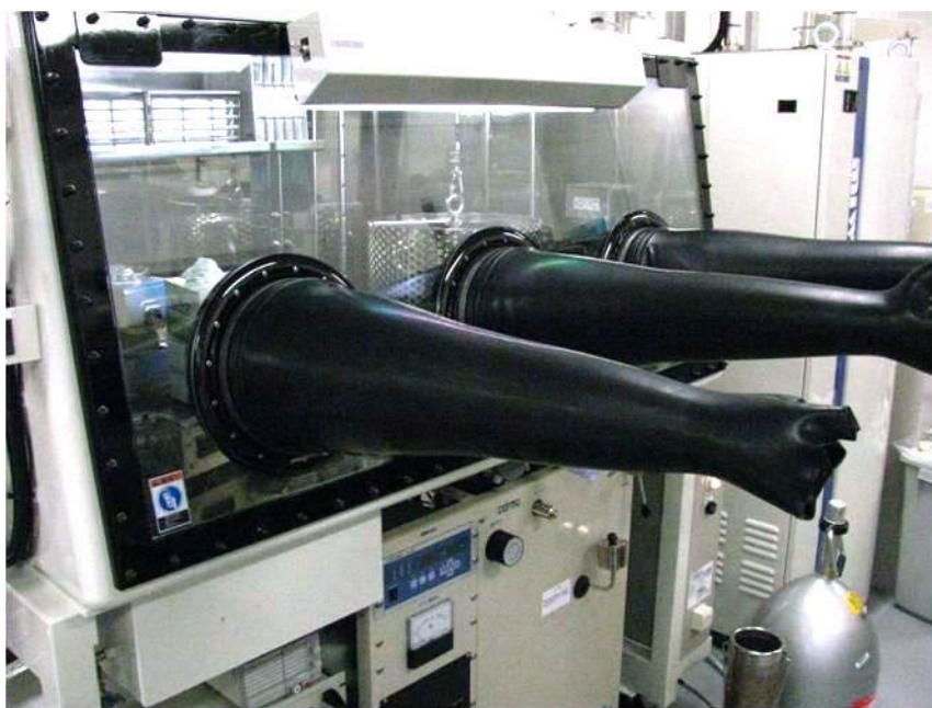
Fig. 2.12 Glove box with a built-in vacuum evaporator.
