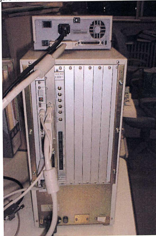
Figure 4.3: The backside of the dedicated VLBI terminal 'SRTP Station'
