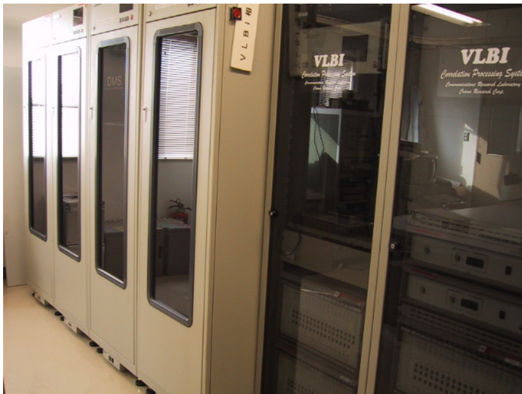
Figure 3.1 Tape-based KSP correlator system.
