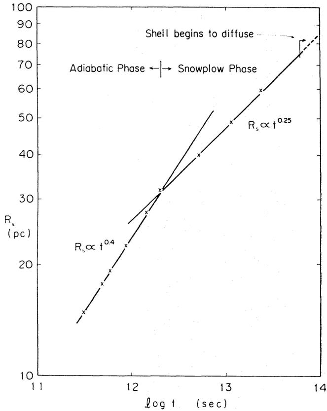
Fig. 1. Time variation of the radius of shock front in the case of a point explosion in a uniform medium.
