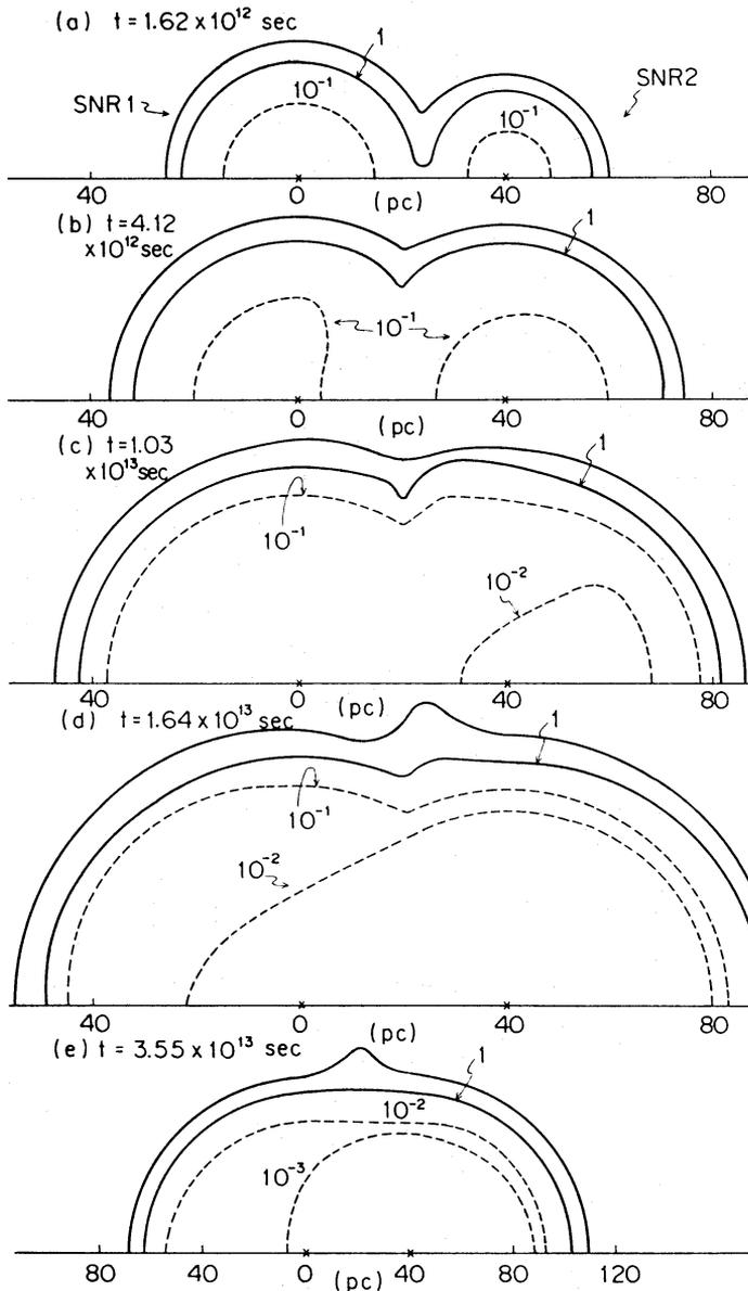
Fig. 3. Density profiles of interacting SNRs at the typical five stages in the case of Model I. The outermost solid line shows the most dense shell and the inner solid line is for  $n=1$  atom  $\text{cm}^{-3}$ . Then, the region surrounded by these two solid lines is the compressed shell by the shock wave. Two crosses show the explosion points. Contours are labeled with the value of number density in atoms  $\text{cm}^{-3}$ .
