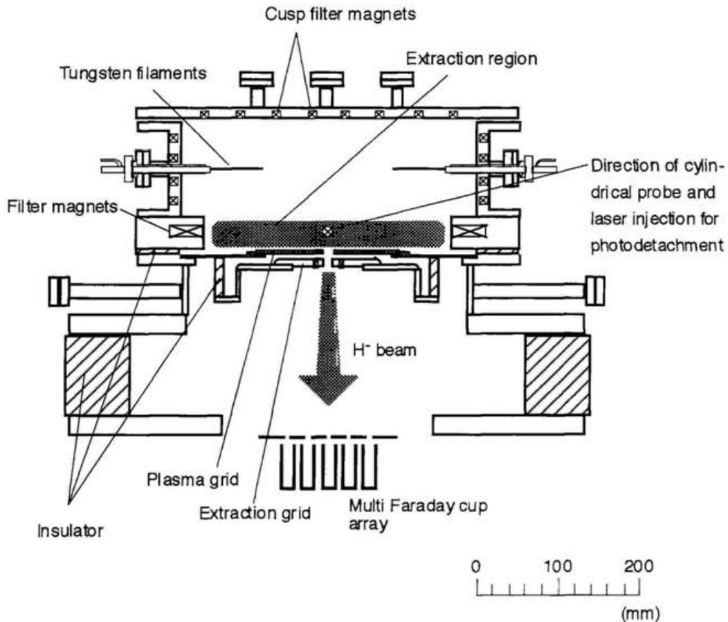
Fig. 3-1. A schematic diagram of the ion source.
