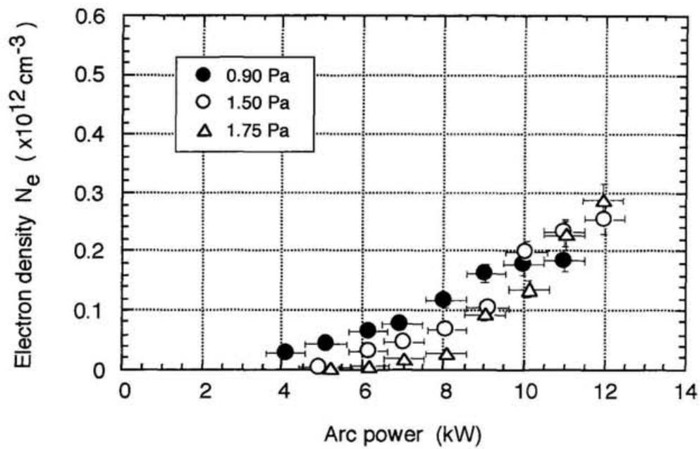
Fig. 4-14. The discharge arc power dependence of the electron density in the extraction region at configuration B.
