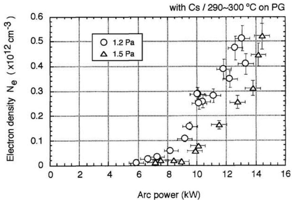
Fig. 4-19. The discharge arc power dependence of the electron density in the extraction region with injection of the cesium vapor into the arc chamber.
