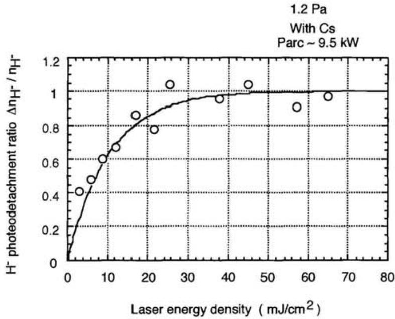
Fig. 3-6. Laser power dependence of the photodetachment ratio to the original  $H^-$  ions (here, the electron density and the  $H^-$  density in the extraction region are  $3.9 \times 10^{11} \text{ cm}^{-3}$  and  $3.0 \times 10^{11} \text{ cm}^{-3}$ , respectively).
