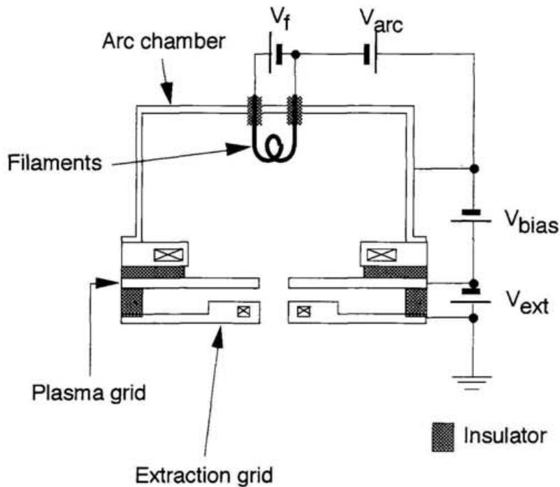
Fig. 3-11. A schematic diagram of the power supply for the ion source.
