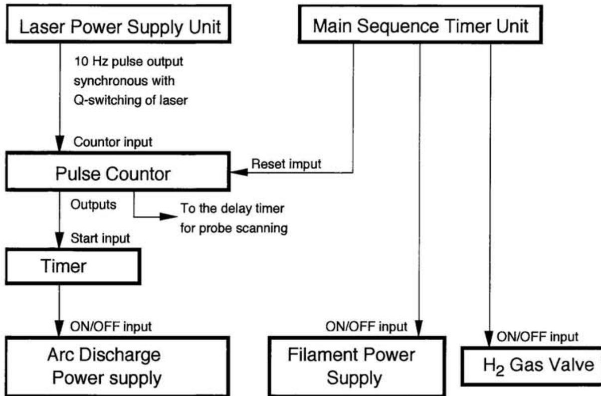
Fig. 3-12. A diagram of timing connection of the operation systems of the ion source.
