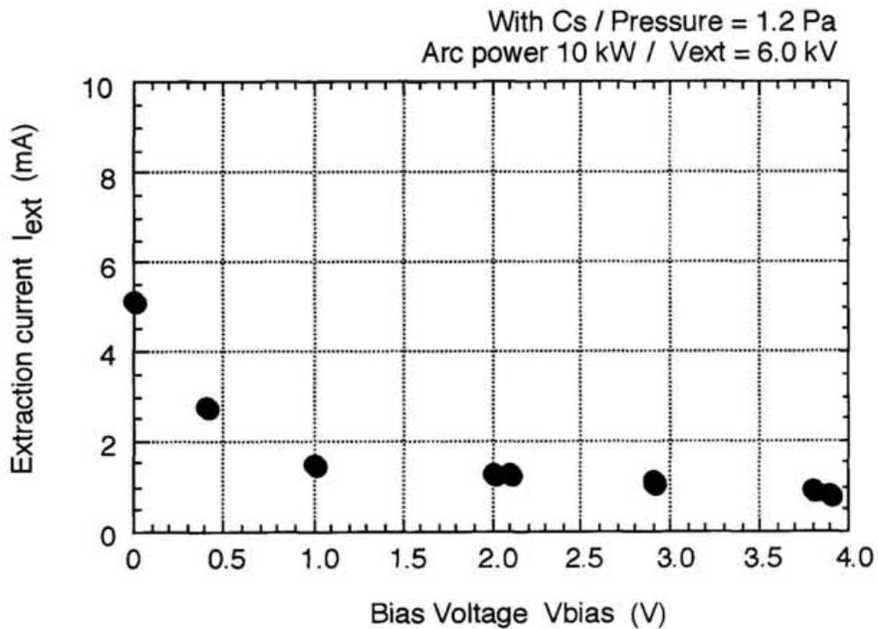
Fig.4-22. The bias voltage dependence of the extracted electron current from the ion source with injection of the cesium vapor into the arc chamber.
