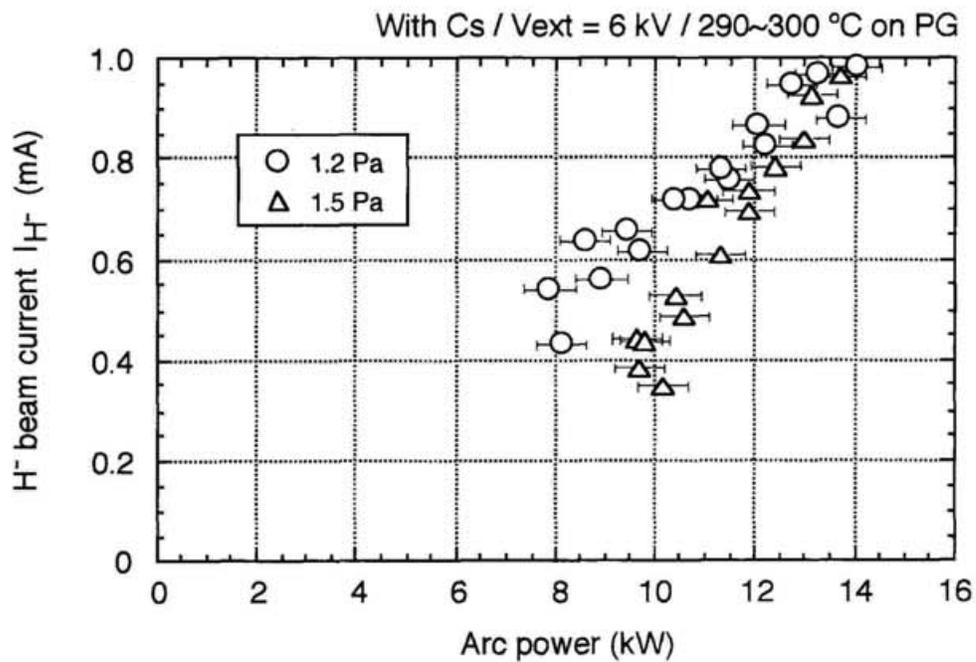
Fig. 4-16. The discharge arc power dependence of the H<sup>-</sup> beam current extracted from the ion source with injection of the cesium vapor into the arc chamber.
