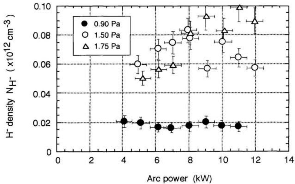
Fig. 4-13. The discharge arc power dependence of the  $\text{H}^-$  density in the extraction region at configuration B.
