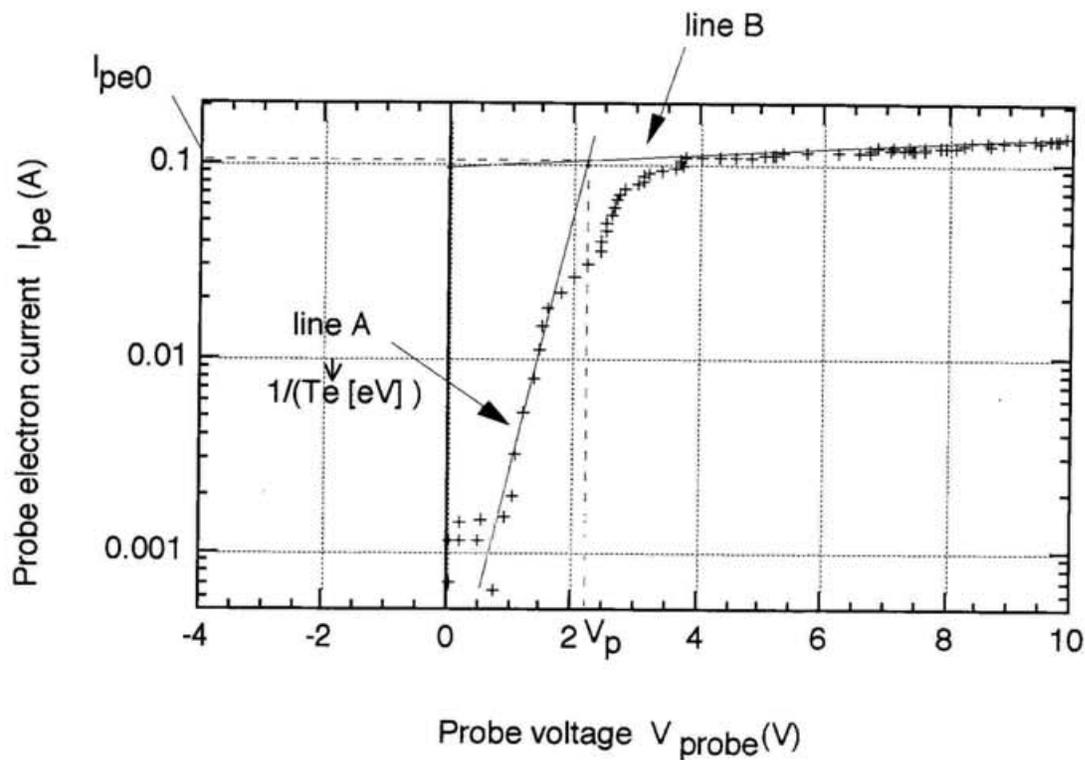
Fig. 3-8. An example of probe trace in the extraction region (in operating with cesium, pressure 1.2 Pa, arc power 12.4 kW).
