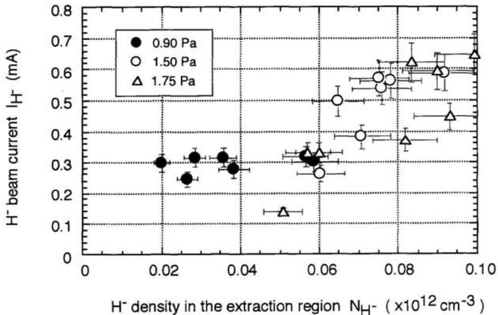
Fig. 5-1. The relation between the  $H^-$  density in the extraction region and the extracted  $H^-$  beam current at the operation without cesium.
