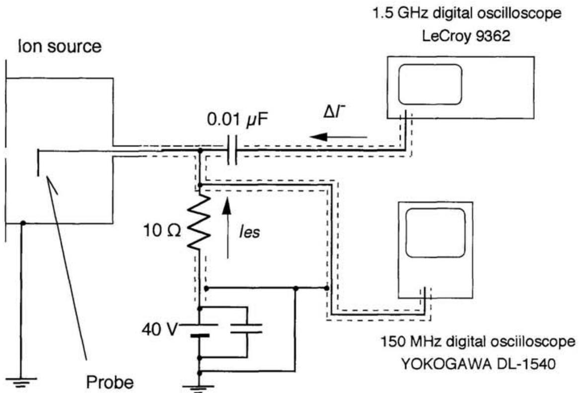
Fig. 3-4. A schematic diagram of the circuit for the photodetachment measurement.
