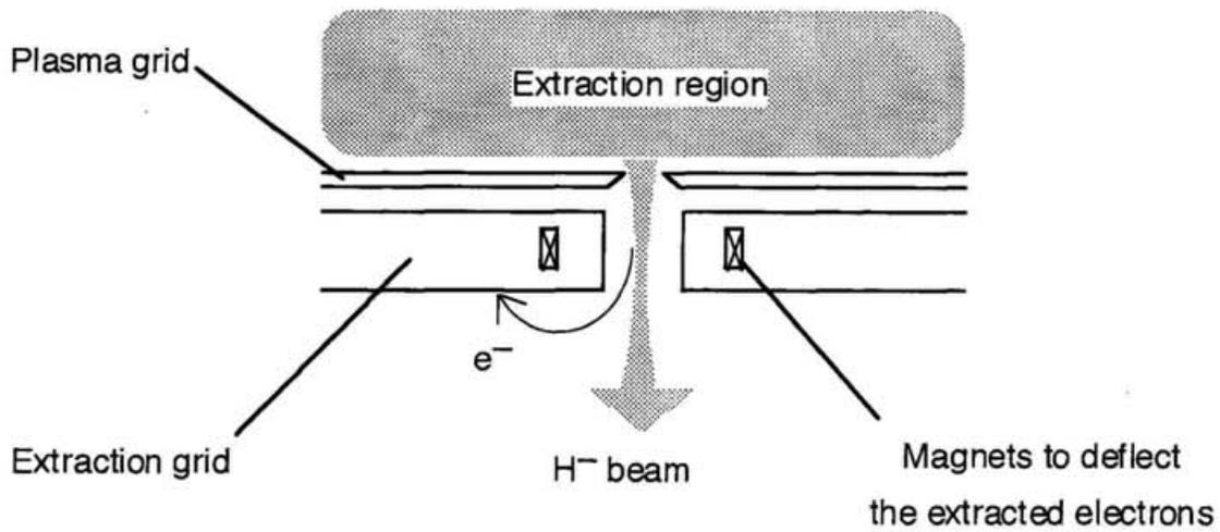
Fig. 3-2. A schematic diagram of the extractor.
