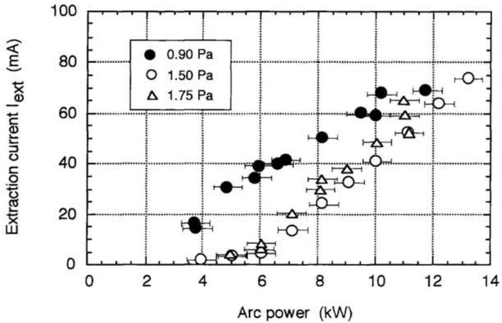
Fig. 4-5. The discharge arc power dependence of the extracted electron current from the ion source at configuration A.
