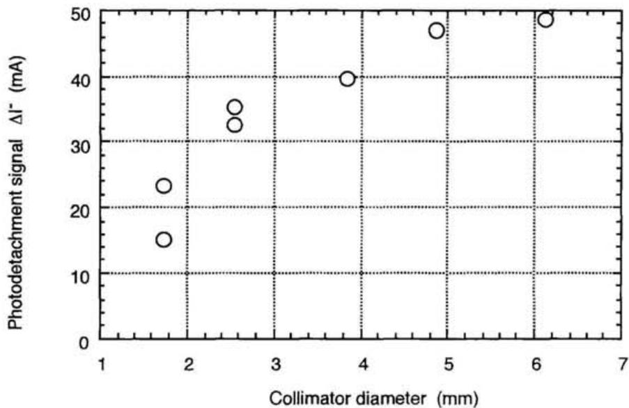
Fig. 3-7. Laser diameter dependence of the photodetachment signal under the constant laser power density (in operating without cesium, pressure 1.5 Pa, arc power 5 kW).
