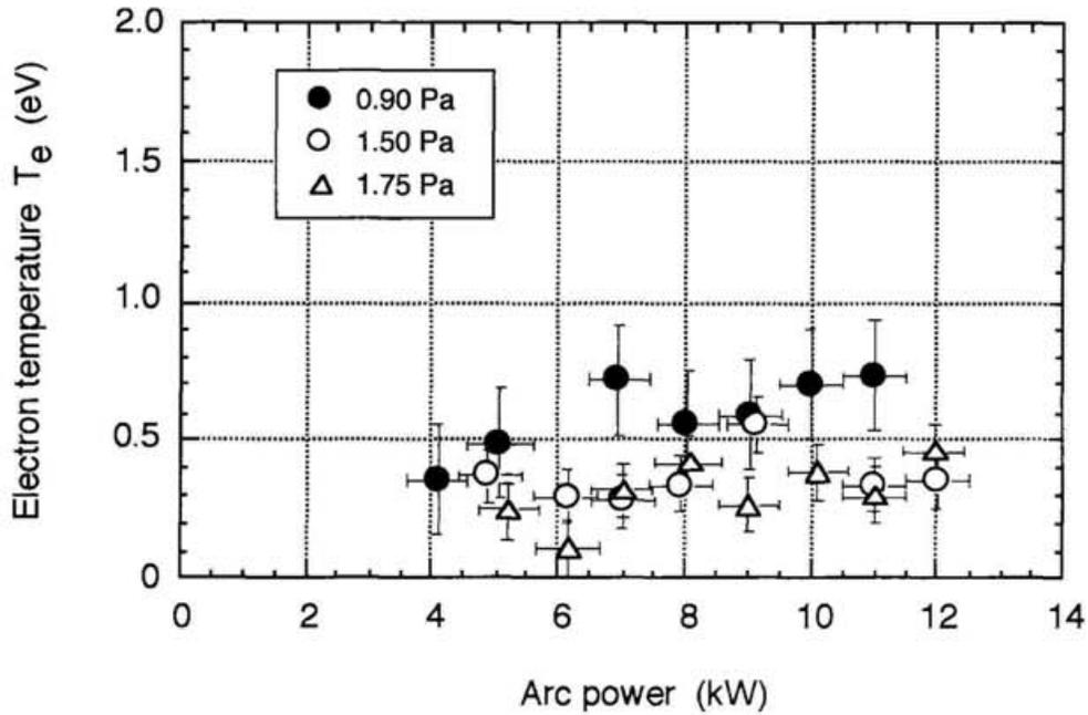
Fig.4-15. The discharge arc power dependence of the electron temperature in the extraction region at configuration B.
