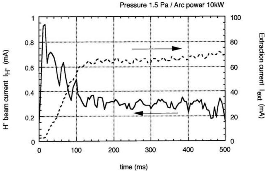
Fig. 4-2. The time evolution of the H<sup>-</sup> beam current (solid line) and the electron current (dotted line) extracted from the ion source at configuration A in operating without cesium.
