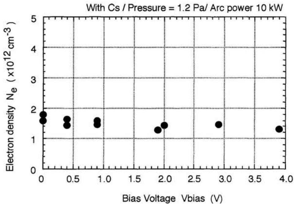
Fig. 4-24. The bias voltage dependence of the electron density in the extraction region with injection of the cesium vapor into the arc chamber.
