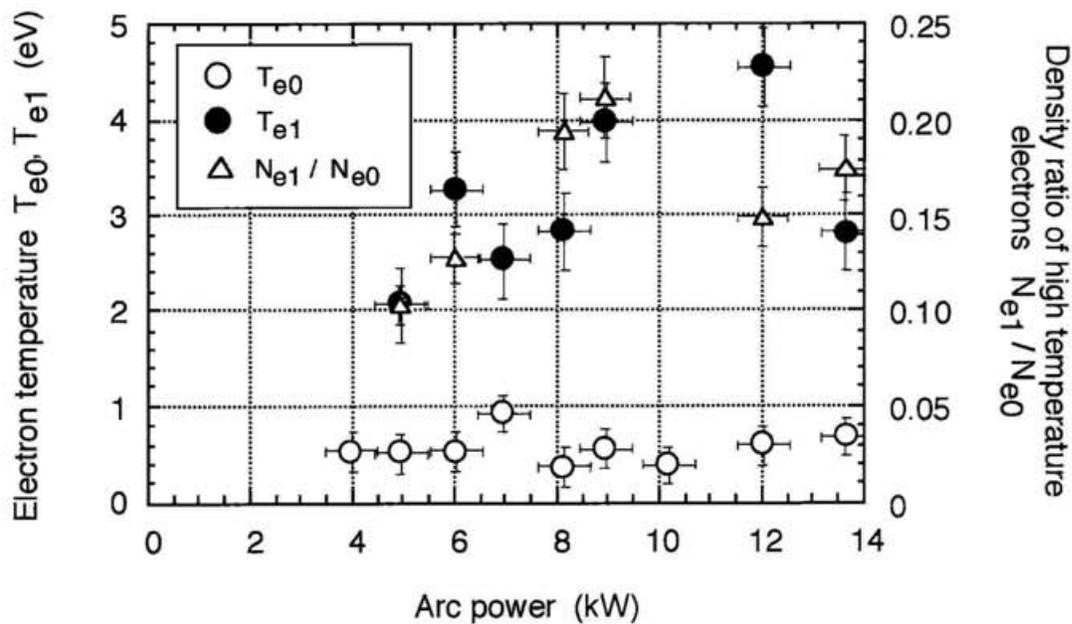
Fig. 4-10. The discharge arc power dependence of the electron temperature  $T_{e0}$  (main component),  $T_{e1}$  (high temperature component) and the density ratio of the high energy tail to the main electrons in the extraction region at configuration A at gas pressure; 1.2 Pa.
