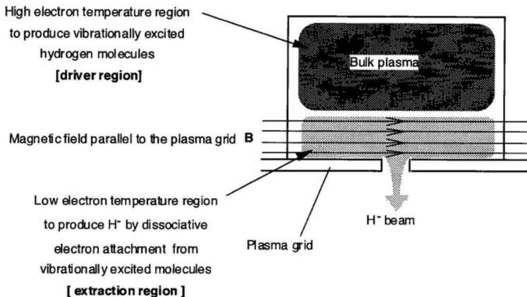
Fig. 1-1 An illustration of the tandem source.
