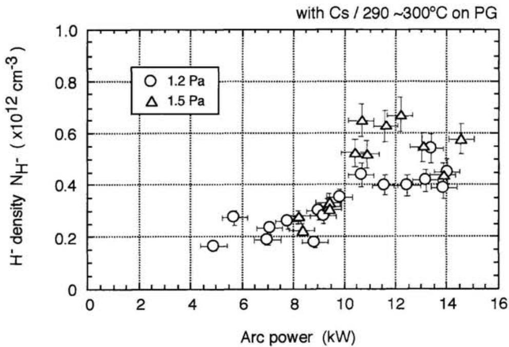
Fig. 4-18. The discharge arc power dependence of the H<sup>-</sup> density in the extraction region with injection of the cesium vapor into the arc chamber.
