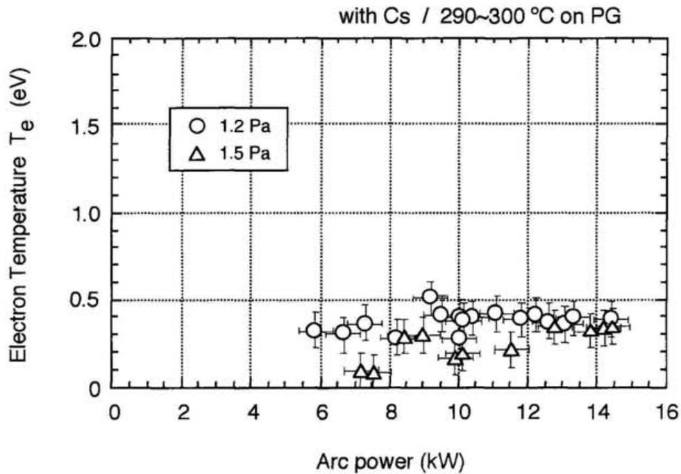
Fig.4-20. The discharge arc power dependence of the electron temperature in the extraction region with injection of the cesium vapor into the arc chamber.
