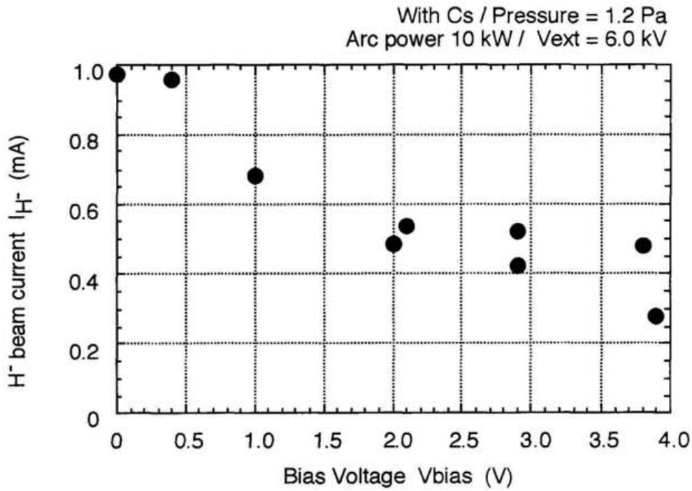
Fig. 4-21. The bias voltage dependence of the  $H^-$  beam current extracted from the ion source with injection of the cesium vapor into the arc chamber.
