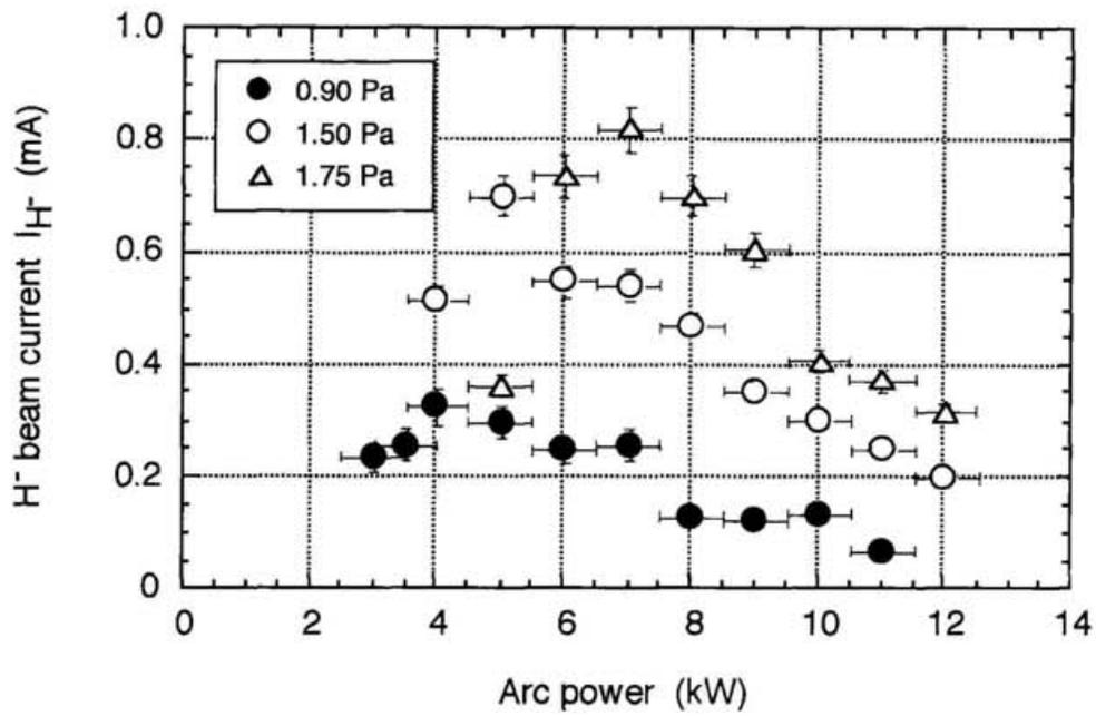
Fig. 4-4. The discharge arc power dependence of the H<sup>-</sup> beam current extracted from the ion source at configuration A.
