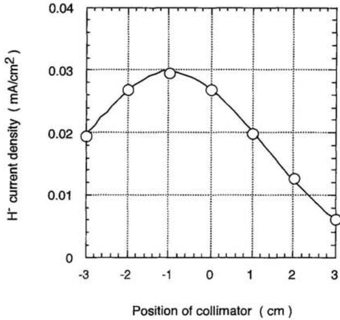
Fig. 3-10. An example of the Faraday cup signal on the horizontal direction. Here, a total H<sup>-</sup> current is measured as 0.98 mA at the condition of 1.2 Pa, 10 kW of the arc power, 6.0 kV of the extraction voltage, and operating with cesium.
