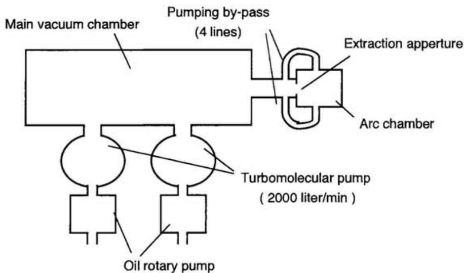
Fig. 3-14. A schematic diagram of the gas pumping system.
