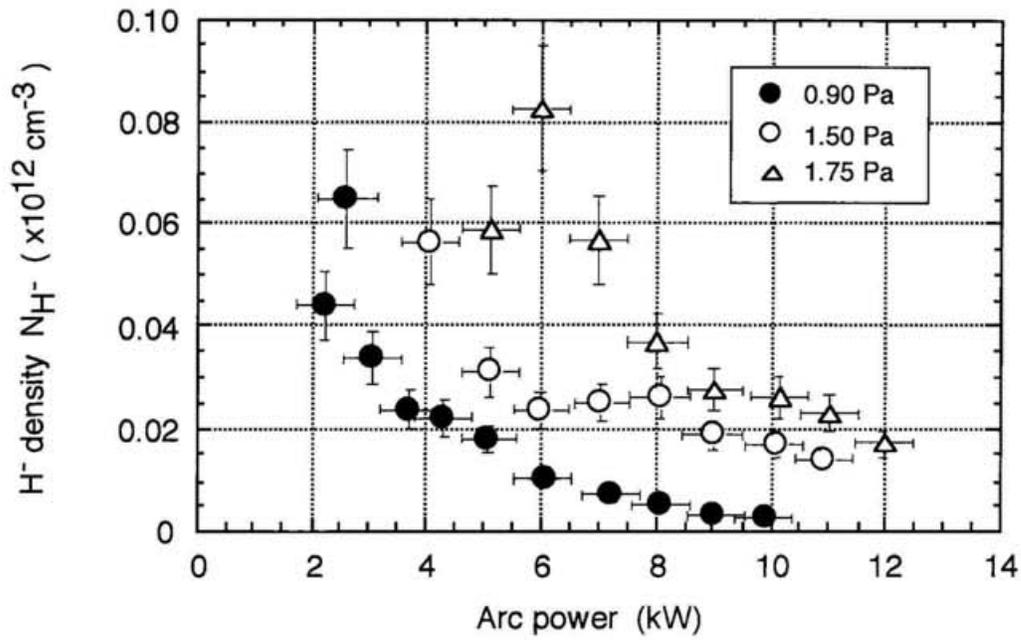
Fig. 4-6. The discharge arc power dependence of the  $H^-$  density in the extraction region at configuration A.
