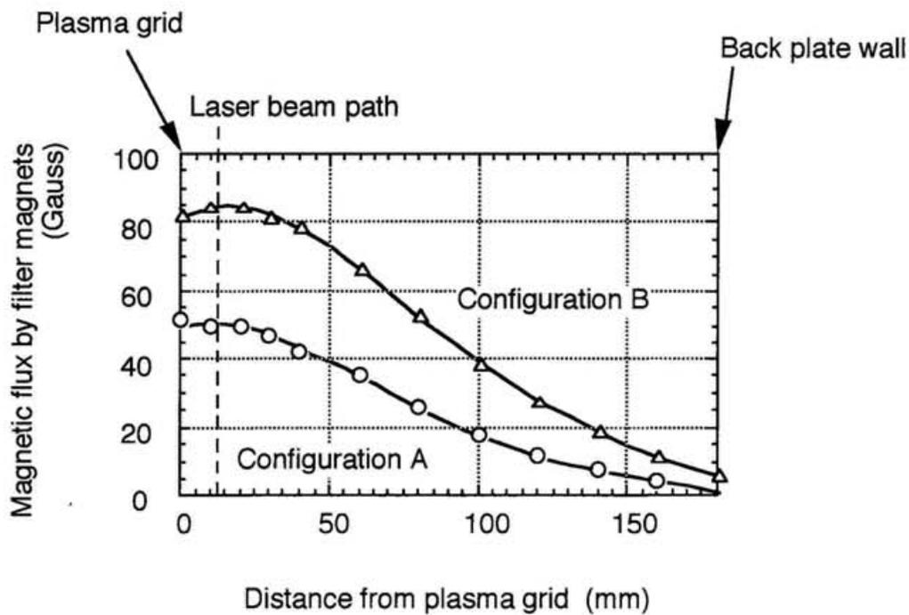
Fig. 4-3. Measured filter magnetic field distribution on the center axis of the ion source. (circle; configuration A: weak magnetic field of  $750 \text{ G} \cdot \text{cm}$ , triangle; configuration B: strong magnetic field of  $1600 \text{ G} \cdot \text{cm}$ )
