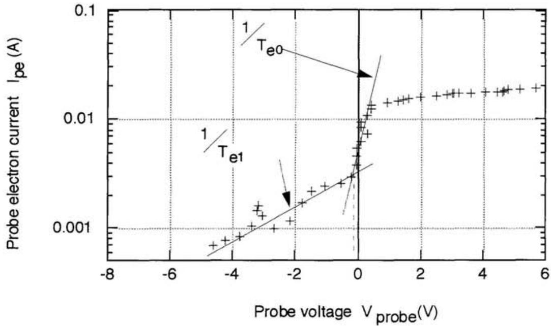
Fig. 4-9. An example of the probe trace at configuration A. It can be seen that there are two components in electron temperature.
