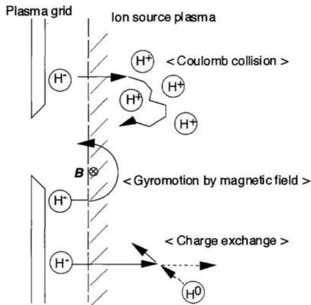
Fig. 5-3. An illustration of the models of the reflection of surface-produced  $H^-$  into an aperture on a plasma grid.
