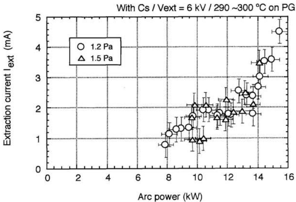
Fig. 4-17. The discharge arc power dependence of the extracted electron current from the ion source with injection of the cesium vapor into the arc chamber.
