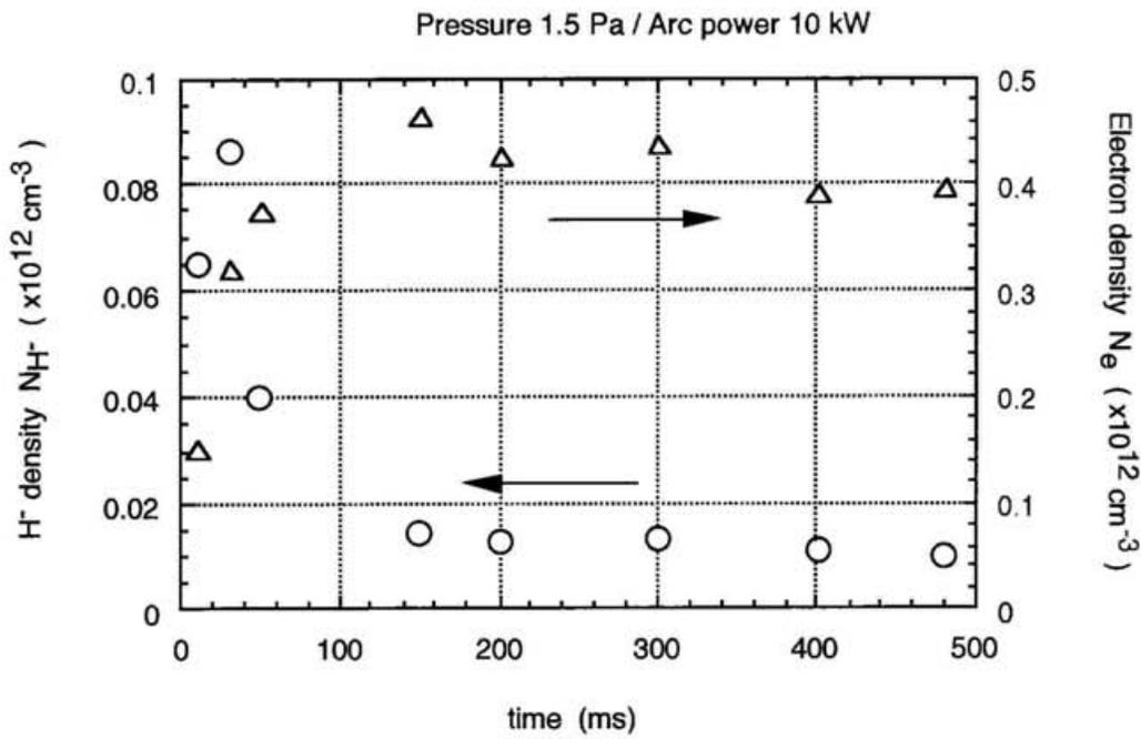
Fig. 4-1. The time evolution of the H<sup>-</sup> density (open circle) and the electron density (triangle) in the extraction region at configuration A in operating without cesium.
