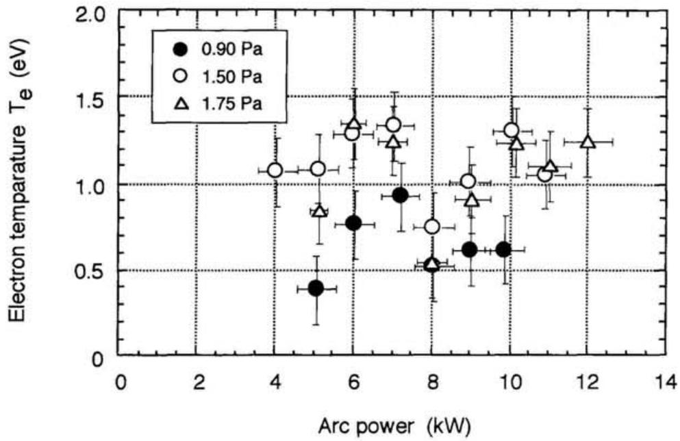
Fig. 4-8. The discharge arc power dependence of the electron temperature in the extraction region at configuration A.
