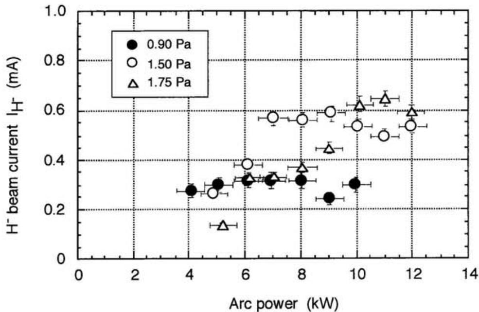
Fig. 4-11. The discharge arc power dependence of the  $H^-$  beam current extracted from the ion source at configuration B.
