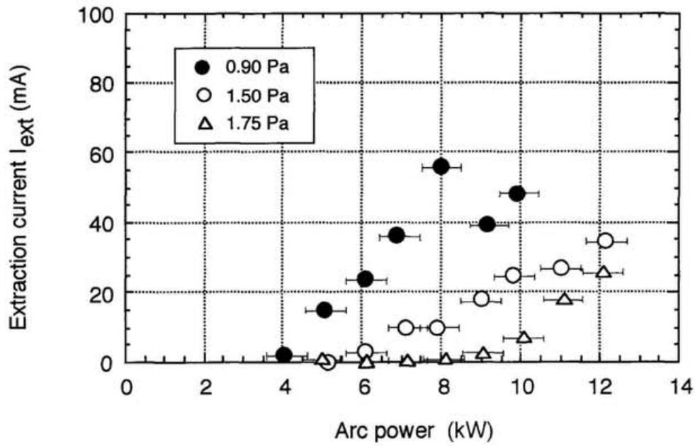
Fig. 4-12. The discharge arc power dependence of the extracted electron current from the ion source at configuration B.
