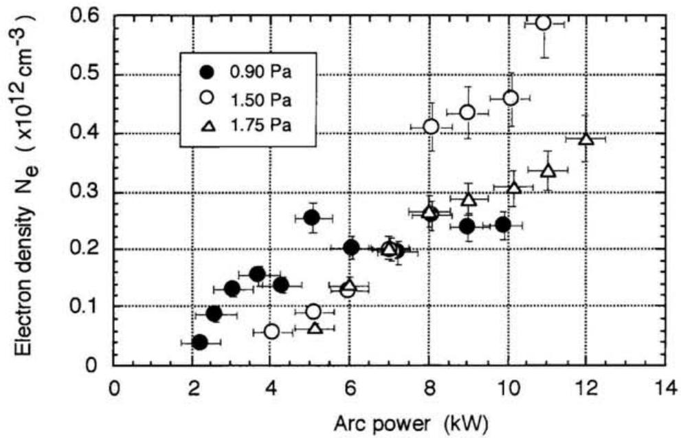
Fig. 4-7. The discharge arc power dependence of the electron density in the extraction region at configuration A.
