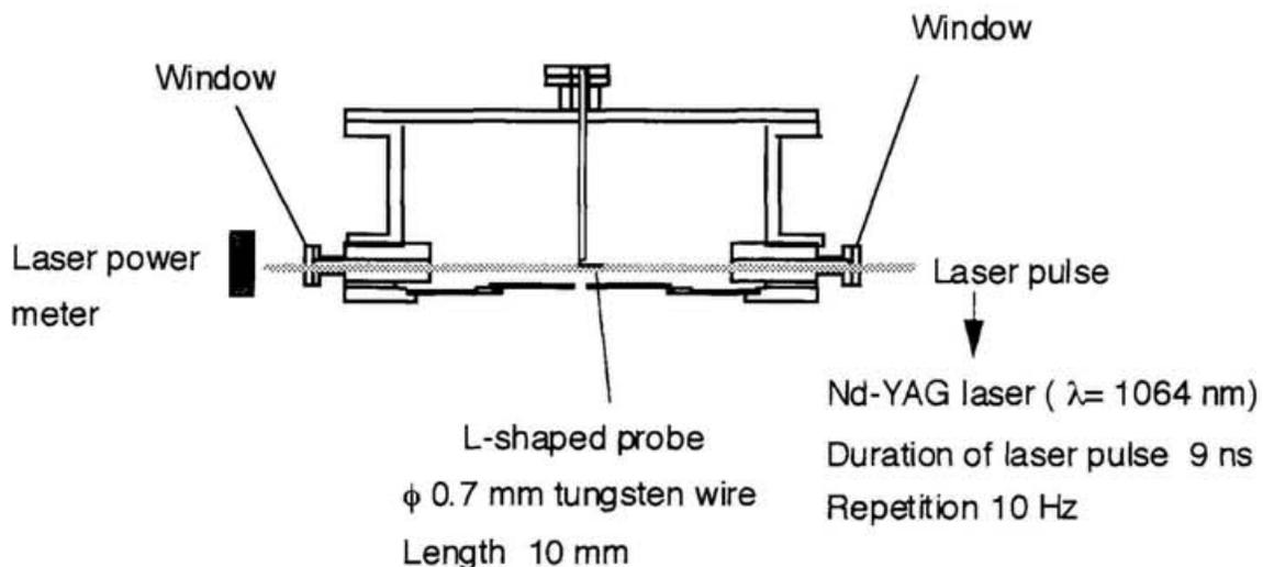
Fig. 3-3. A schematic diagram of the laser photodetachment measurement system.
