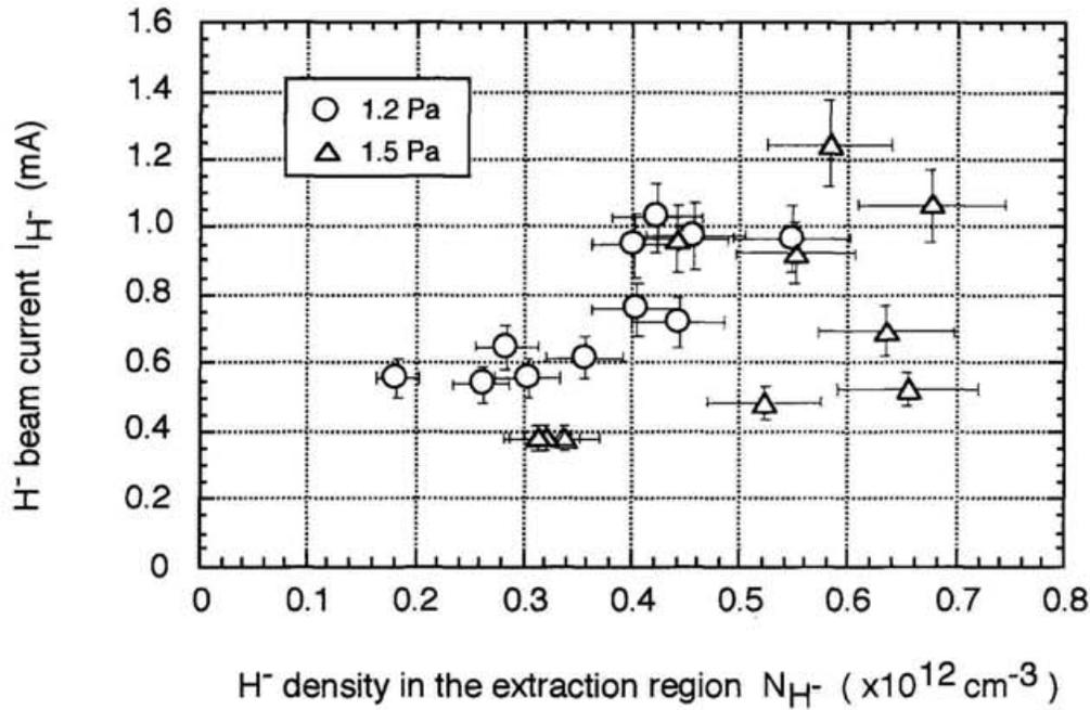
Fig. 5-2. The relation between the  $H^-$  density in the extraction region and the extracted  $H^-$  beam current at the operation with cesium.
