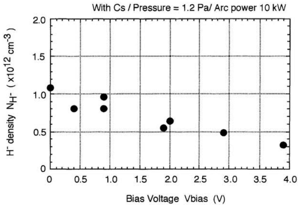
Fig. 4-23. The bias voltage dependence of the  $H^-$  density in the extraction region with injection of the cesium vapor into the arc chamber.
