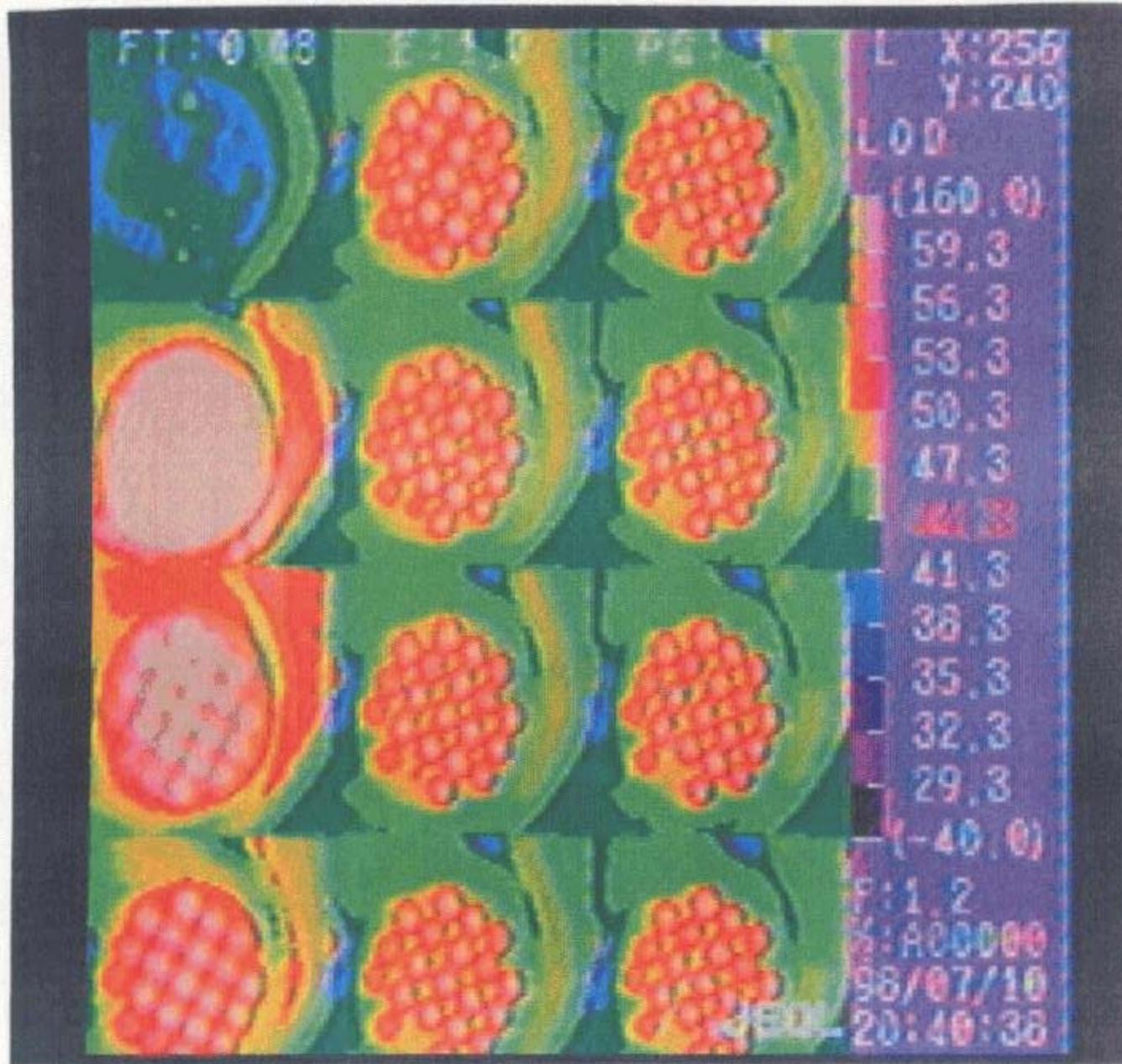
Fig.3.12 Temperature profile of carbon plate
