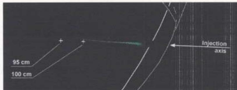
Fig. 47. CCD image of a reference pellet without a core (Shot #74652,  $R_{ax} = 92.1$  cm): Li II filter, side view from CCD3.
