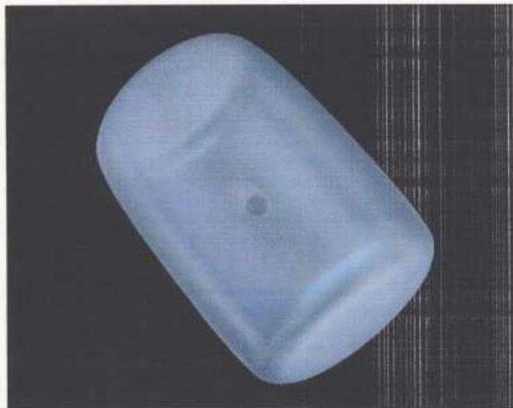
Fig. 28. One example of the 3D reconstructed virtual picture of the tracer-encapsulated cryogenic pellet.
