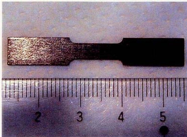
Fig. 4.2-5 \text{Al}_2\text{O}_3 long fiber/BPSCCO test piece for tensile test.
