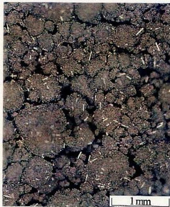
Fig. 3.2-6 Photograph of \text{Al}_2\text{O}_3 /short fiber/BPSCCO mixed powder by optical microscope.
