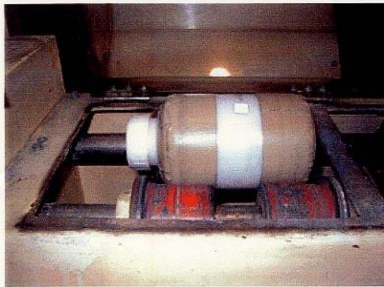
Fig. 3.2-4 Photograph of ball mill for short fibers and BPSCCO calcined powder.
