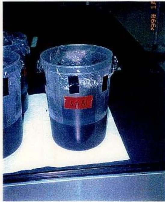
Fig. 3.2-5 Photograph of short fiber/BPSCCO/ethanol mixed slurry.
