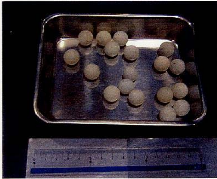
Fig. 3.2-3 Photograph of balls for ball mill.
