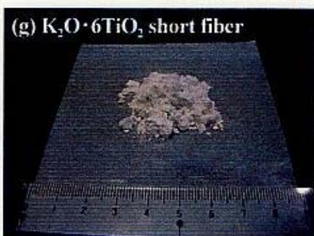
Fig. 3.2-1 Photographs of the fibers for addition to BPSCCO.
