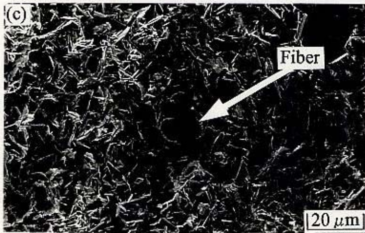
Fig. 3.4.1-1 Structure of no-fiber BPSCCO sample and short fiber/BPSCCO samples sintering at 1113 K for 90ks; (a) no-fiber BPSCCO, (b) \text{Al}_2\text{O}_3/\text{BPSCCO} , (c) \text{ZrO}_2 \cdot \text{Y}_2\text{O}_3/\text{BPSCCO} .
