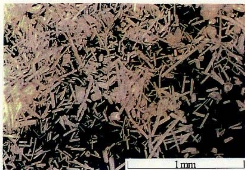
Fig. 3.4.1-6 Photograph of ZrO_2 \cdot Y_2O_3 fibers by optical microscopy.
