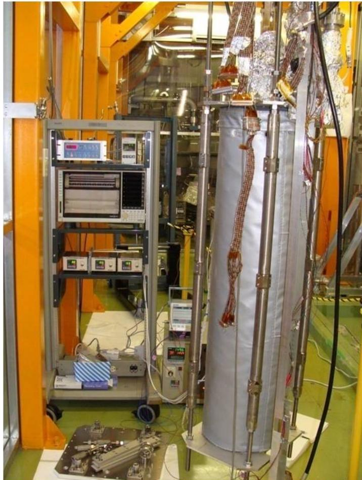
Figure 2. 35 Cavity during baking with heating jacket.
