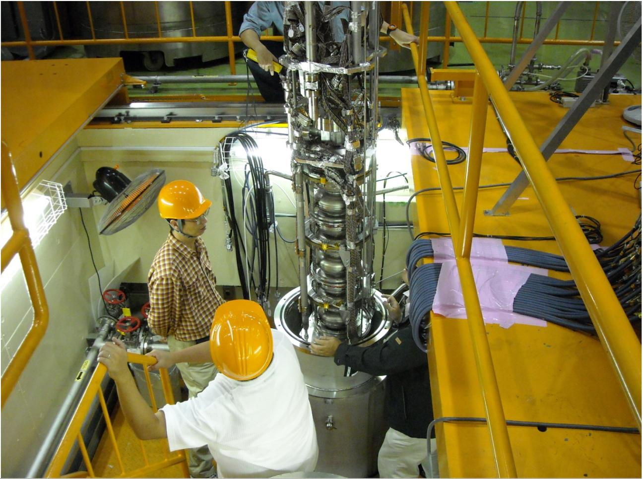
Figure 4.2 Cryostat pit for vertical test in STF.
