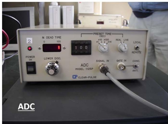
Figure 4.9 NaI scintillator setup, photomultiplier (top left), high voltage generator (top right) and analog-digital converter (bottom right).
