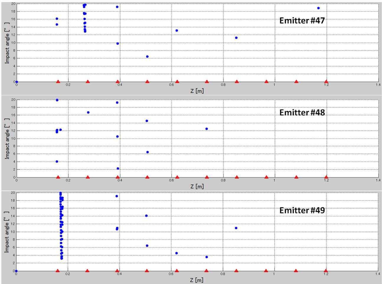
Figure 5. 72 Incident angle along  $360^\circ$  meridian for  $8/9 \pi$  mode at 23.5MV/m for emitters 47, 48 and 49.
