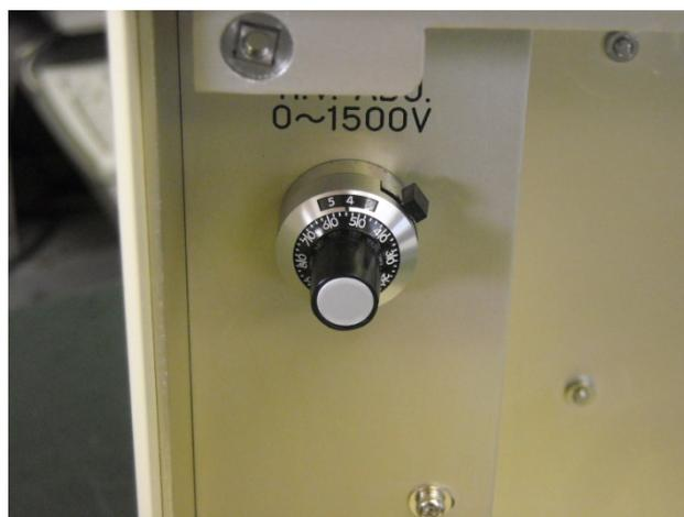
Figure 4.10 Voltage adjustment knob.
