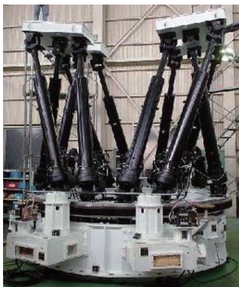
Figure 2.3: Stewart-mount dual-beam platform of the VERA antennas. ©VERA Project/National Astronomical Observatory Japan
