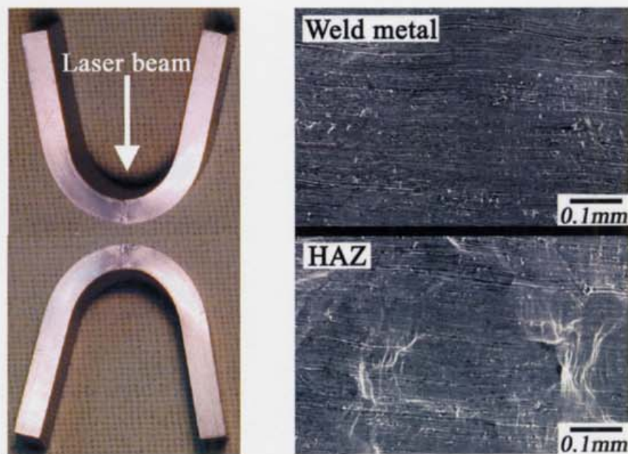
Fig. 3-16 Outwards and the surface of the weld zone after the bend test in the low input power.
