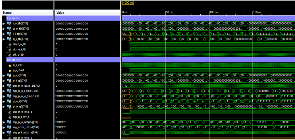
Figure 8.3: iSim simulation of the LUT-based klystron linearization algorithm.
