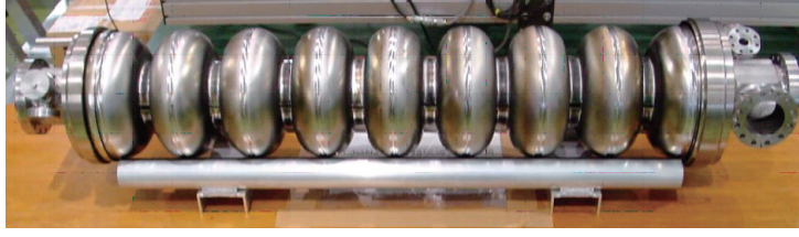
Figure 2.2: Picture of a 9-cell TESLA-like cavity [7].
