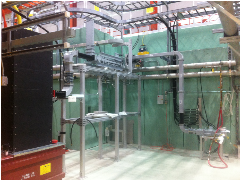
Figure 8.14: Photo of setup of klystron linearization measurement. On the left side the klystron is located, in the middle the circulator, and on the right side the water load.
