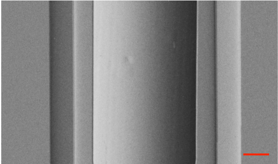
Fig. 3.11. Differential image of acrylic case using MDEI at 17.5 keV. Bar = 1 mm.
