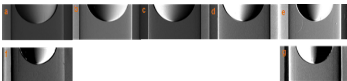
Fig. 4.8. DEI projection images (a-e) and MDEI (7times) projection images (f, g) of refraction based phantom.
