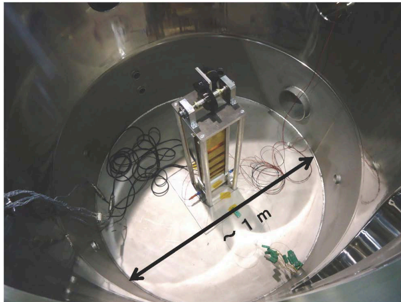
Figure 3.25: Experimental configuration for investigating compressional stress dependence of the thermal conductivity of powdered materials.
